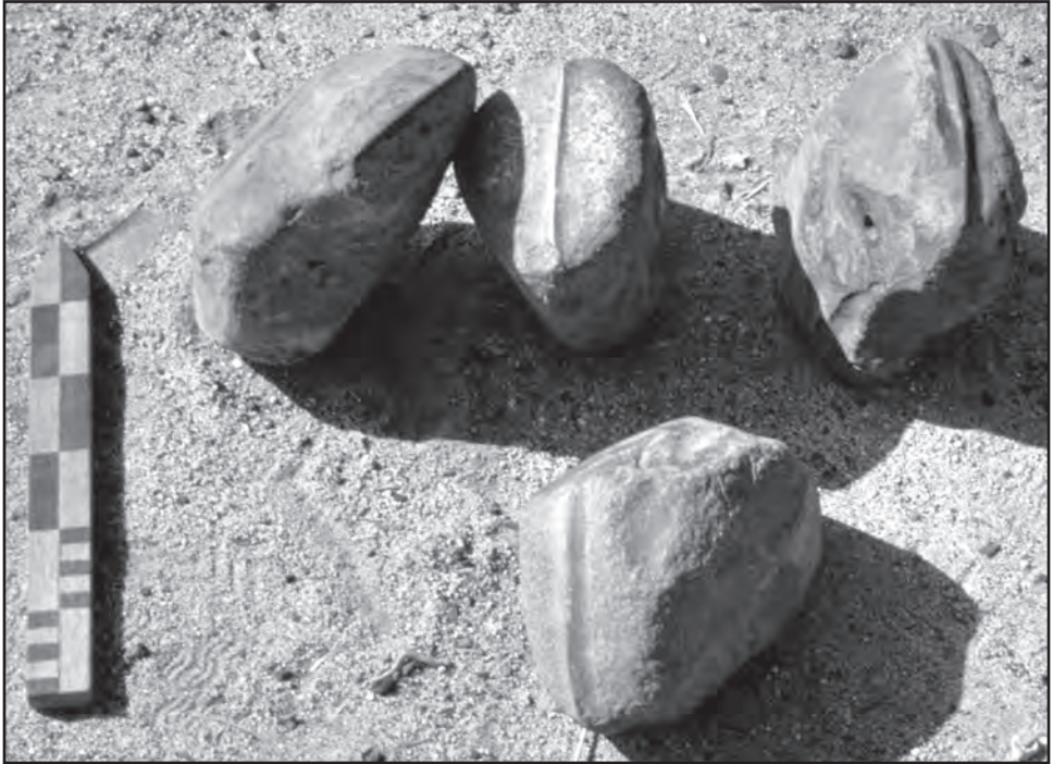
Figure 7.2. Ridged-boulder forging hammers. These particular tools are from the shop of a Mafa smith, but they are essentially the same as those used by the Plata.
