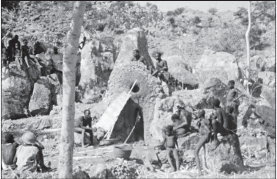
Figure 3.2. A moment early in the smelt by Truadak at Ldamszay in February 1953. Behind the furnace shield, a smith, his forehead smeared with red ocher, pumps pot bellows and is egged on by the songs of a smith playing the harp. Below and to the right Truadak and his brother, the latter wearing a hat of hyrax fur and holding a child, are seated on a rock. They are observing the color of the gases driven out of the vent at the base of the mud wall reinforced by bent withies that seals the furnace shaft. Shade provided by a mat improves their view of the gases. A sacrificed cock roasts on a stick leant against the furnace. Still from film by René Gardi (processing by Elias Kreyenbühl, Media Laboratory, Universität Basel).
