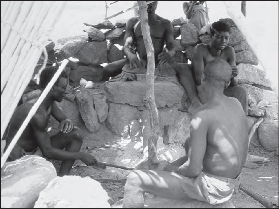
Figure 6.2. An Uldeme forge, showing the position of the bellows man. The striker is sitting on the anvil. Photo: Scott MacEachern.
