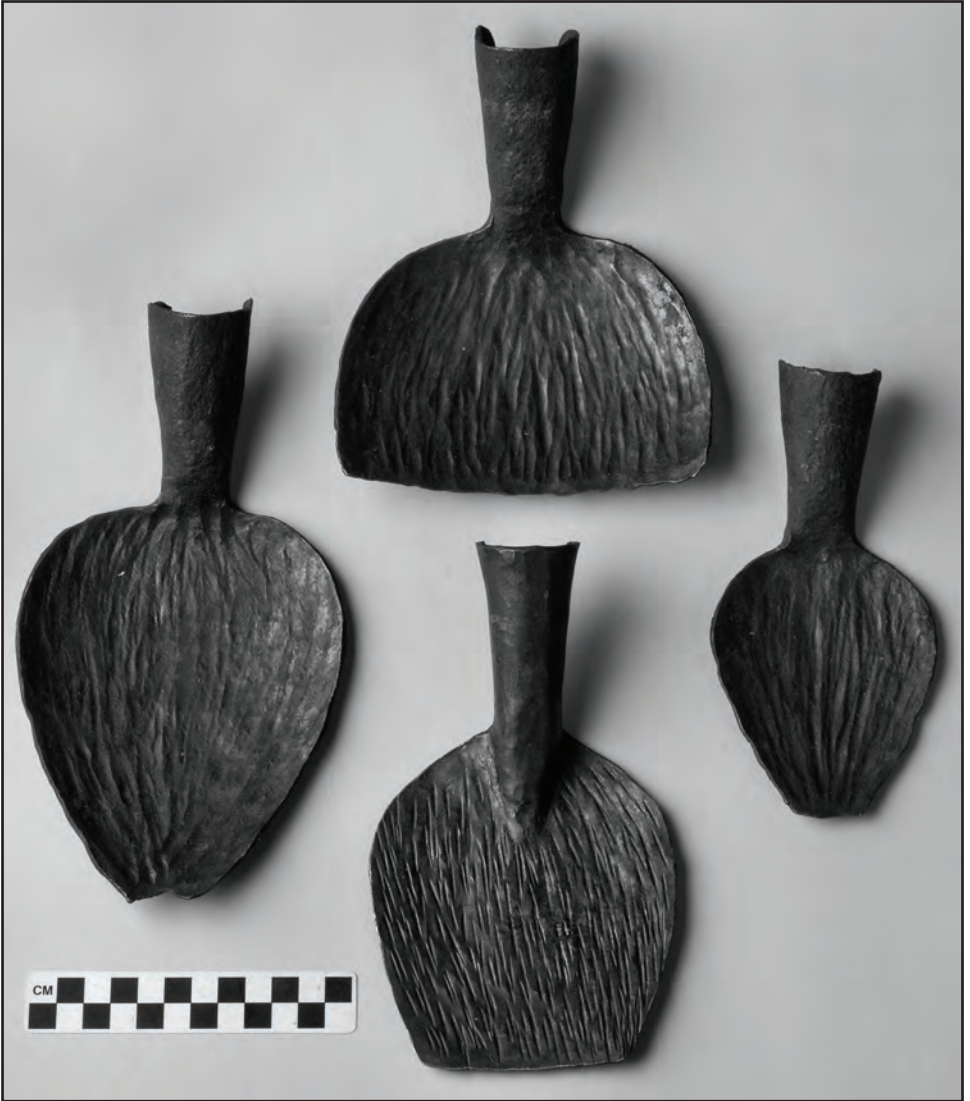
Figure 7.3. Hoes made by Plata smiths for Vamé (top), Mukhtelé (left) and Podokwo (right) farmers, each showing the wide, shallow striations left by the ridged-boulder hammers that are used to spread the blade area. The fourth hoe (bottom) was made by a Wandala smith at Manaouatchi, but intended for sale to montagnard farmers. Both the form and the narrow blade striations created by the use of a cross-peen hammer are intended to attract consumers who might otherwise buy a Plata-made hoe. Photo: Dave Brown, University of Calgary Imaging Services.
