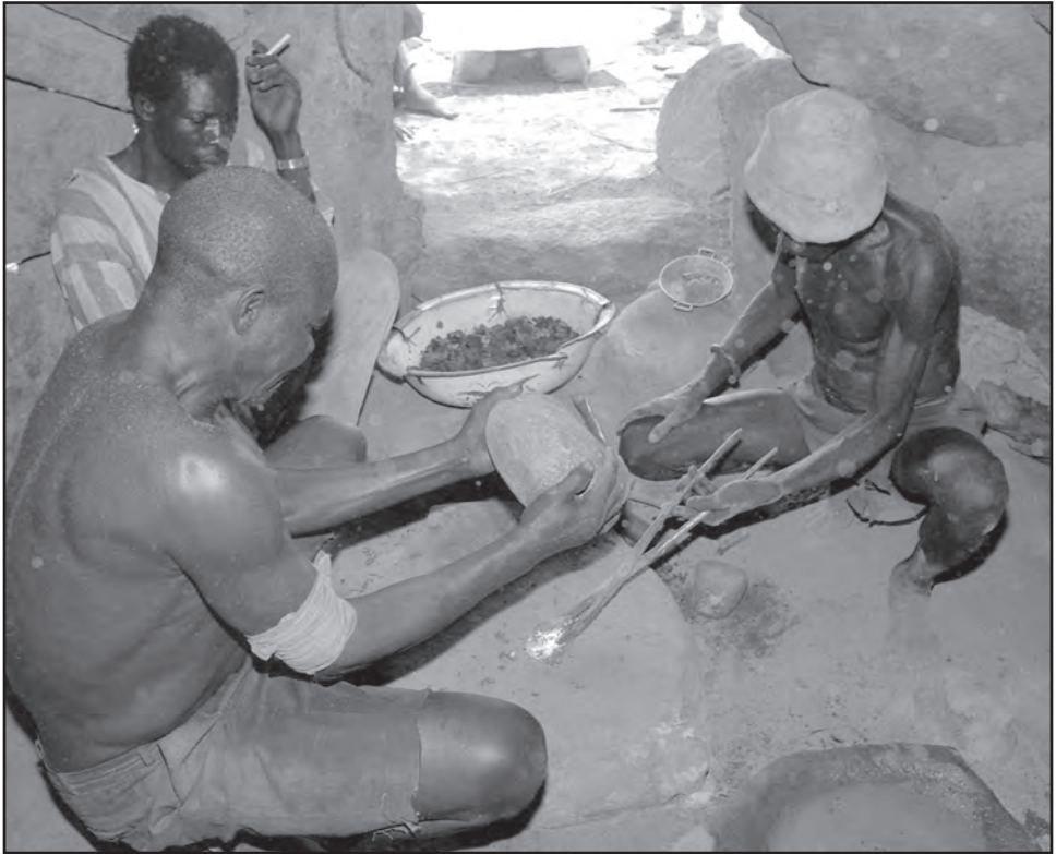
Figure 6.1. In their typical Mafa forge, Bazlagay Dokwaza uses light blows with a boulder hammer to weld an iron ingot held by Dokwaza Kawa. Photo: Nicholas David.
