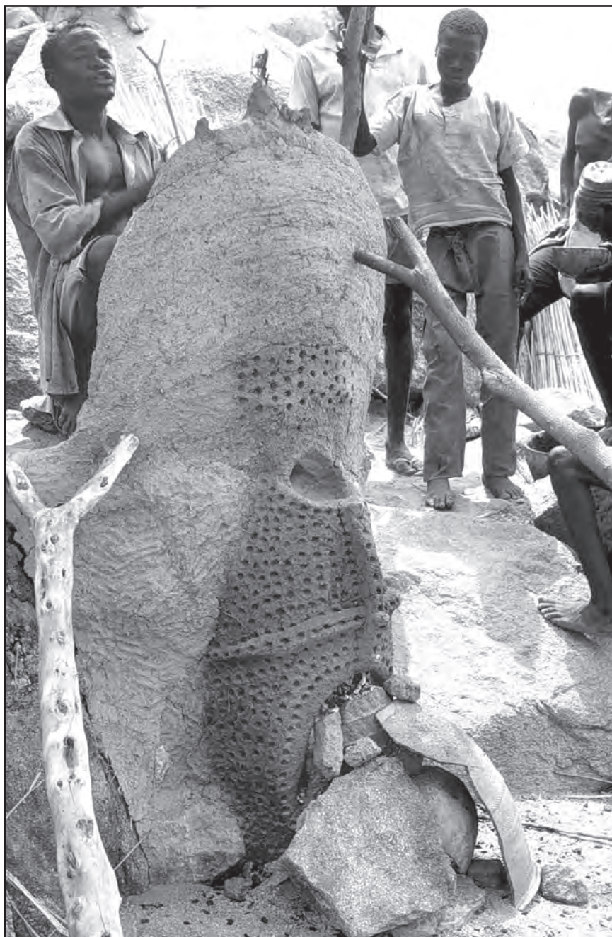
Figure 1.3. The Sukurian furnace built by Plata smelter Ajokfa in use in 1989. Note the poor closing of the furnace shaft. Photo: David Killick.
