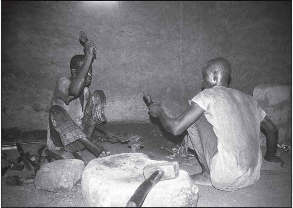
Figure 6.3. Smith (left) and bellowsman/striker beat out a hoe in a Manaouatchi (Wandala) forge. The latter's body obscures the bellows but the shallow hearth can be seen beneath his left elbow. Note the sledge hammer on the main anvil. Photo: Ian Robertson.
