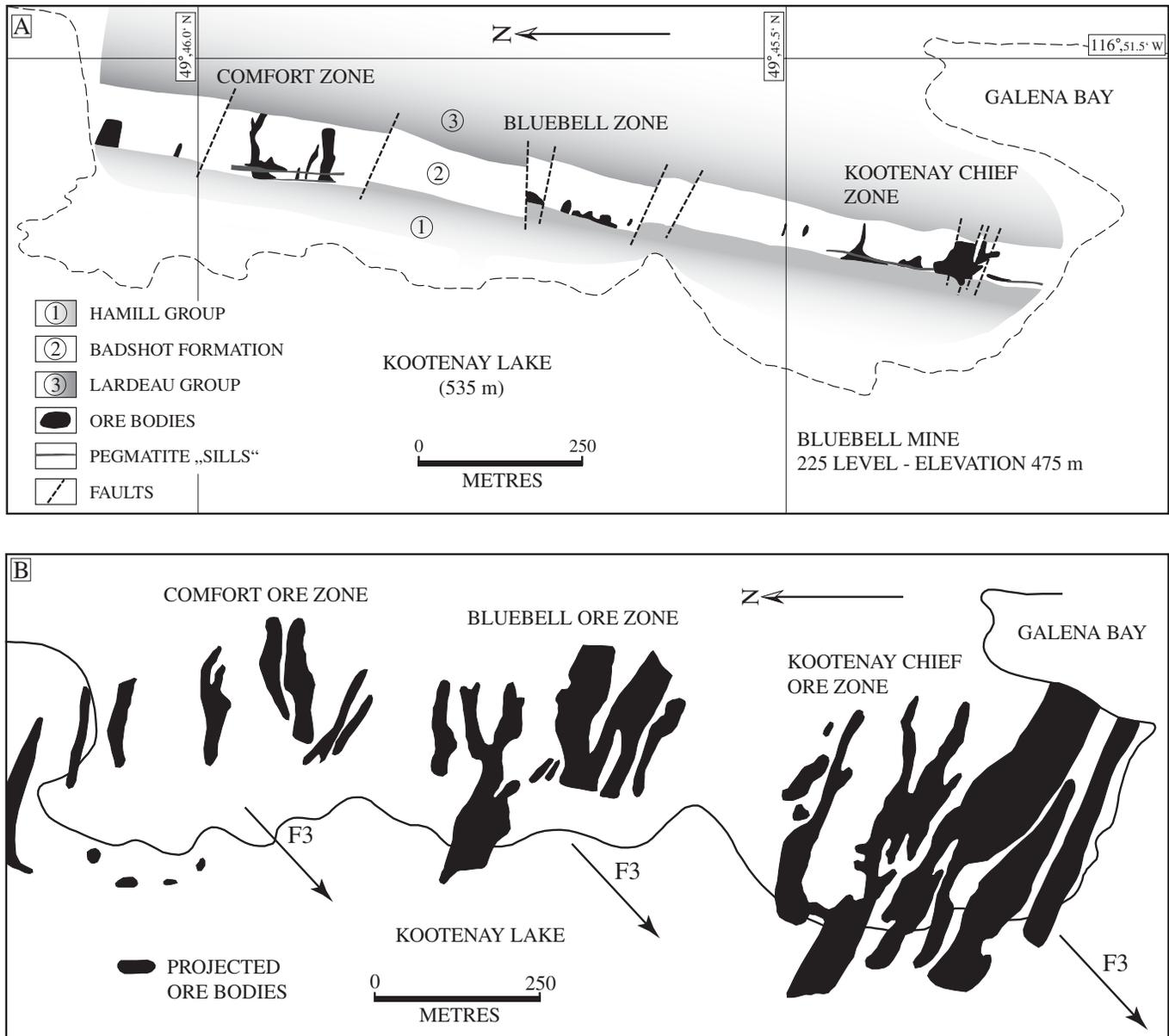
FIG. 4. A) Plan of the 225 level of the Bluebell mine. The outline of the Riondel peninsula is also shown. Adapted from Irvine (1957). B) Plan of the Bluebell mine showing the projection of orebodies onto the surface, from Shannon (1970).
