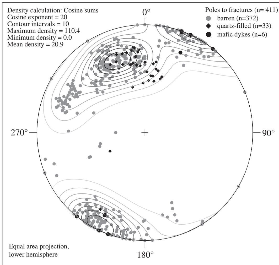
FIG. 9. Equal area lower hemisphere stereonet showing contoured poles to brittle fractures in the Hamill Group (hanging wall), directly to the west of the Comfort and Bluebell ore zones. There are two dominant orientations. The fracture set trending west-northwest is mineralized and hosts mafic dikes. Fractures trending east-northeast are commonly filled with quartz. A third set of fractures, striking north-northeast, is locally developed.
