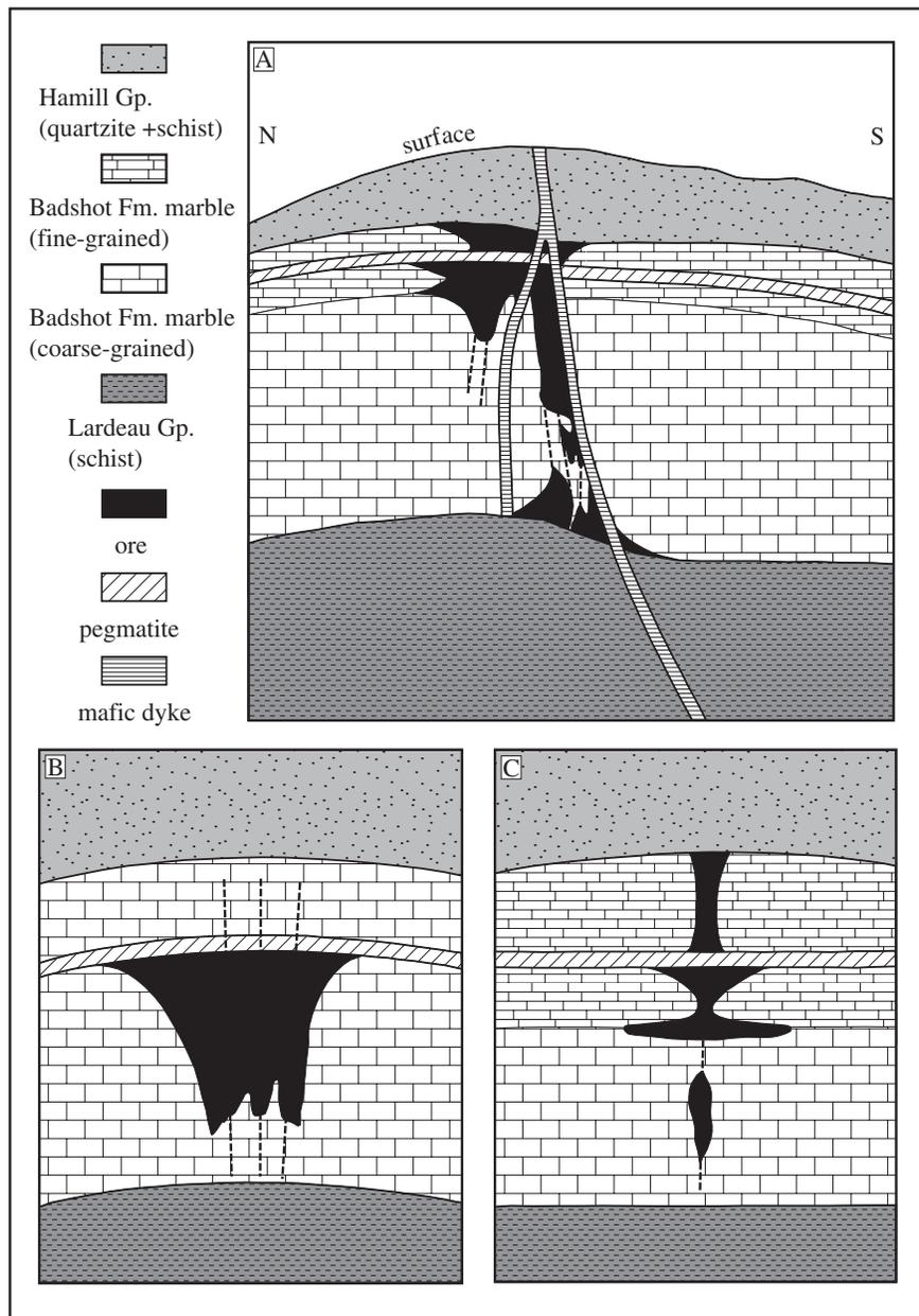
FIG. 7. Examples of longitudinal profiles through Bluebell orebodies. These show the influence on ore location exerted by fractures (A), mafic dikes (A), pegmatite (B, C) and lithology (A, C). From Shannon (1970).
