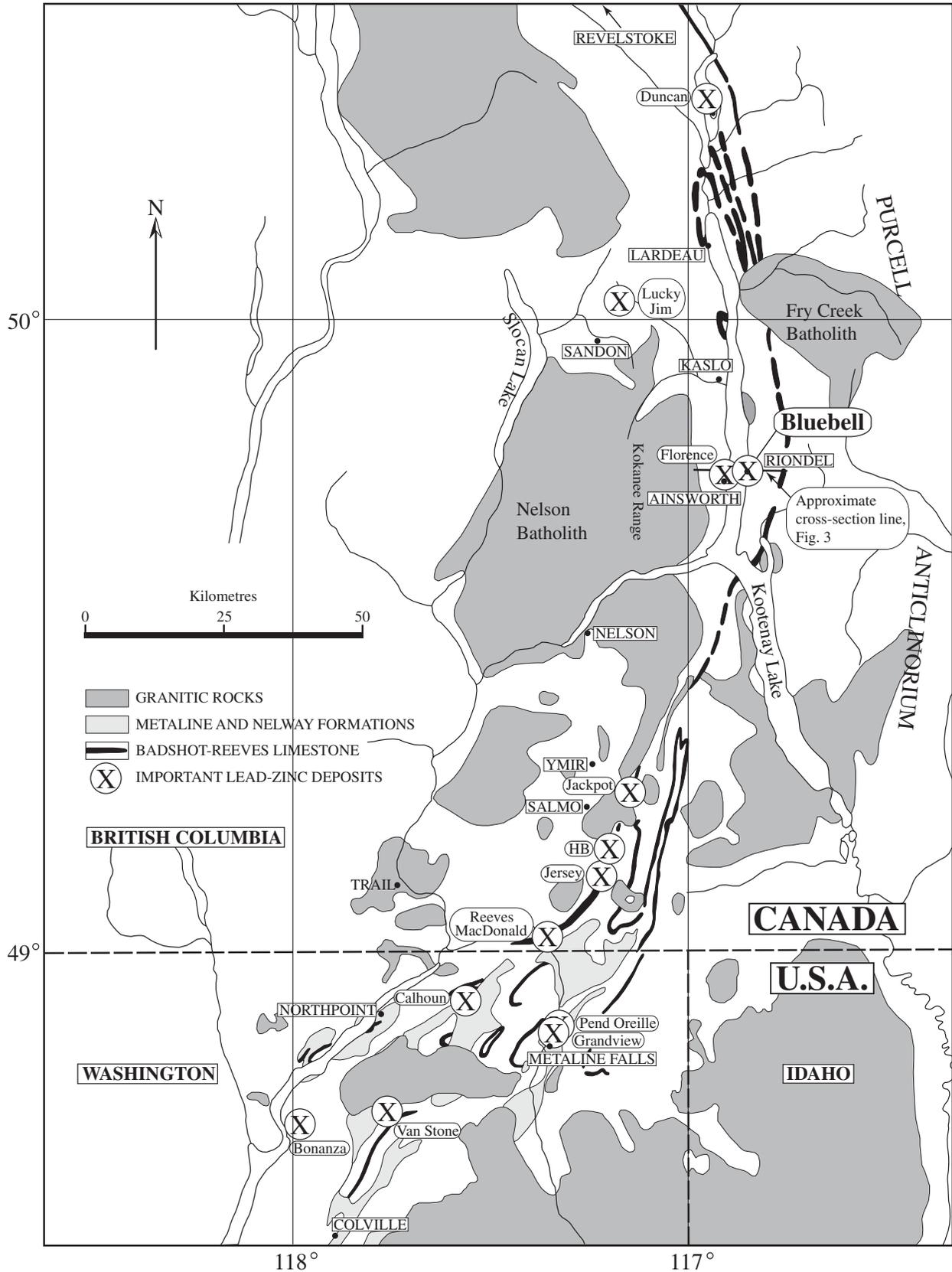
FIG. 1. Map of the Kootenay Arc showing the location of important lead-zinc deposits, igneous rocks, and major host carbonate units. The approximate line of section from Figure 3 is also shown. The name "Kootenay Arc" refers to the arcuate shape of the belt rather than to a magmatic arc. After Fyles (1970).
