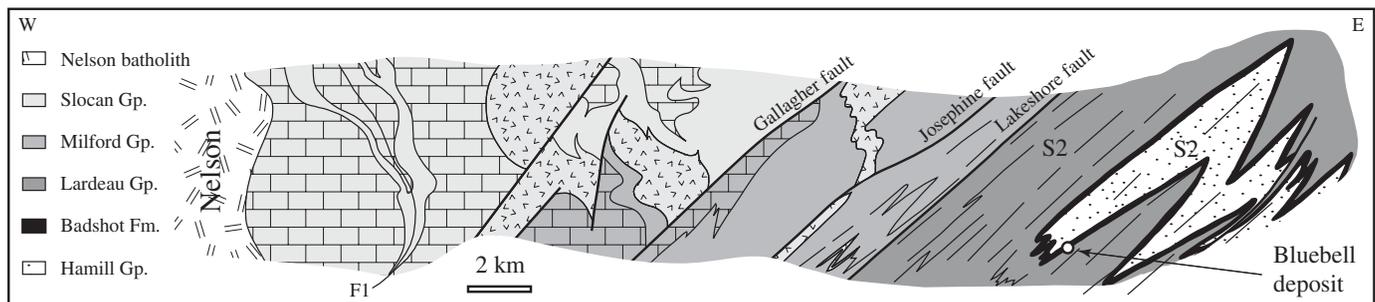
FIG. 3. Cross section across the central Kootenay Arc, showing the location of the Bluebell mine on the overturned limb of a refolded fold nappe. The approximate line of section is marked on Figure 1. The normal faults around Ainsworth, on the west side of Kootenay Lake, are labeled. From Fyles and Read (1981), based on Fyles (1967) and Hoy (1980).
