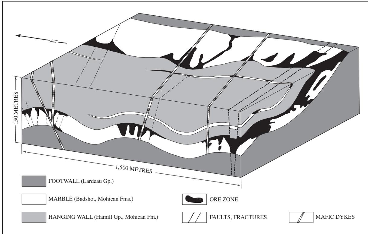
FIG. 12. Block diagram of the Bluebell mine area, reproduced from Shannon (1970). Similar diagrams appear in Ohmoto and Rye (1970), Ohmoto (1971), and Nelson (1991). Three antiforms are shown, with mineralization developed in the outer arcs of antiforms, parallel to fractures. Note the vertical exaggeration. This geometry is not supported by data presented here. See discussion in text.
