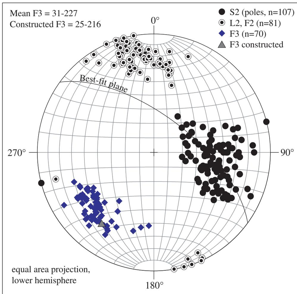
FIG. 6. Equal area lower hemisphere stereonet showing the orientation of ductile structures on the Riondel peninsula.  $S_2$  and  $L_2$  are gently folded around southwest-plunging  $F_3$  folds. “ $L_2$ ” includes minor  $F_2$  fold axes,  $S_2/S_0$  intersection lineations and  $L_2$  mineral lineations as these are invariably parallel to one another in this area.
