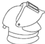
Class 7D Respirator facepiece with loose-fitting hood or helmet for non-ionizing radiation protection
