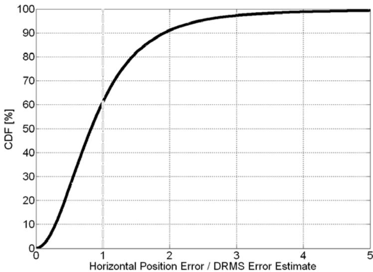
*Fig. 53. Garage: Empirical Distribution of the Ratio Between Horizontal Position Error and DRMS Error Estimate.*
