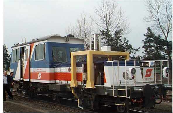
Figure 2: Self propelled trolley of the Austrian railways (ÖBB) used for track measurements with measurement platform mounted.
