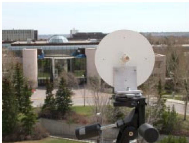
Directional Antenna Pointing at MacEwan Student Centre for Indoor Location Tests
