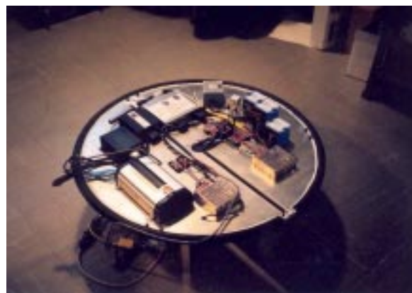
UofC GPS Receiver on the instrument platform of the Large Adaptive Reflector Telescope Prototype at the Dominion Radio Astrophysical Observatory, Penticton, BC (left). This receiver, along with the base station receiver (above) will provide cm-level positioning for the telescope focal point which will be suspended from a blimp 500m above the reflector below.
