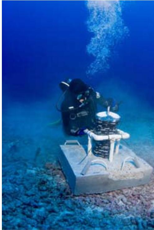
**Figure 1.6 Bottom Mounted Sonar systems (Source: [oceanexplorer.noaa.gov](http://oceanexplorer.noaa.gov))**
