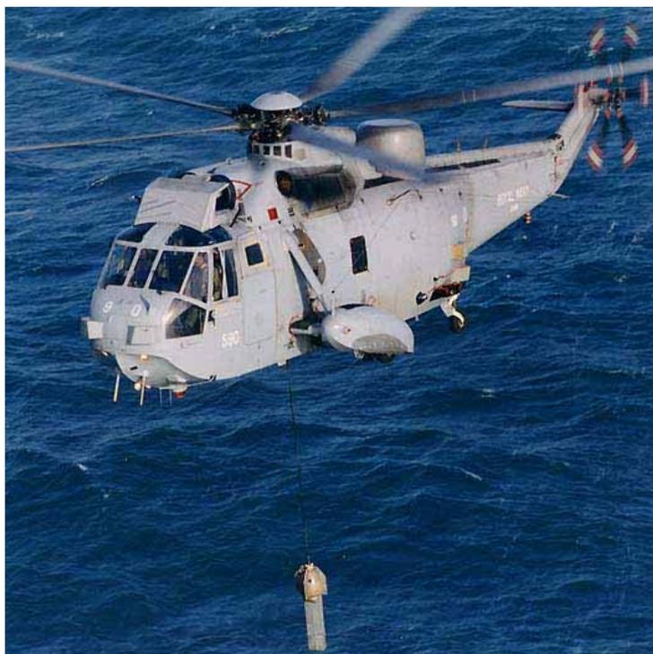
**Figure 1.3 Dipping Sonar System** (Source: [www.dutchsubmarines.com](http://www.dutchsubmarines.com))
