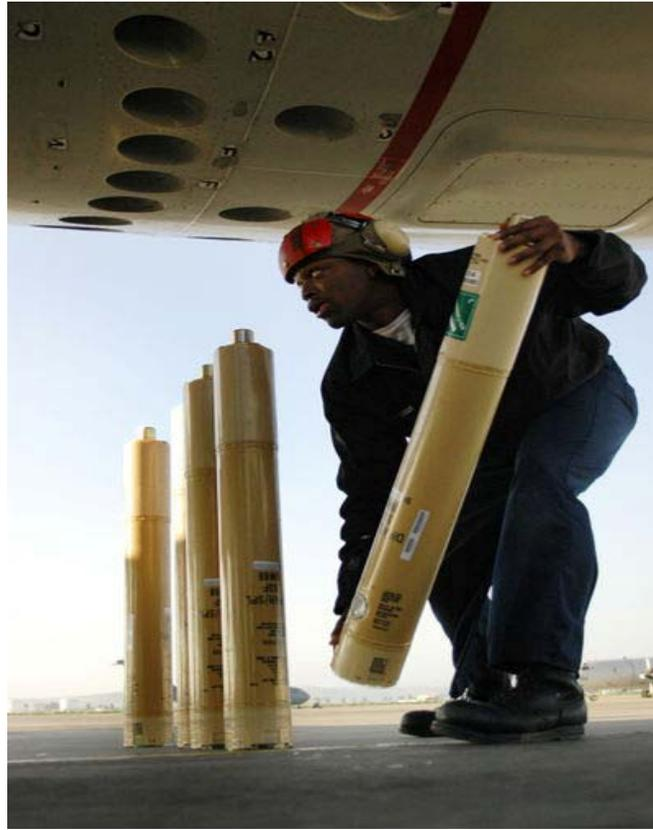
Figure 1.7 Sonobuoy loaded on aircraft (Source: <http://www.navy.mil>)
