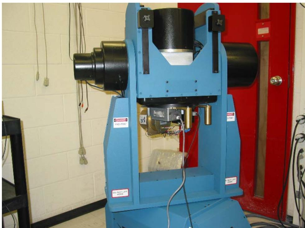
**Figure 5.9: Drilling Simulation Test—Rotation Table in Highly Inclined Section**
