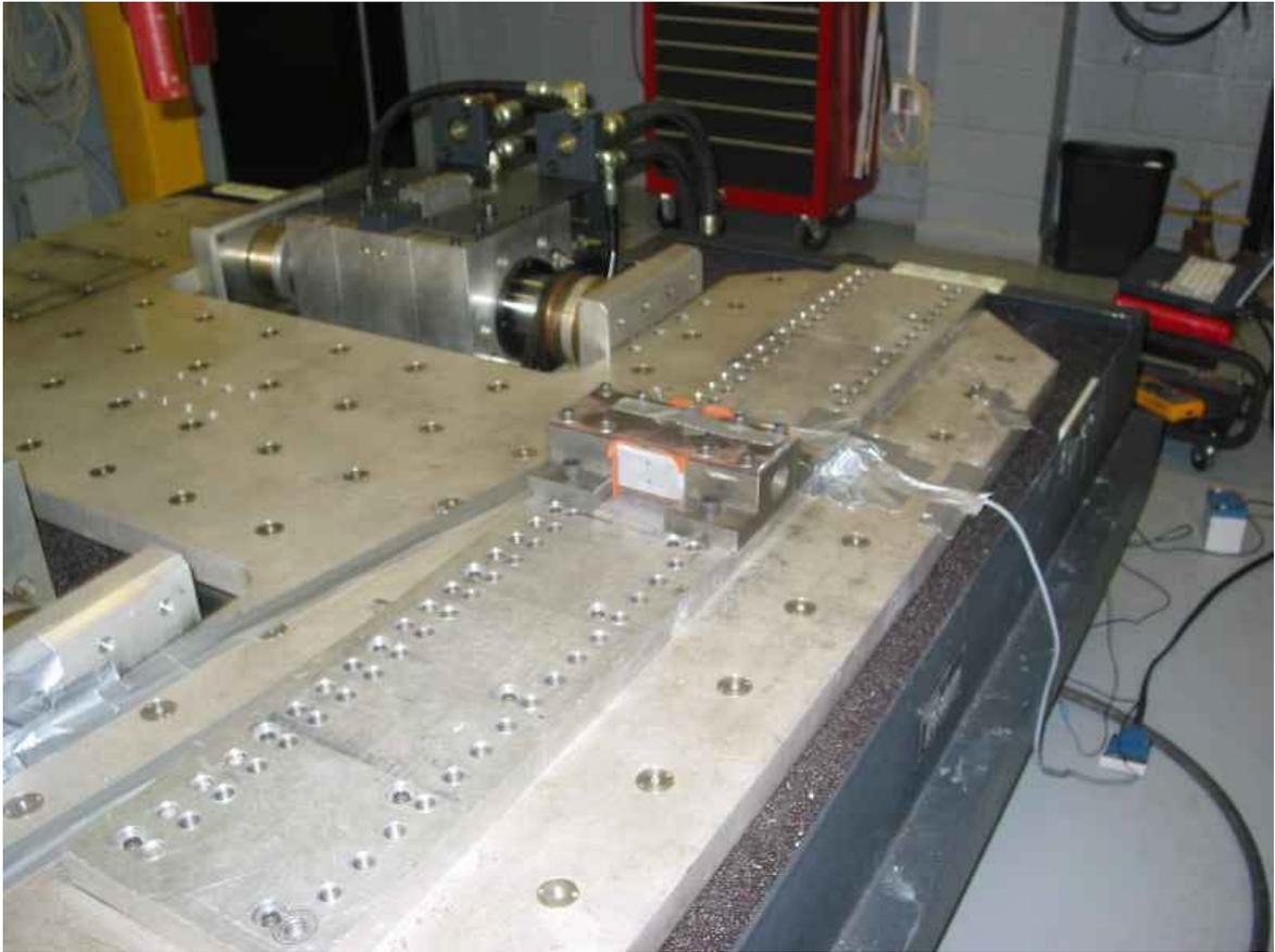
**Figure 3.7: Sensors Package Installed on the Vibration Table**
