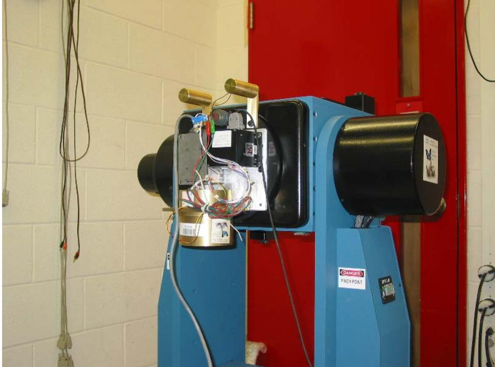
**Figure 5.7: Drilling Simulation Test—Rotation Table in Vertical Position**
