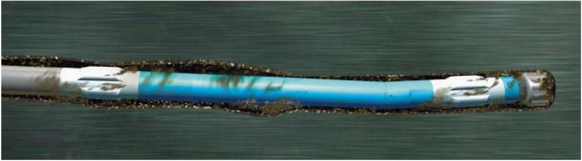
**Figure 2.2: Conventional PDM Motor behind the Drill Bit [Berger et al., 1999]**
