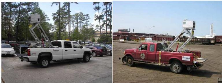
Figure 3.13: The TITANs mounted on the hydraulic racks built on trucks
