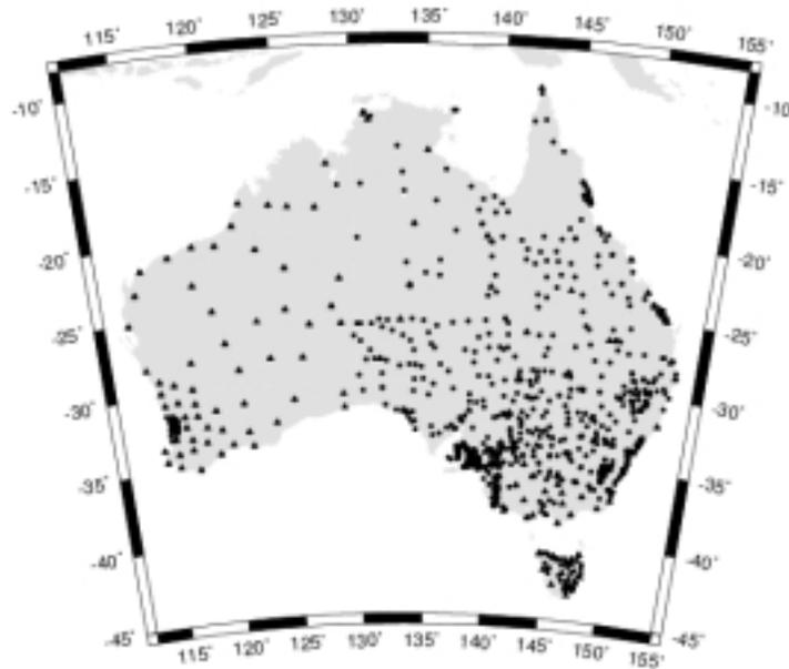
**Figure 4.11:** GPS-levelling data on the Australian mainland (according to Featherstone and Guo, 2001)
