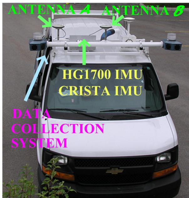
**Figure 3.1 Vehicle Test Setup**
