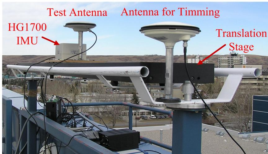
**Figure 4.5 Translation Stage Test Setup**
