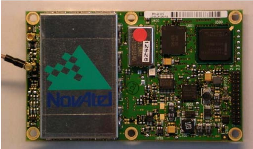
**Figure 4-1: NovAtel OEM4-G2L Dual-Frequency GPS Receiver (125X85 mm)
