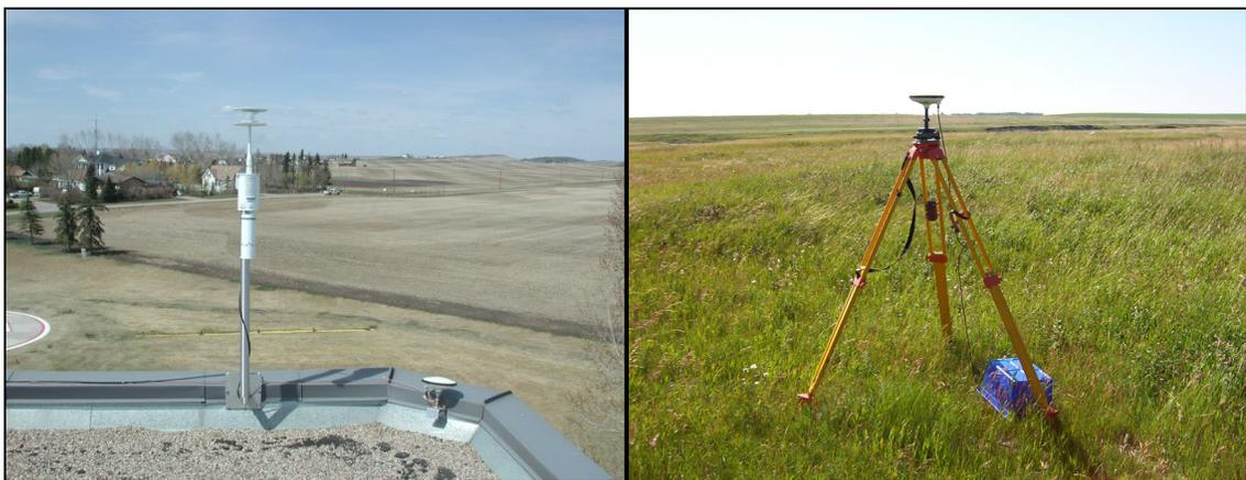
Figure 5.2 GPS Reference Remote (left) and Local (right) Station Setup
