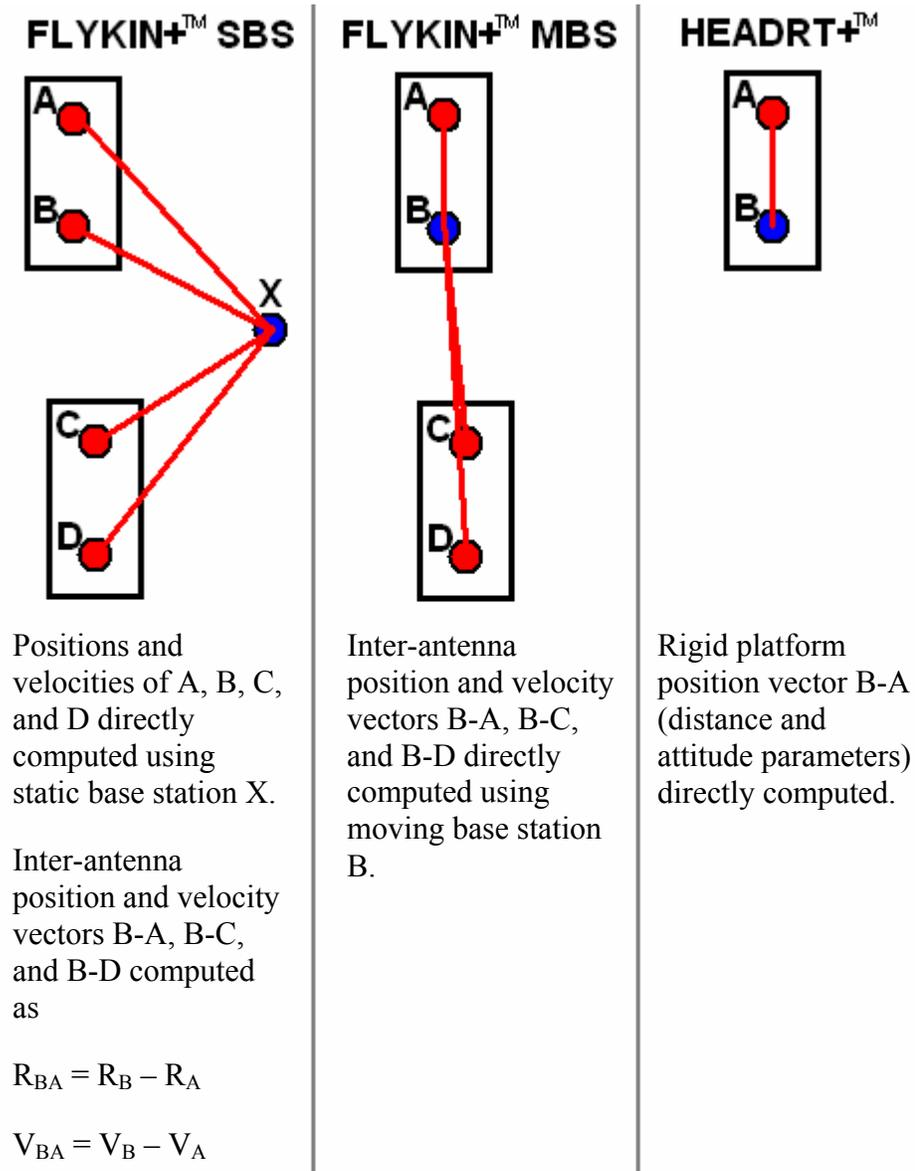
**Figure 3.8: Graphical Representation of Three Processing Techniques**
