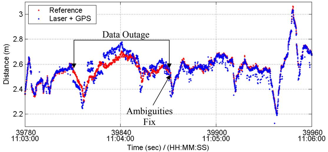
**Figure 4.41: GPS+Laser-Measured Distance during Dynamic Data Outage Period using Pitch Constraint**
