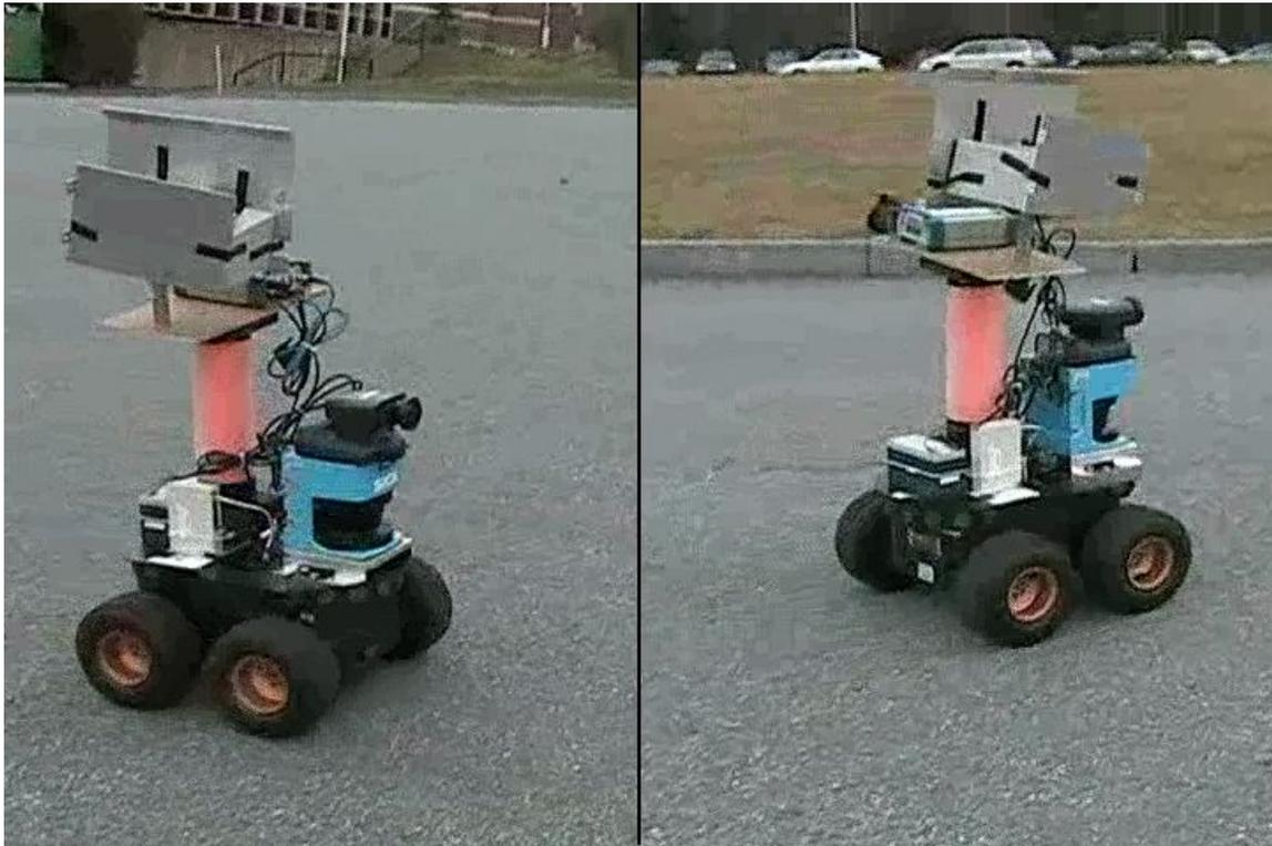
**Figure 4.64: Follower Robot with Home Made GPS Blockage Box Mounted**
