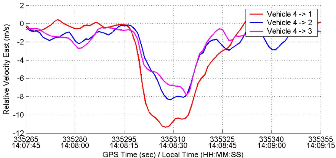
**Figure 3.29: Relative Velocity East (Along-Track) during Passing Manoeuvre**
