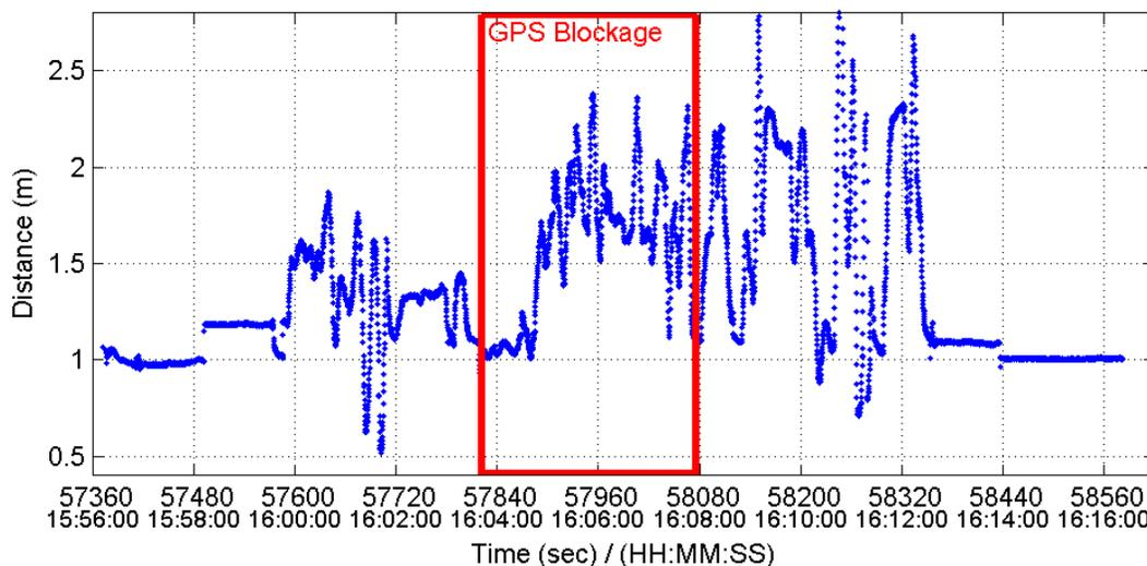
**Figure 4.66: Real-Time (GPS+Camera) Measured Distance during GPS Blockage Real-Time Test**
