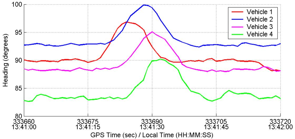
**Figure 3.18: Time Lags in Heading Curves of Vehicles in a Platoon**
