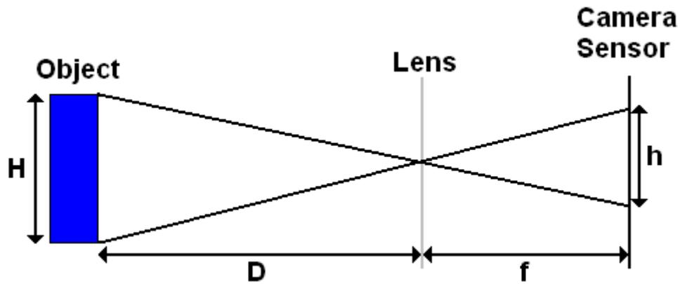
**Figure 2.1: Relationship Between Real-World and Image for Distance Computation**
