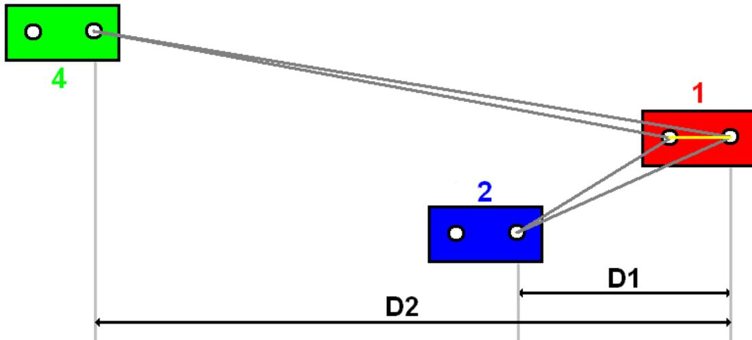
**Figure 3.30: Computation of Inter-Antenna Vector on Vehicle 1 Using Other Vehicles as Base Stations at Varying Distances**
