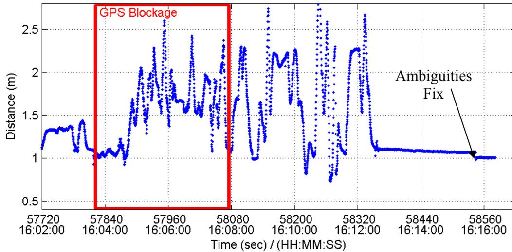
**Figure 4.72: GPS+Camera+Laser-Measured Distance during GPS Blockage Real-Time Test**
