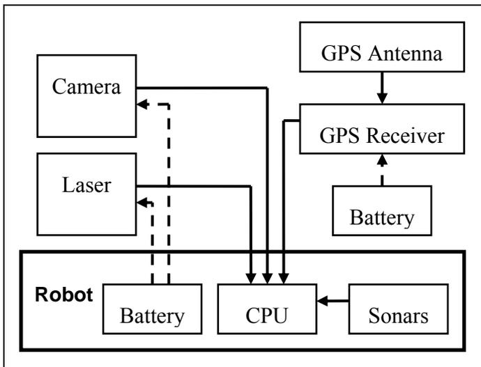
**Figure 4.2: Layout of Sensors on Follower Robot**
