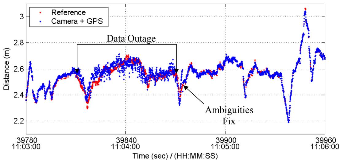
**Figure 4.40: GPS+Camera-Measured Distance during Dynamic Data Outage Period using Pitch Constraint**
