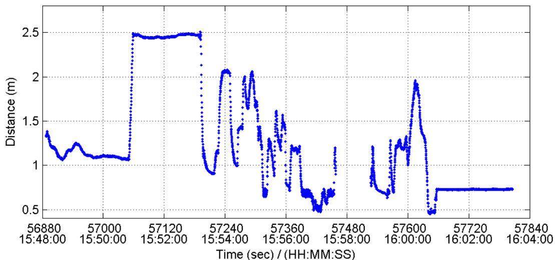
**Figure 4.55: GPS-Measured Distance during All Sensors Real-Time Test**
