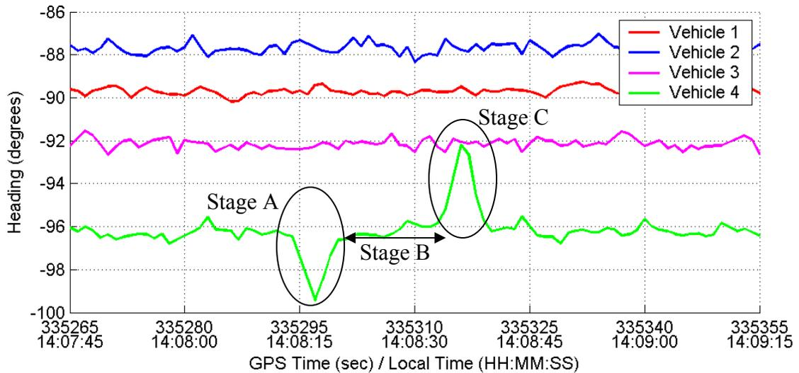
**Figure 3.25: Vehicle Headings during a Passing Manoeuvre**
