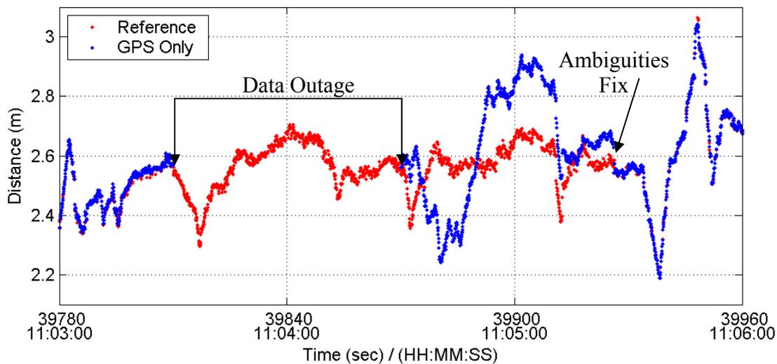
**Figure 4.39: GPS-Measured Distance during Dynamic Data Outage Period using Pitch Constraint**
