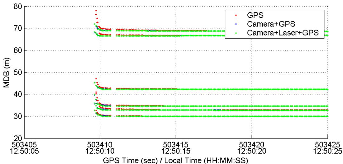
**Figure 4.43: MDB for Code Observations at the Beginning of the Test**
