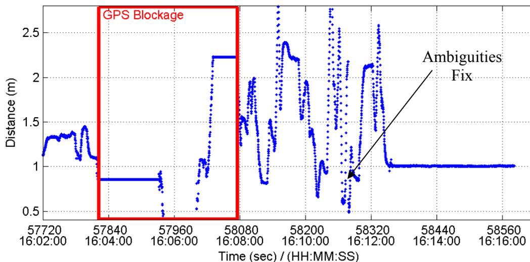
**Figure 4.67: GPS-Measured Distance during GPS Blockage Real-Time Test**
