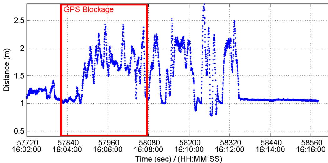
**Figure 4.68: Camera-Measured Distance during GPS Blockage Real-Time Test**
