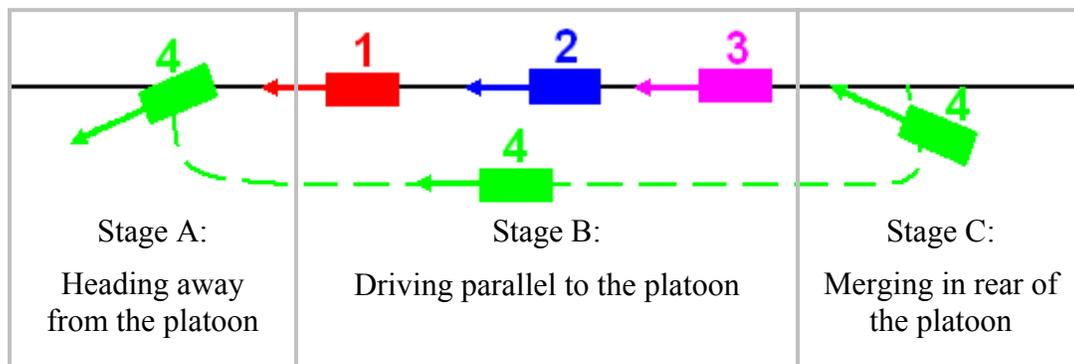
**Figure 3.24: Stages in the Passing Manoeuvre**
