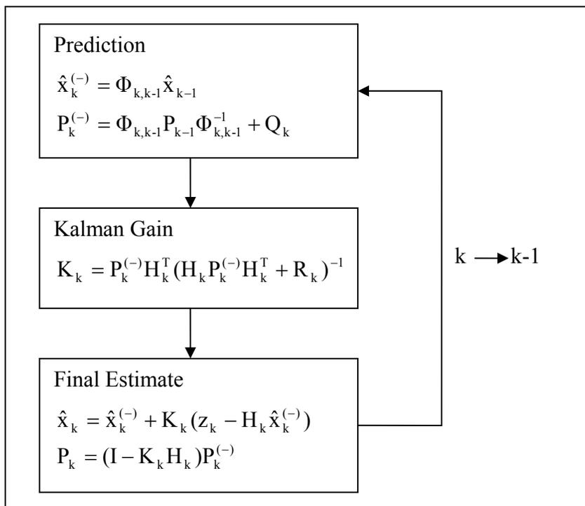
**Figure 2.4: Flow Chart of Kalman Filtering**
