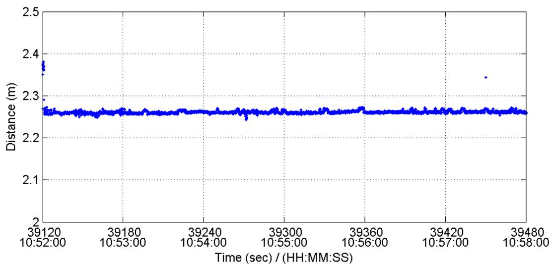
**Figure 4.24: GPS+Laser-Measured Distance during Static Time**
