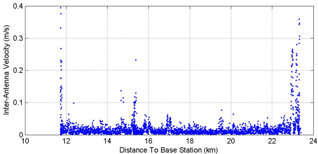
**Figure 3.36: Inter-Antenna Velocity on Vehicle 1 Measured From U of C Base Station with respect to Distance From Base Station**
