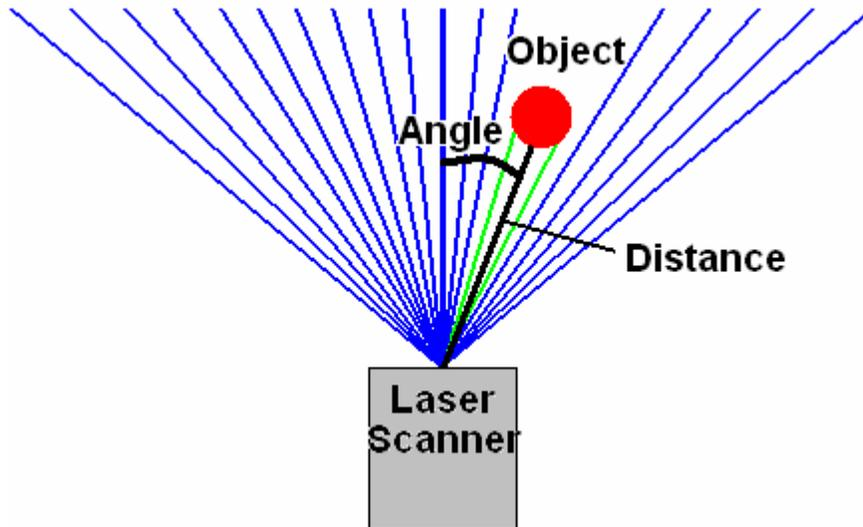
**Figure 2.3: Laser Scanner Detecting an Object to Measure Distance and Angle**
