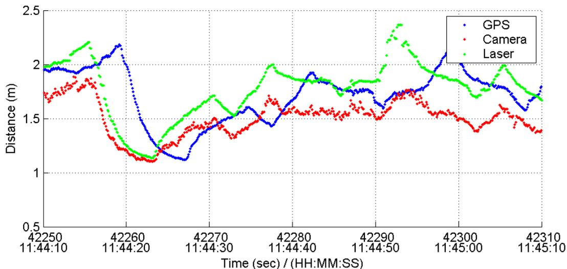
**Figure 4.49: GPS, Camera, and Laser Output during Kinematic Period, Showing GPS Time Lag**
