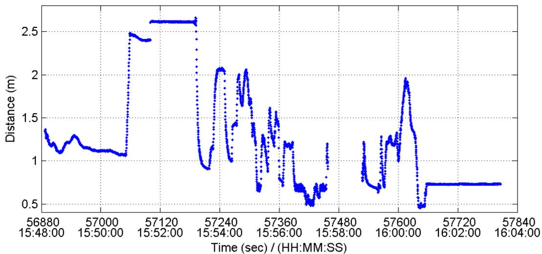
**Figure 4.61: GPS-Measured Distance during All Sensors Real-Time Test using Pitch Constraint**
