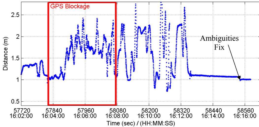
**Figure 4.70: GPS+Camera-Measured Distance during GPS Blockage Real-Time Test**
