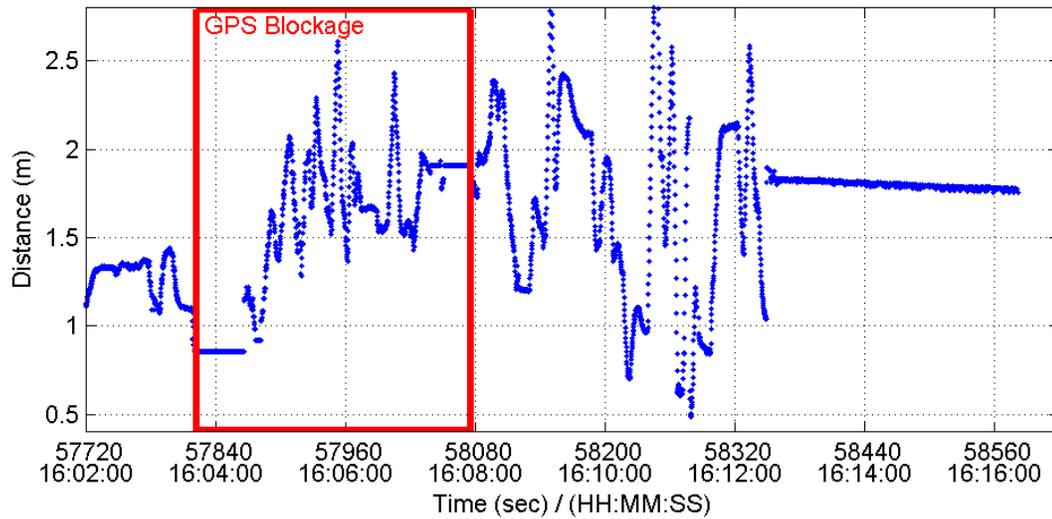
**Figure 4.71: GPS+Laser-Measured Distance during GPS Blockage Real-Time Test**
