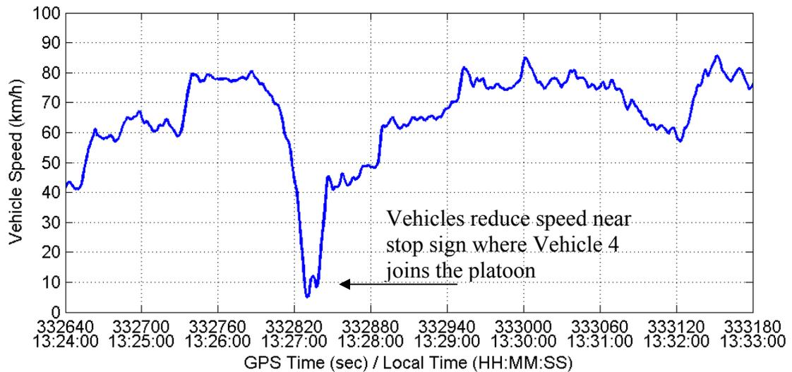
**Figure 3.19: Speed of Vehicle 3 during One Run**
