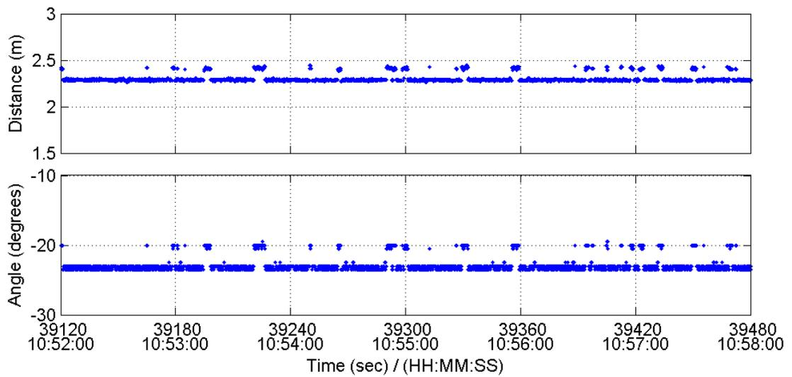
**Figure 4.15: Distribution of Raw Laser Measurements during Static Period**
