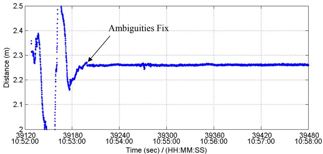
**Figure 4.20: GPS-Measured Distance during Static Time**
