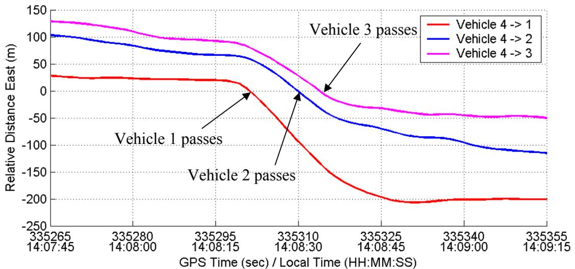
**Figure 3.27: Relative Distance East (Along-Track) during Passing Manoeuvre**
