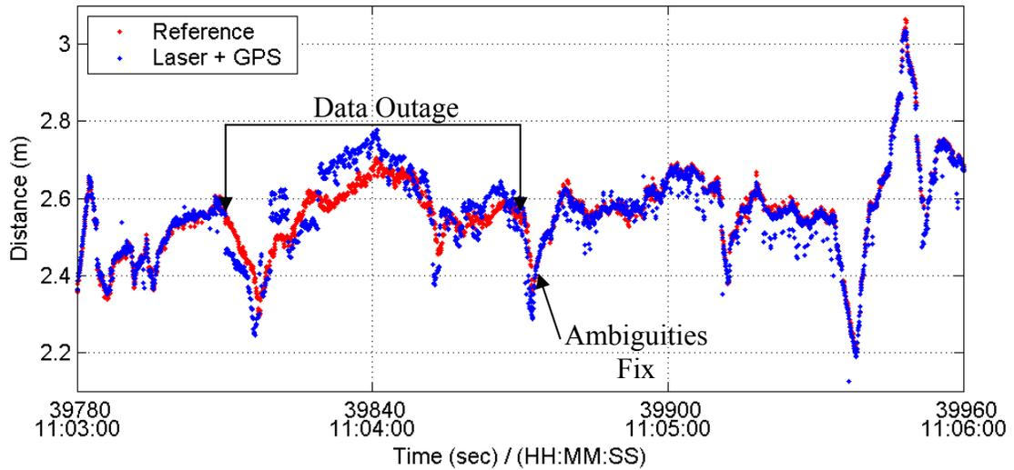
**Figure 4.38: GPS+Laser-Measured Distance during Dynamic Data Outage Period**
