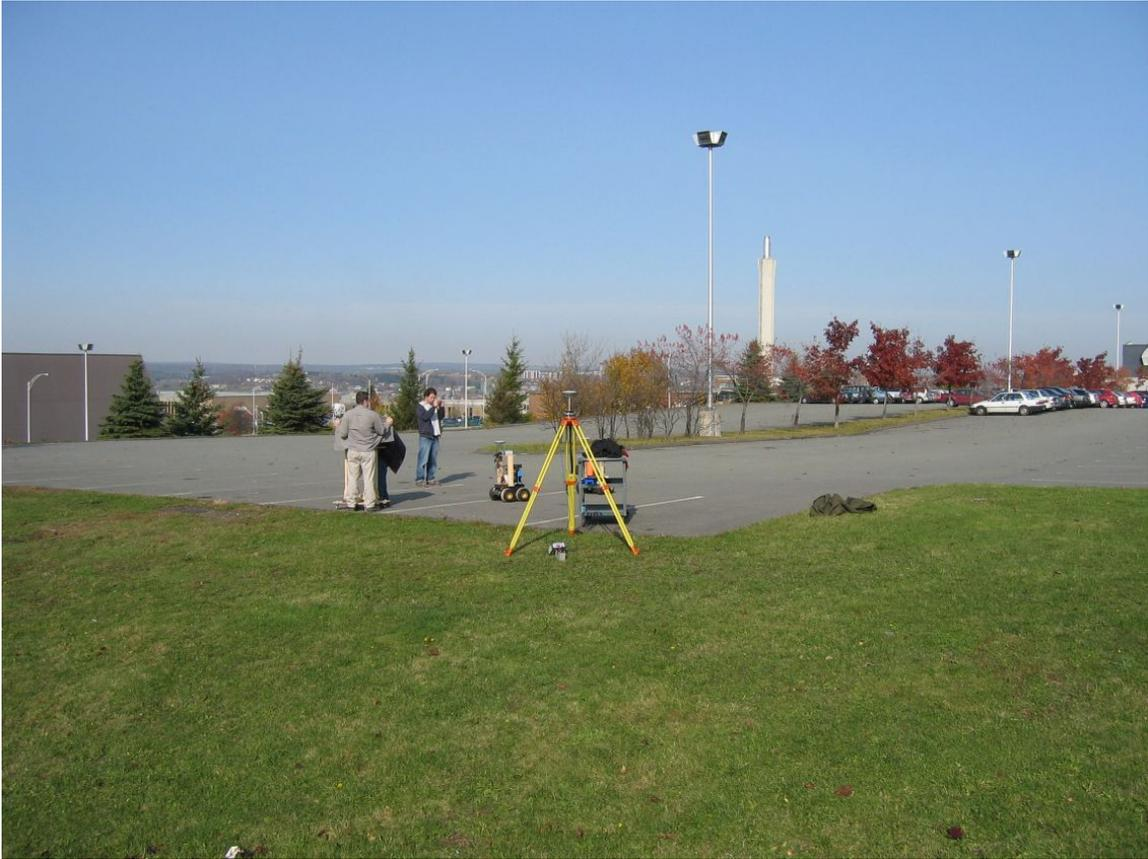
**Figure 4.11: Example of Reference Station Setup**
