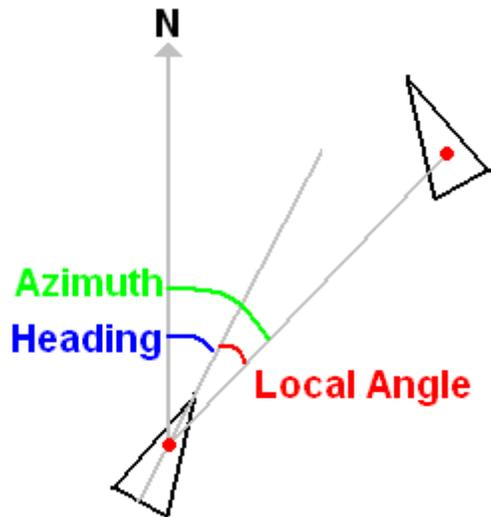
**Figure 4.3: Relationship Between Azimuth, Heading, and Local Angle**
