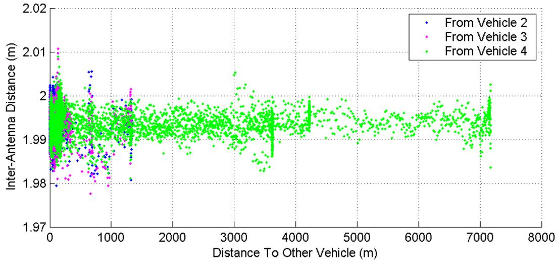
**Figure 3.32: Inter-Antenna Baseline on Vehicle 1 Measured From Other Vehicles with respect to Distance From Other Vehicle**
