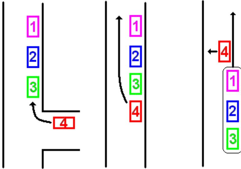
**Figure 3.7: Vehicle 4 Joins the Platoon, Passes the Platoon, and Lets the Platoon Pass**
