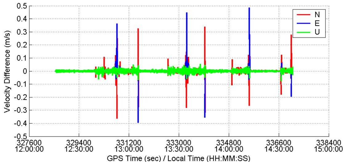
**Figure 3.13: Components of Inter-Antenna Velocity for Vehicle 2 Using FLYKIN+™ SBS Approach**
