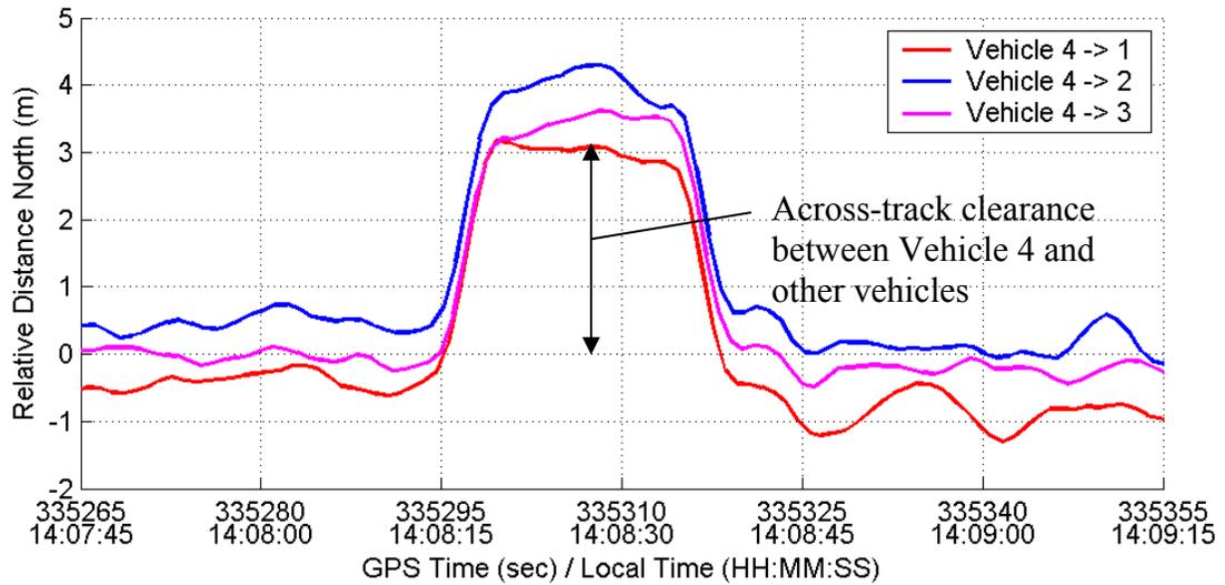
**Figure 3.26: Relative Distance North (Across-Track) during Passing Manoeuvre**
