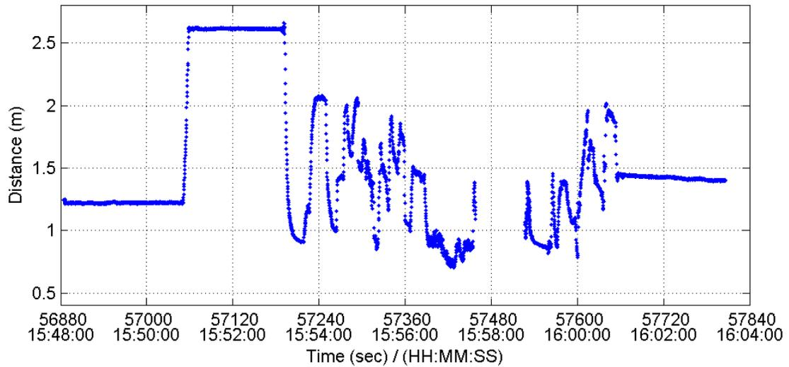
**Figure 4.63: GPS+Laser-Measured Distance during All Sensors Real-Time Test using Pitch Constraint**
