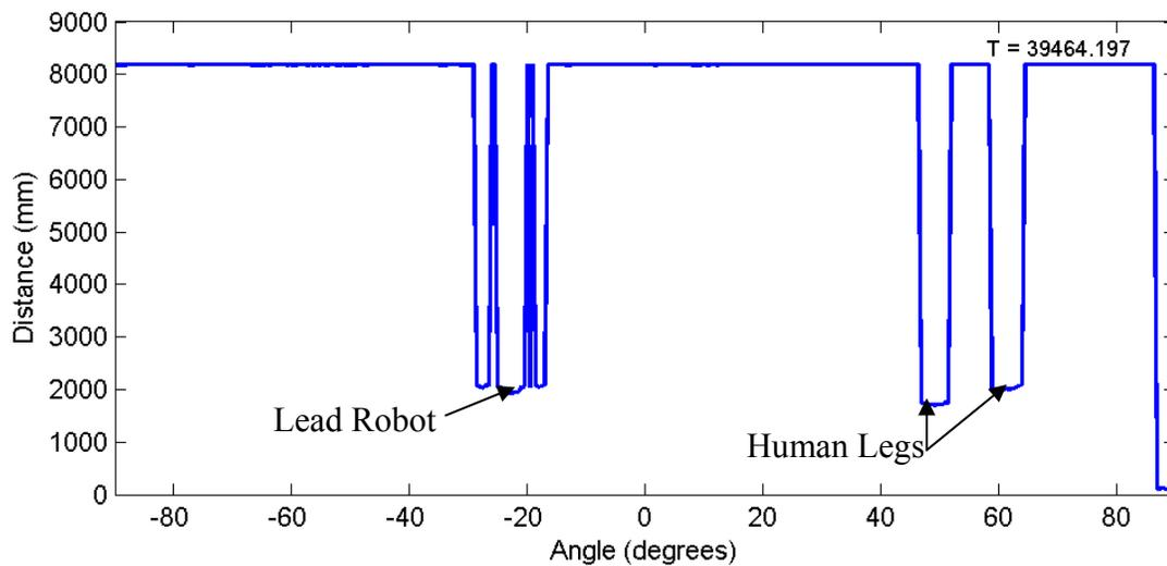
**Figure 4.6:** Laser Profile using Original Setup
