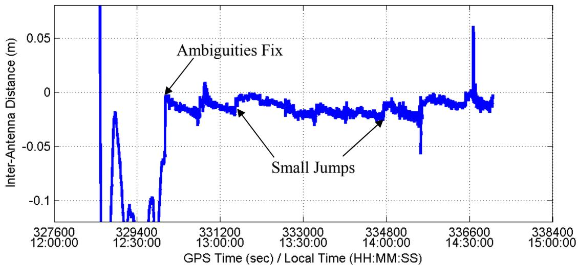
**Figure 3.11: Magnitude of Inter-Antenna Vector for Vehicle 2 Using FLYKIN+™ MBS Approach Relative to Tape Measured Distance**
