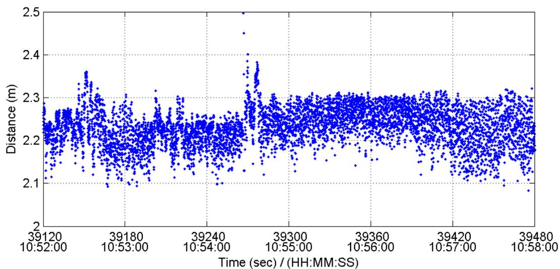
**Figure 4.21: Camera-Measured Distance during Static Time**
