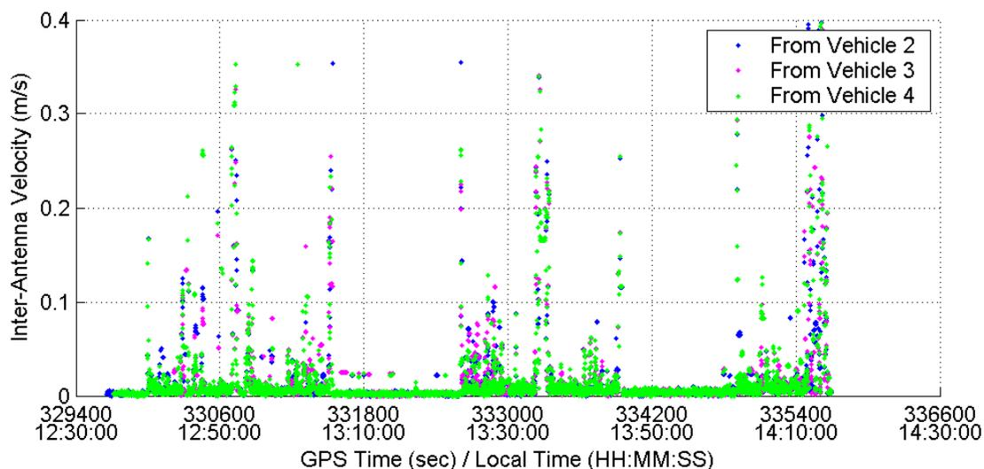
**Figure 3.34: Inter-Antenna Velocity on Vehicle 1 Measured From Other Vehicles with respect to Time**
