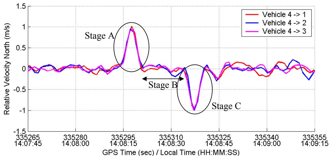
**Figure 3.28: Relative Velocity North (Across-Track) during Passing Manoeuvre**
