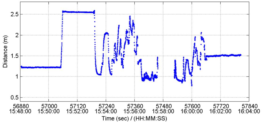
**Figure 4.60: GPS+Camera+Laser-Measured Distance during All Sensors Real-Time Test**
