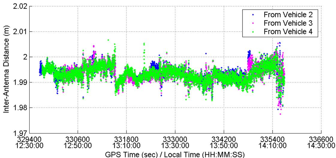
**Figure 3.31: Inter-Antenna Baseline on Vehicle 1 Measured From Other Vehicles with respect to Time**
