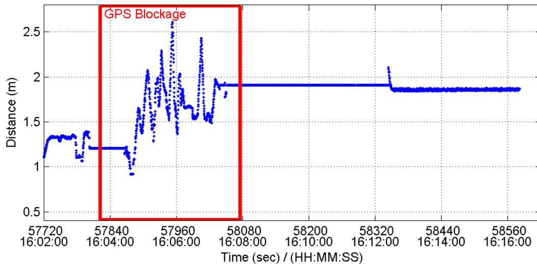
**Figure 4.69: Laser-Measured Distance during GPS Blockage Real-Time Test**
