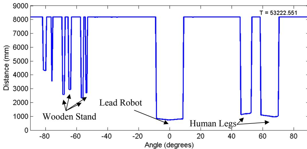
**Figure 4.8: Laser Profile using Improved Setup**
