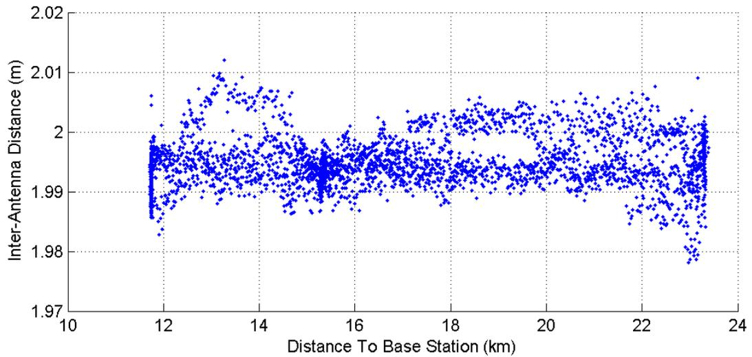
**Figure 3.33: Inter-Antenna Baseline on Vehicle 1 Measured from U of C Base Station with respect to Distance From Base Station**
