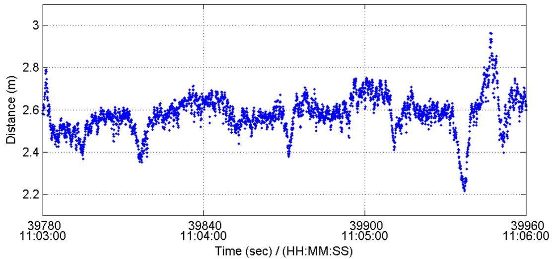
**Figure 4.31: Camera-Measured Distance during Kinematic Period**
