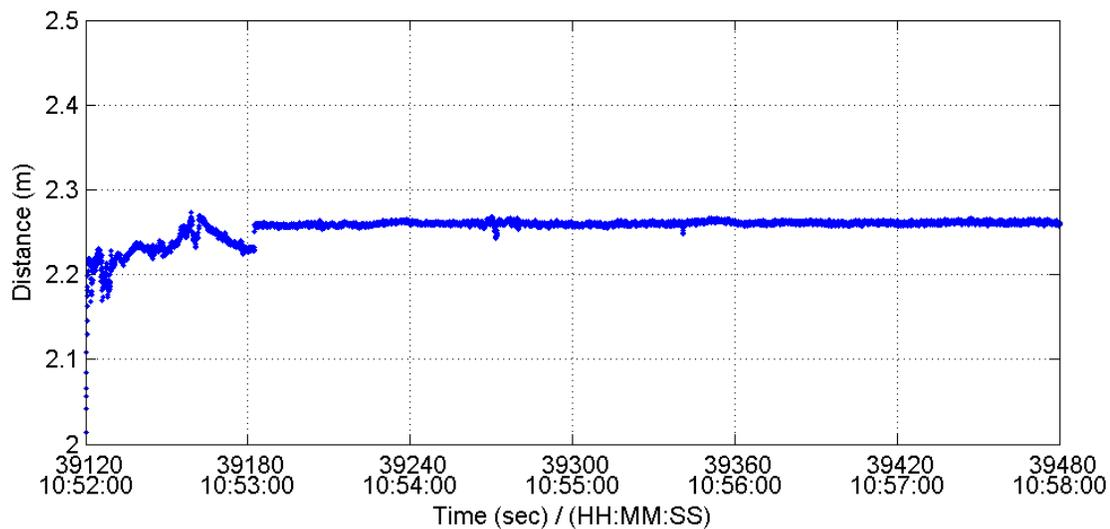
**Figure 4.23: GPS+Camera-Measured Distance during Static Time**
