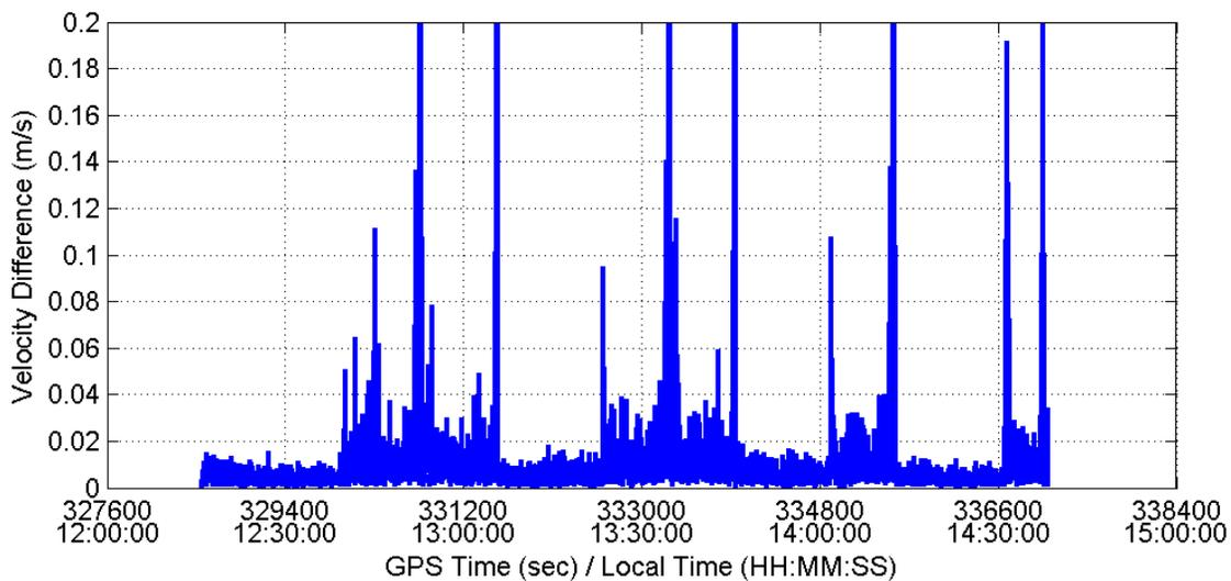
**Figure 3.14: Magnitude of Inter-Antenna Velocity Difference for Vehicle 2 Using FLYKIN+™ SBS Approach**
