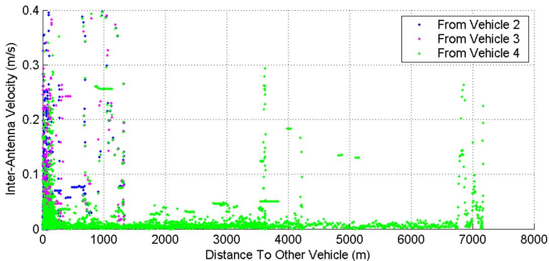
**Figure 3.35: Inter-Antenna Velocity on Vehicle 1 Measured From Other Vehicles with respect to Distance From Other Vehicle**
