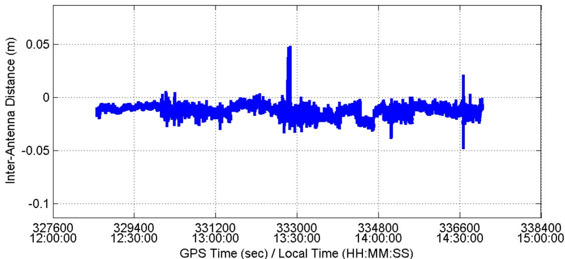
**Figure 3.12: Magnitude of Inter-Antenna Vector for Vehicle 2 Using HEADRT+™ Approach Relative to Tape Measured Distance**
