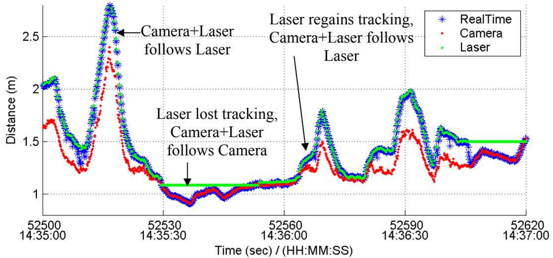
**Figure 4.51: Camera + Laser Test with Incorrect Offsets**
