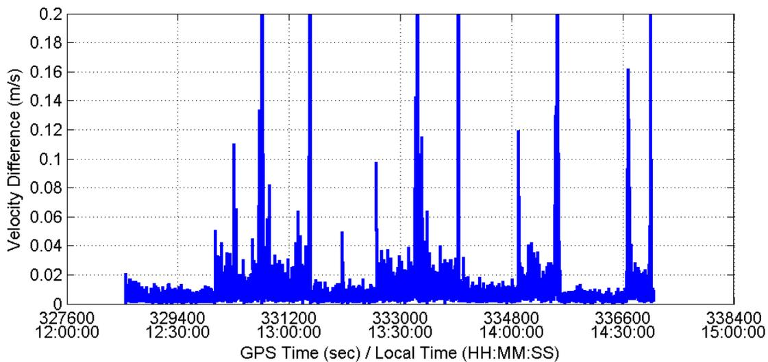
**Figure 3.15: Magnitude of Inter-Antenna Velocity Difference for Vehicle 2 Using FLYKIN+™ MBS Approach**
