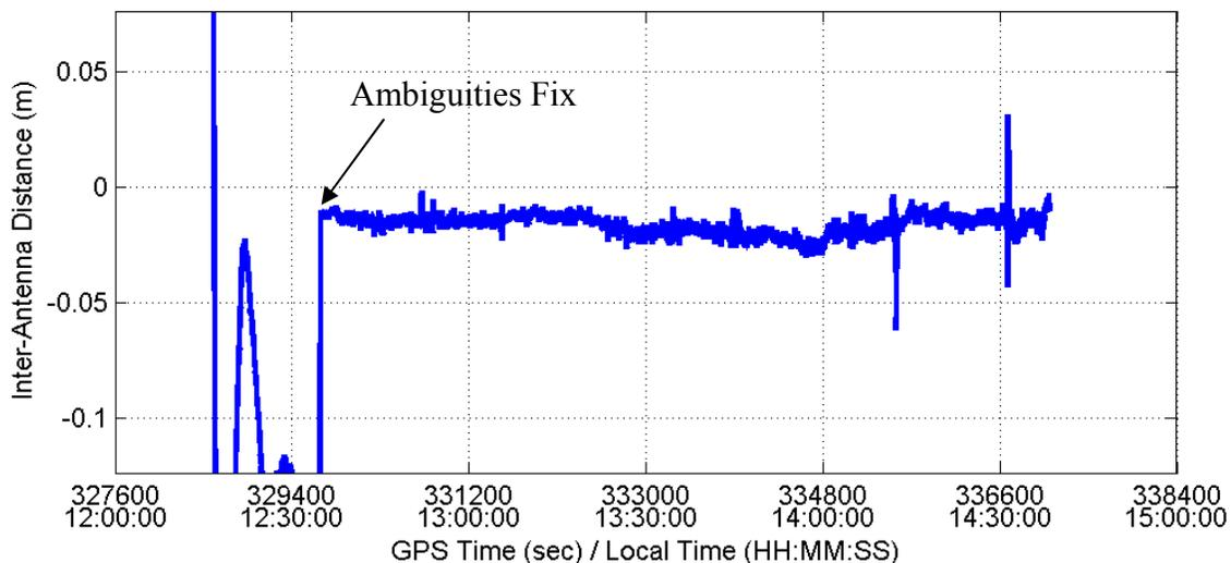
**Figure 3.10: Magnitude of Inter-Antenna Vector for Vehicle 2 Using FLYKIN+™ SBS Approach Relative to Tape Measured Distance**
