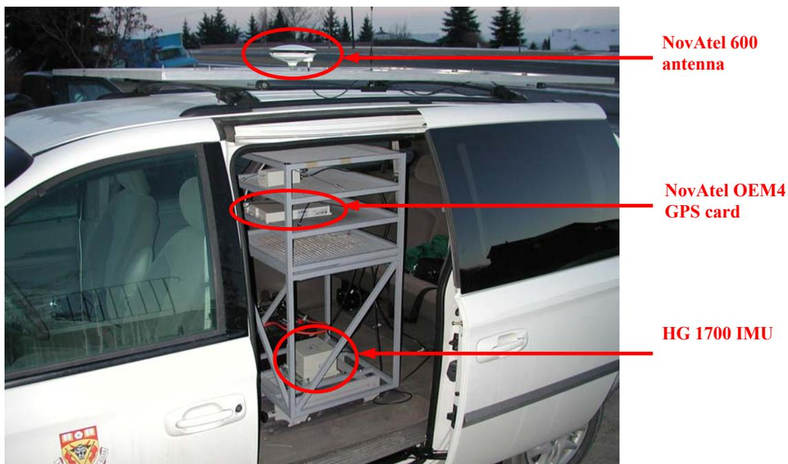
**Figure 6-2: Remote Station Set-up**
