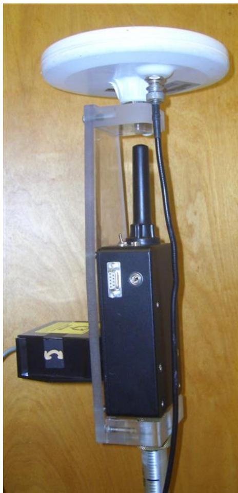
Figure 6.1: MSSSI UWB radio mount
