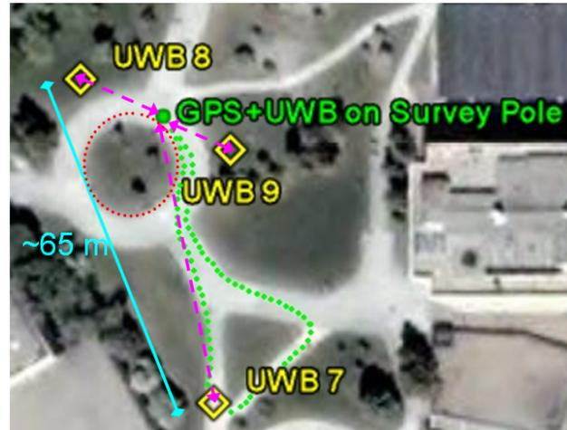
Figure 4.12: The kinematic test
