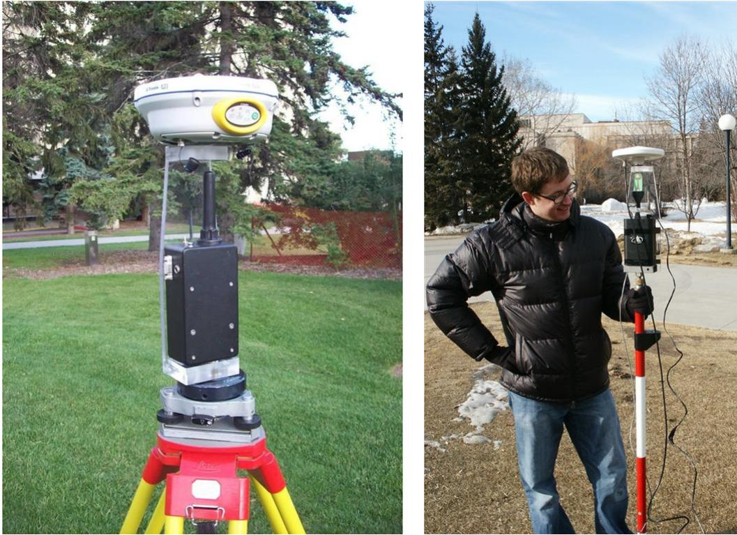
Figure 2.19: Dynamic ranging UWB and GPS using coaxial mounts
