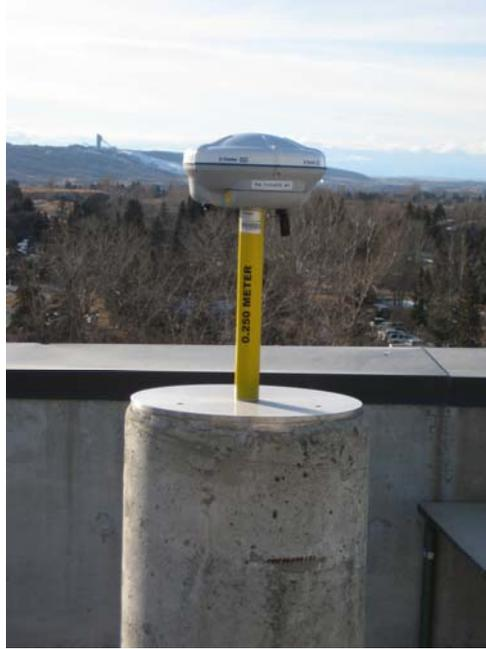
**Figure 6.2:** Trimble R8 GNSS receiver base station
