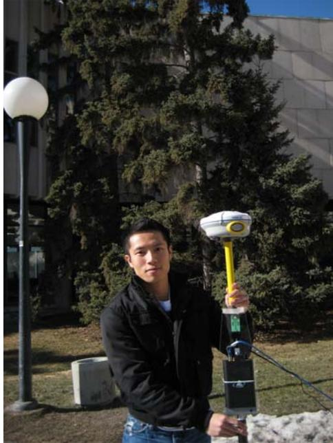
**Figure 6.5:** Trimble R8 receiver with a Time Domain UWB radio on a co-axial amount. The phase centers of both antennas are co-aligned vertically
