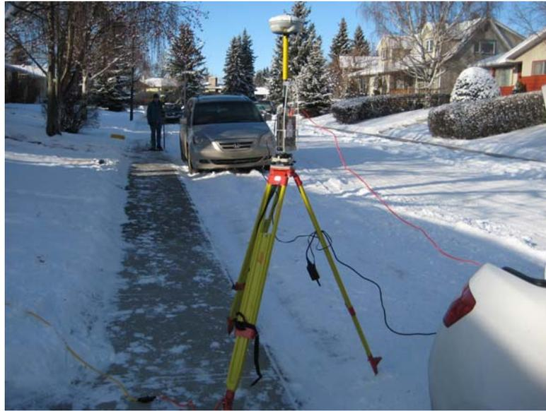
**Figure 7.5:** UWB-GPS mounted on a tripod
