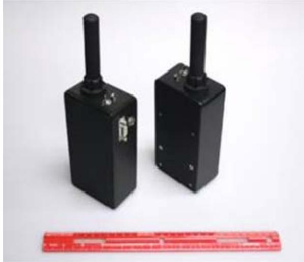
**Figure 4.3:** Multispectral Solutions (MSS) UWB radios
