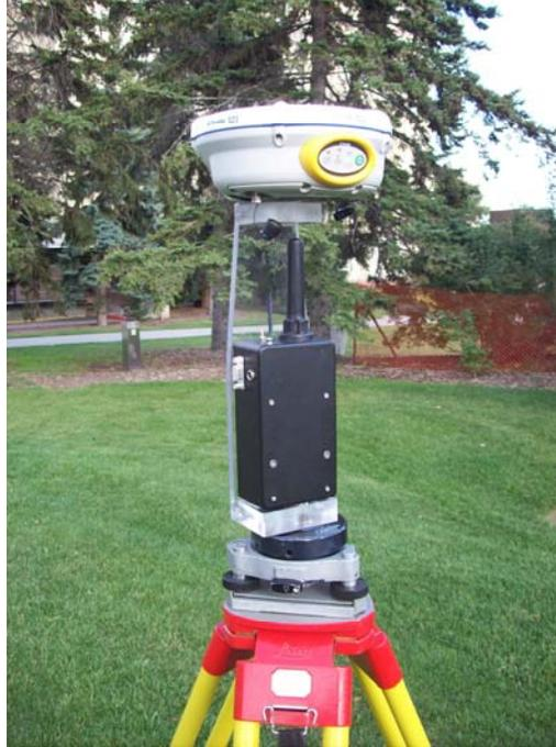
**Figure 4.5:** UWB-GPS co-axial mount
