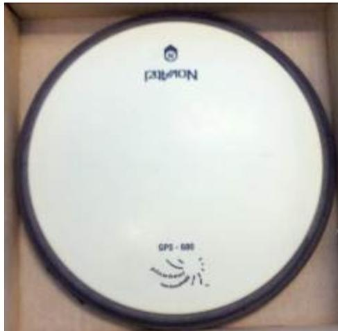
**Figure 4-3: A GPS antenna with a heading indicator**
