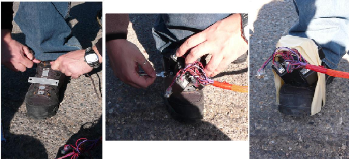
**Figure 5.20: Steps to attach GFIMU on Foot**
