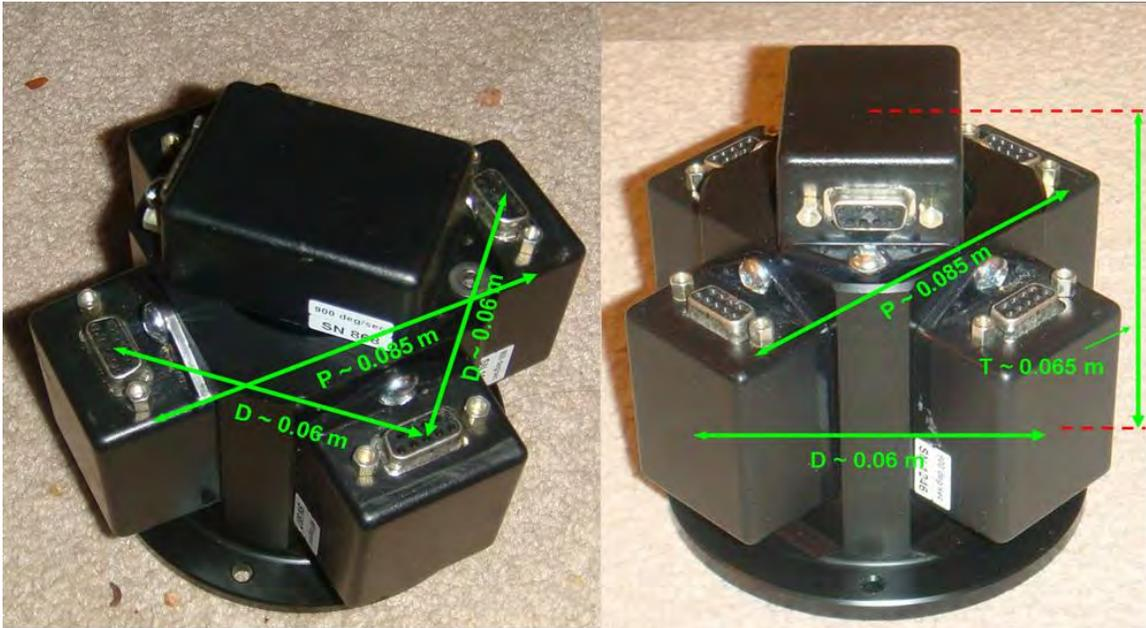
**Figure 3.2: Proposed GFIMU composed of five MEMS IMUs attached to a Delrin® block**
