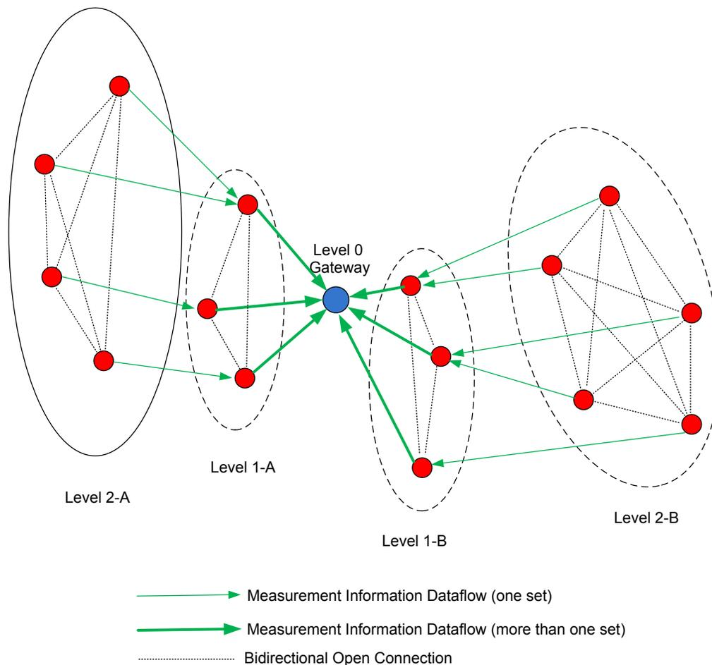
Figure 48 - WSN Centralized Architecture - Measurement Reporting Data Flow
