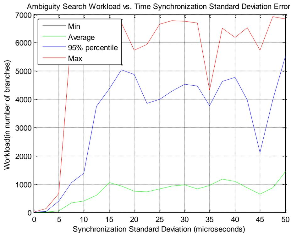
Figure 26 - Search workload vs. inter node time synchronization error
