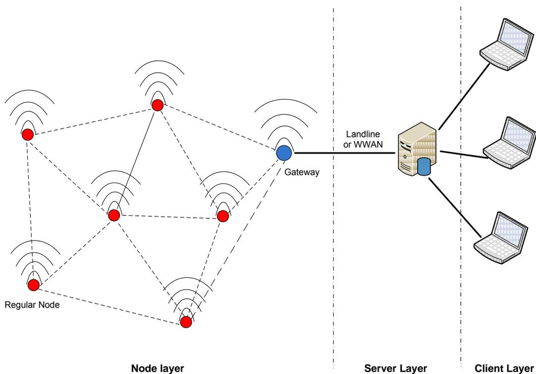
Figure 1 - Wireless Sensor Network Functional Architecture
