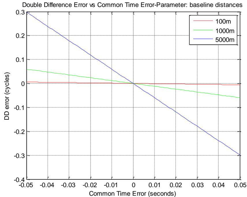
Figure 10 - Double difference in Cycles vs. Common Time Error for Multiple Baselines
