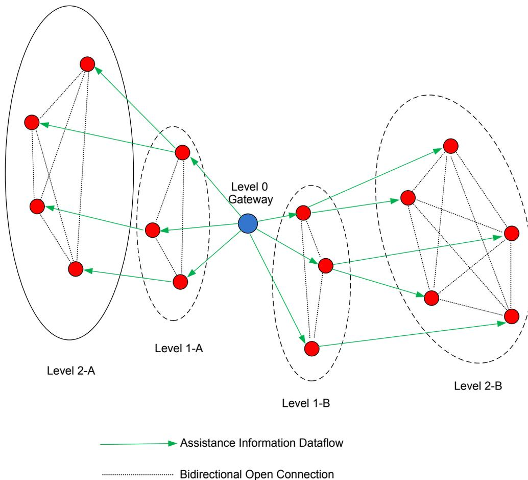
Figure 47 - WSN Centralized Architecture - Assistance Data Flow
