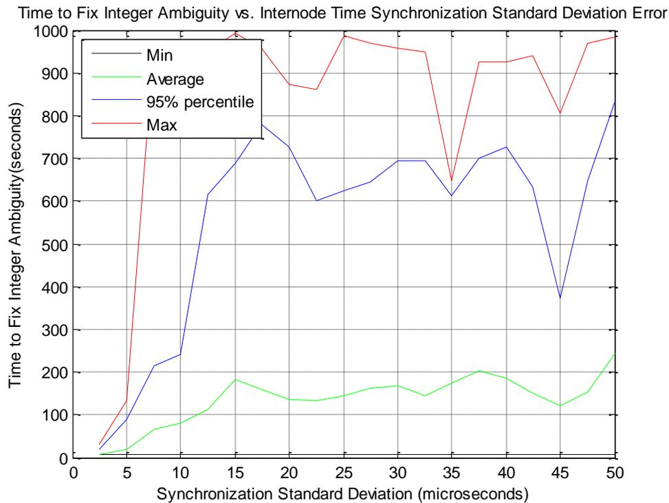
Figure 25 - Time to Fix Integer Ambiguity vs. Synchronization Error
