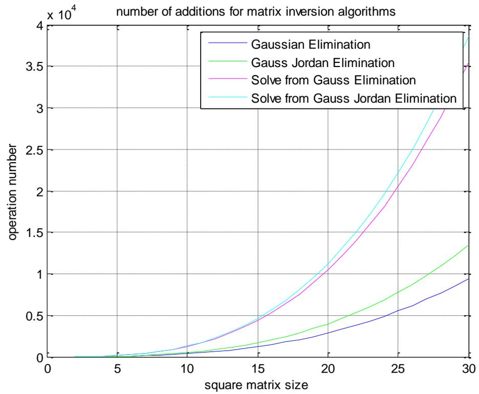
Figure 45 - Matrix Inversion Algorithms - Addition Count
