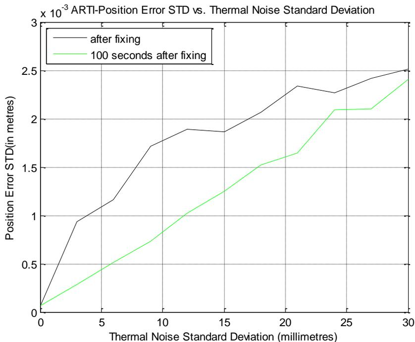
Figure 35 - ARTI - Position Error vs. Thermal Noise
