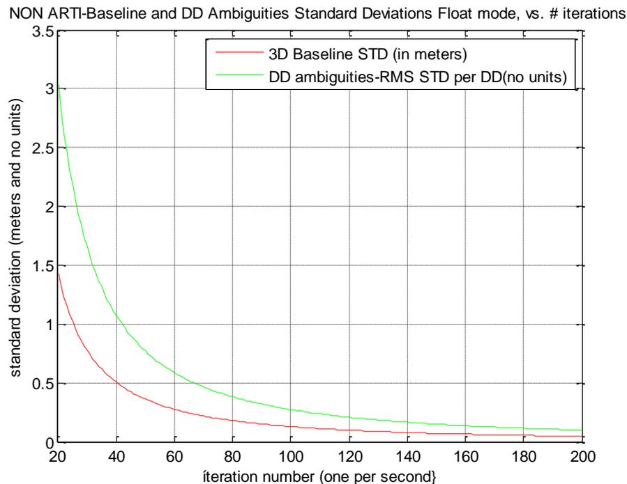
Figure 19 - Baseline and Ambiguities Standard Deviations in Float Mode vs. Number of seconds - 20 to 200 seconds range
