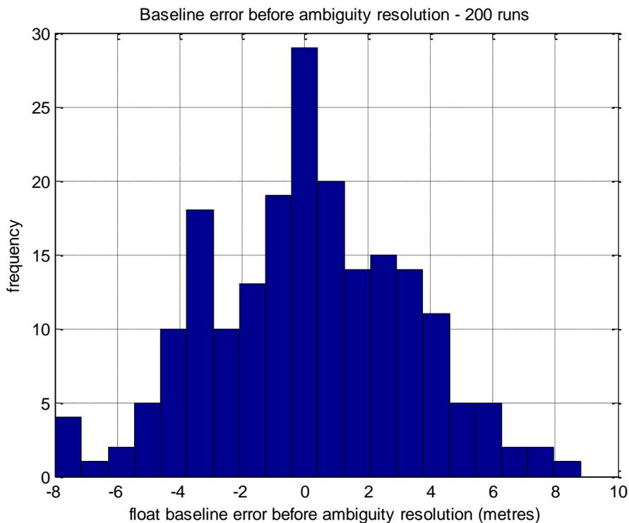
Figure 17 - Float Baseline Error before Ambiguity Resolution - Synchronization Error:  $2.5\mu\text{s}$
