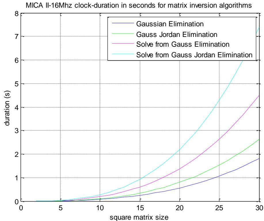
Figure 46 - Matrix Inversion algorithms - Execution Time on MICA II
