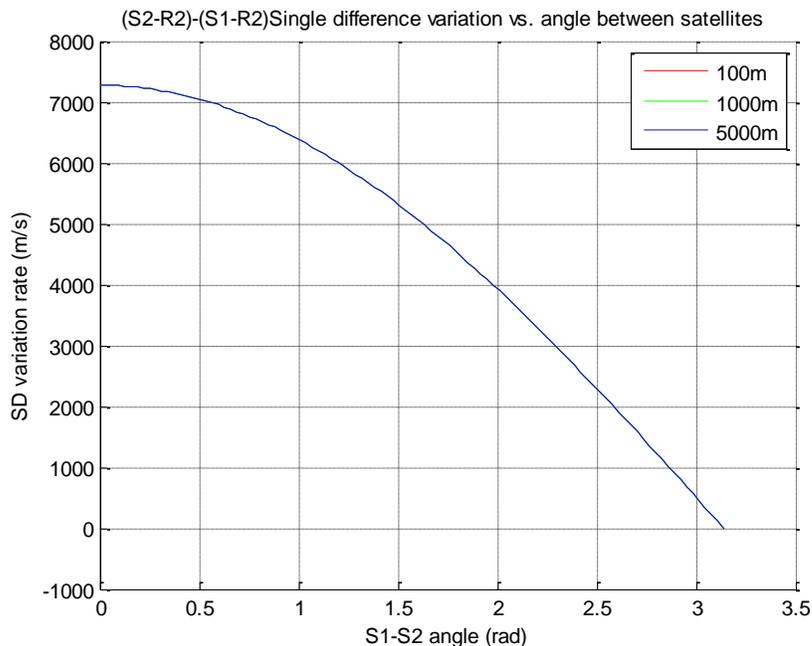
Figure 9 - Single Difference variation vs. angle between satellites
