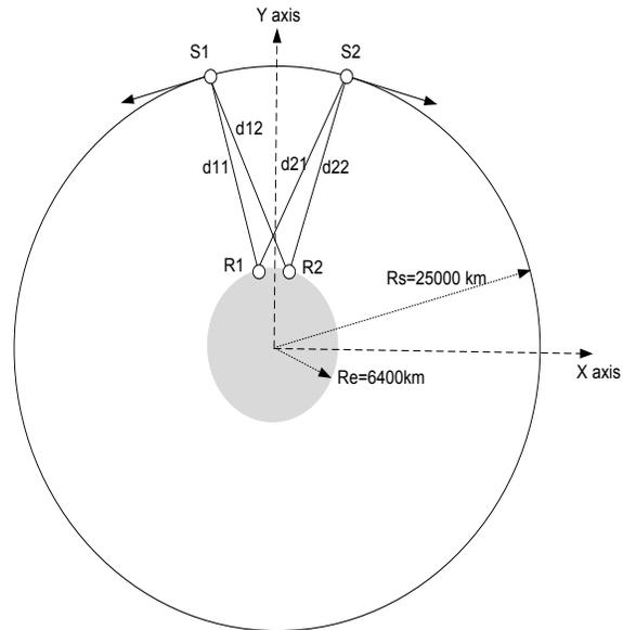
Figure 8 - Double Difference Sensitivity to Timing Errors - Simple Scenario
