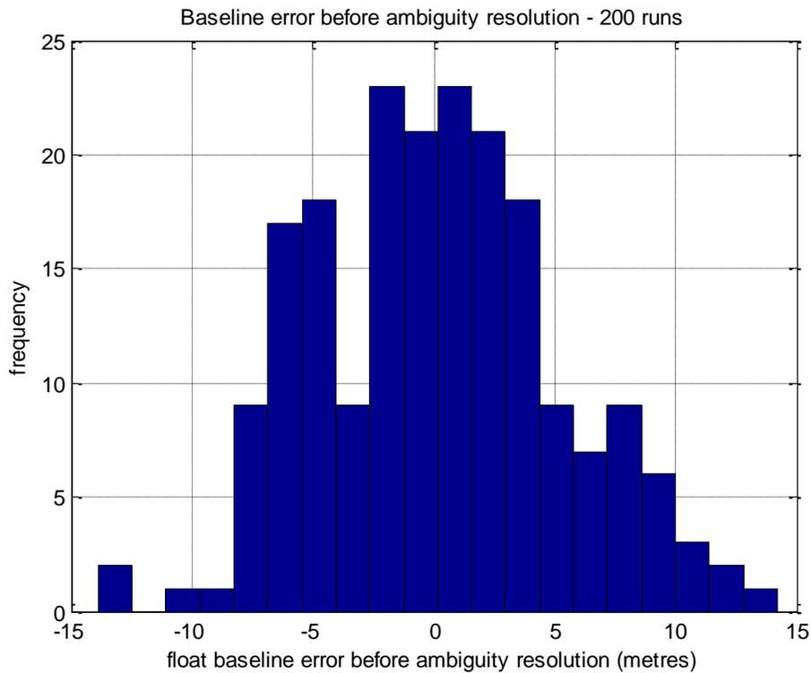
Figure 16 - Float baseline error before ambiguity resolution- no synchronization error
