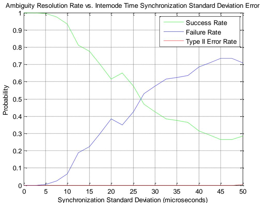
Figure 22 - Ambiguity Resolution Rate vs. Synchronization Error
