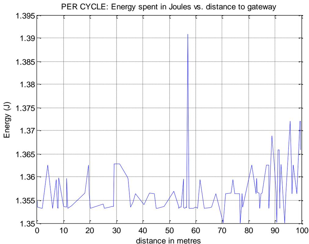
Figure 49 - Per node and per positioning cycle energy consumption vs. distance to gateway
