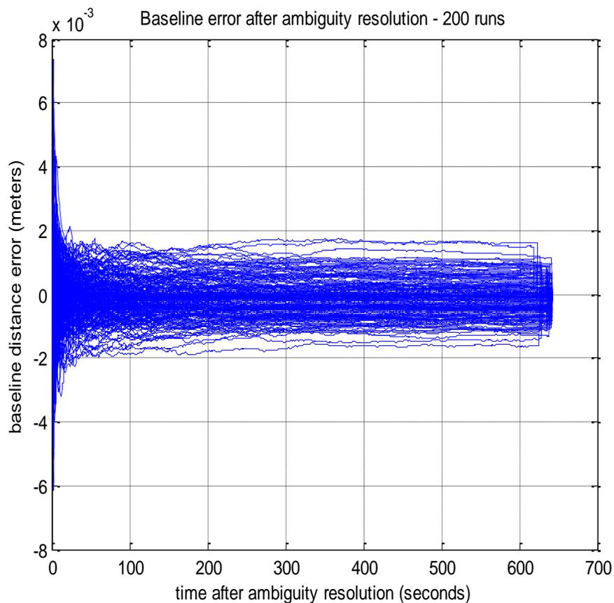
Figure 21 - Baseline Error after Ambiguity Fix - 2.5 us 1 sigma Synchronization Error
