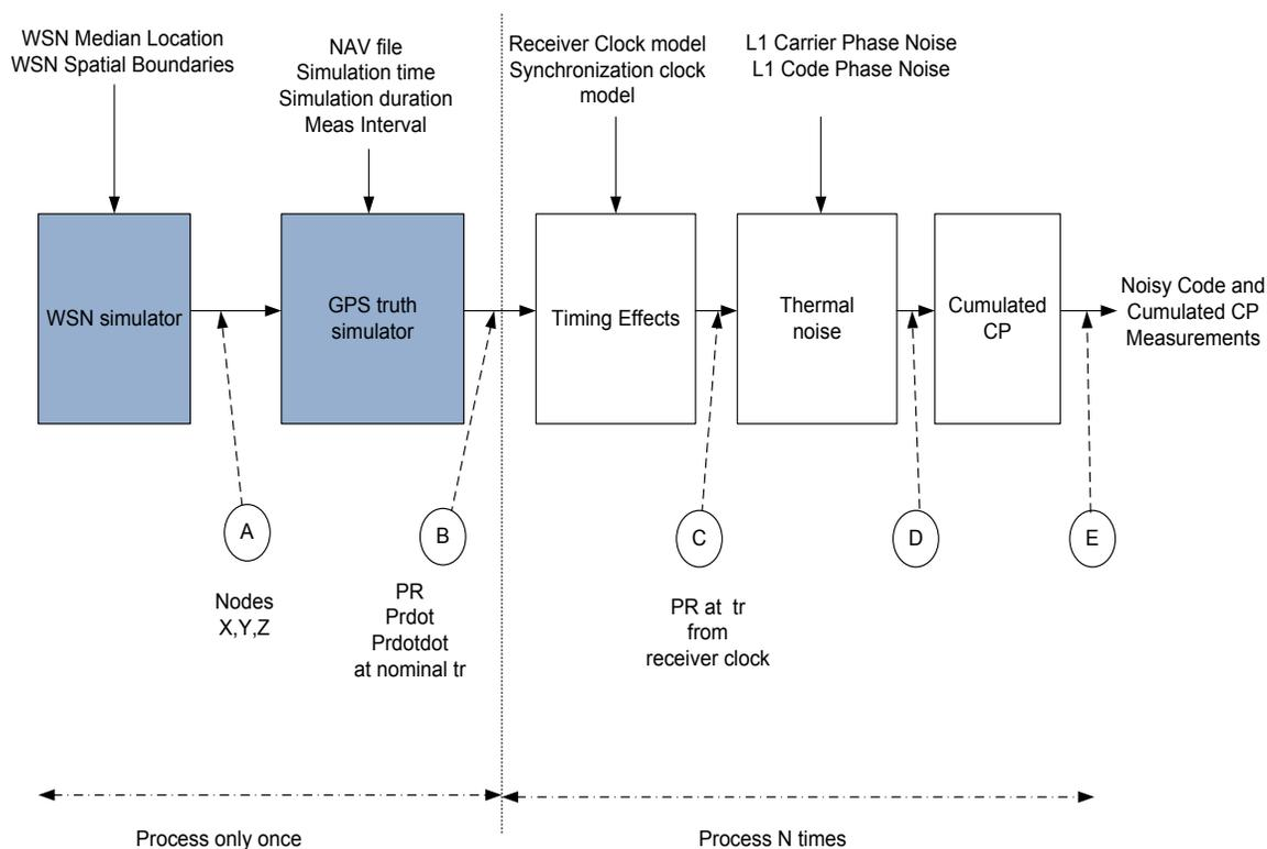
Figure 14 - Simulator Block Diagram
