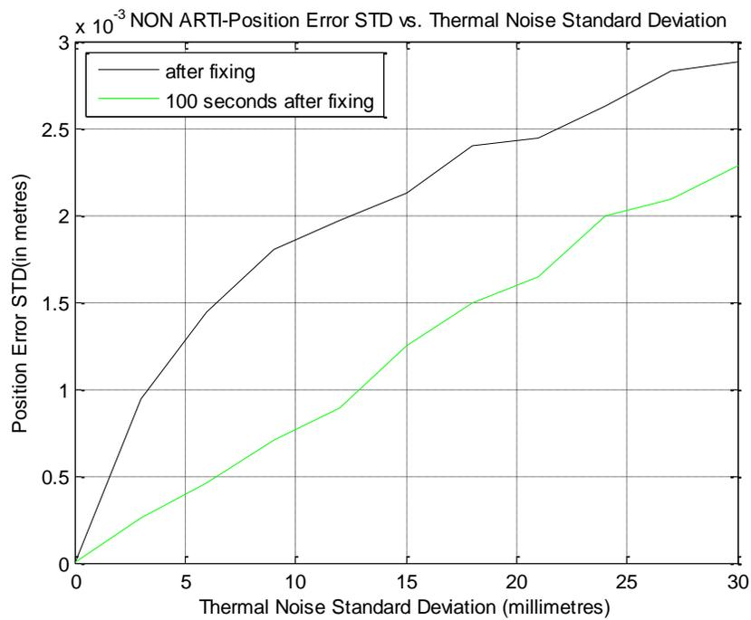
Figure 29 - NON ARTI - Position Error vs. Thermal Noise
