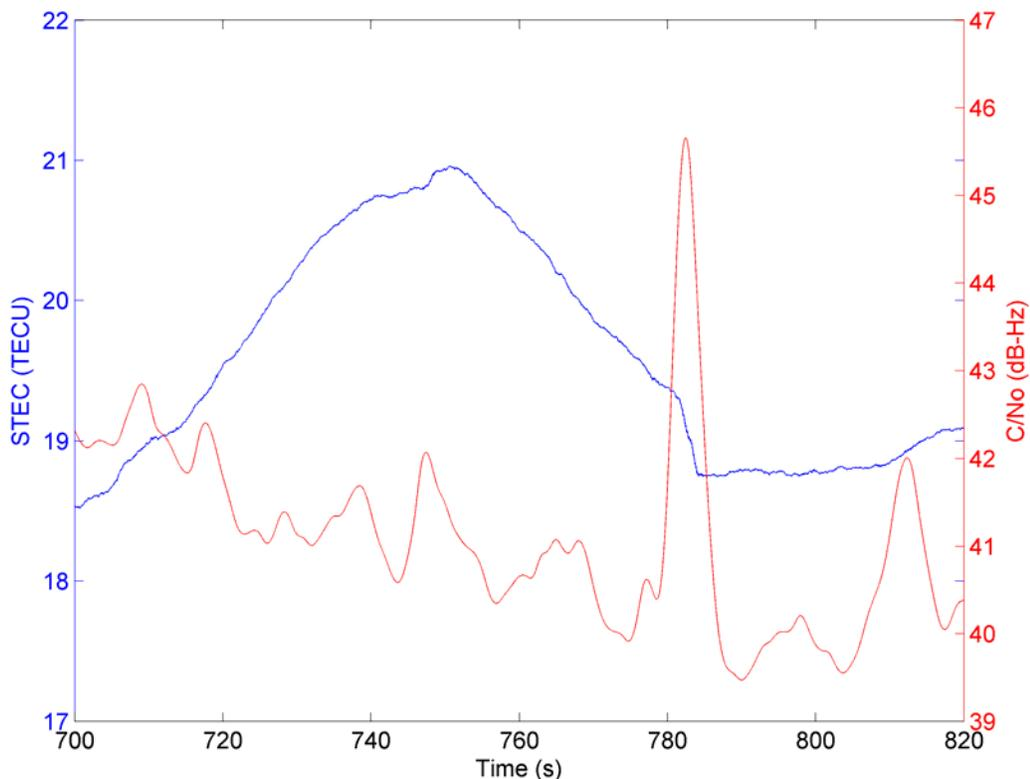
**Figure 6-16: Estimated TEC values and  $C/N_0$  during rapidly varying scintillation**
