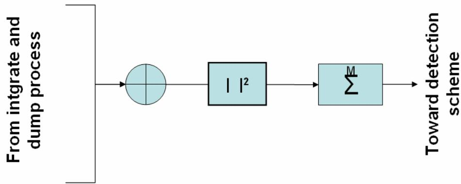
**Figure 3-8: Non-coherent summation of the L1 C/A plus the L2C over M post-correlation outputs**
