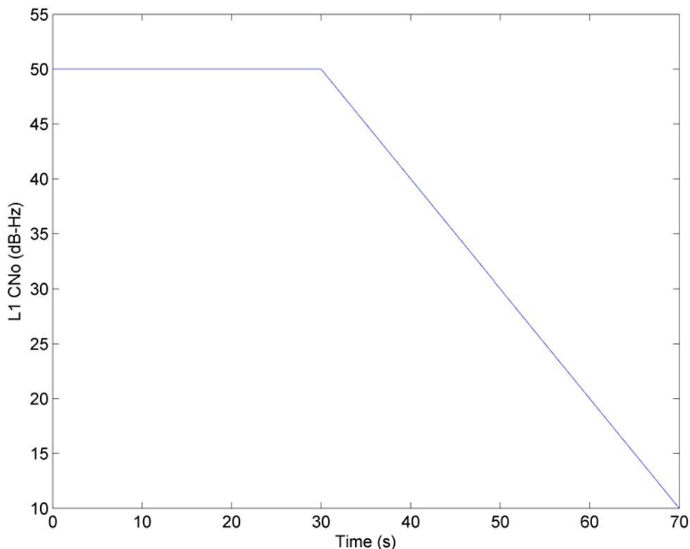
**Figure 6-6: L1 C/N<sub>0</sub> profile over time as estimated by an external commercial receiver**
