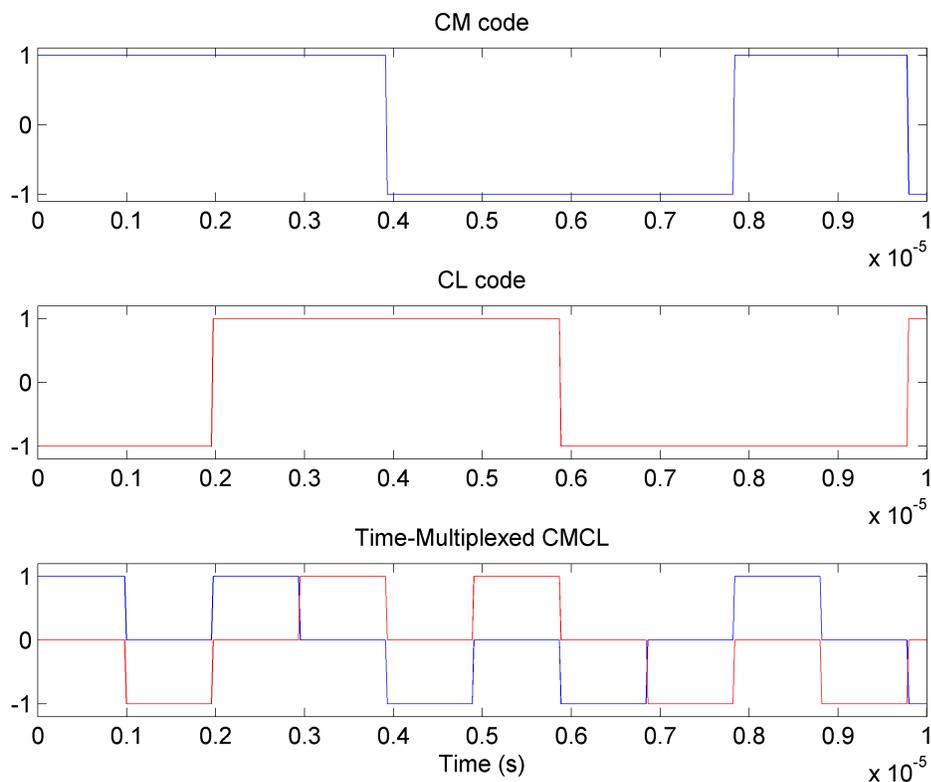
**Figure 2-5: CM and CL codes time-multiplexed representation**
