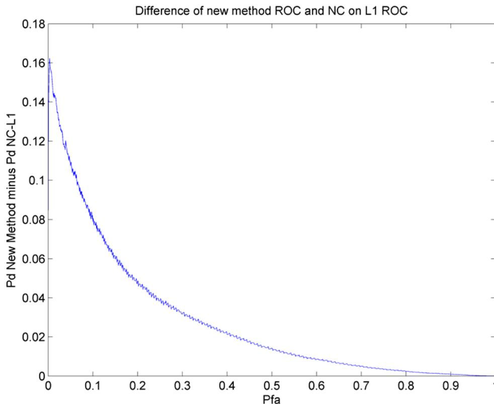
**Figure 4-18 : Difference between the  $\text{NCDiff}_{L1L2}$  ROC and the ROC obtained for a non-coherent acquisition on L1 only using simulated data**
