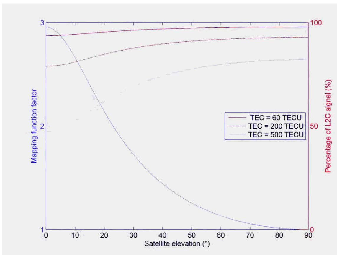
**Figure 2-11: Percentage of L2C signal left when locked on L1**
