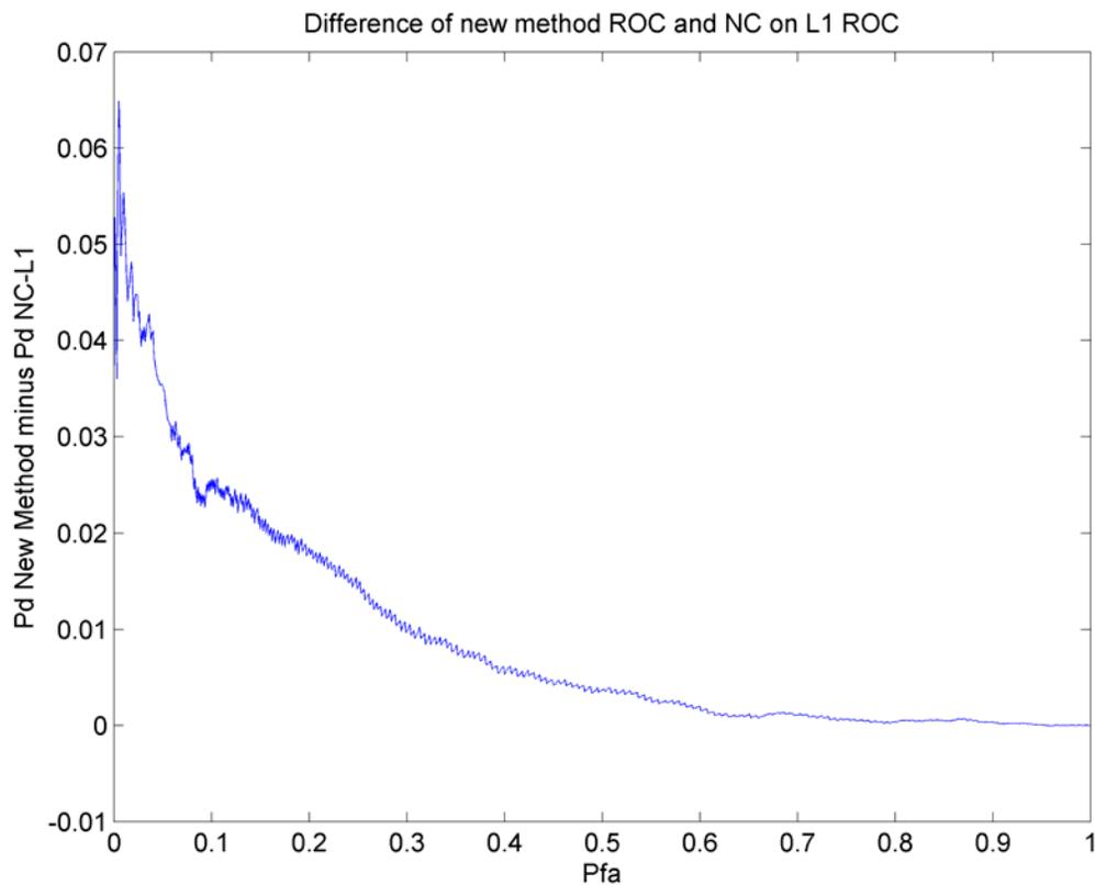
**Figure 4-20 : Difference between the  $NC_{L1L2}$  ROC and the ROC obtained for a non-coherent acquisition on L1 only using real data**
