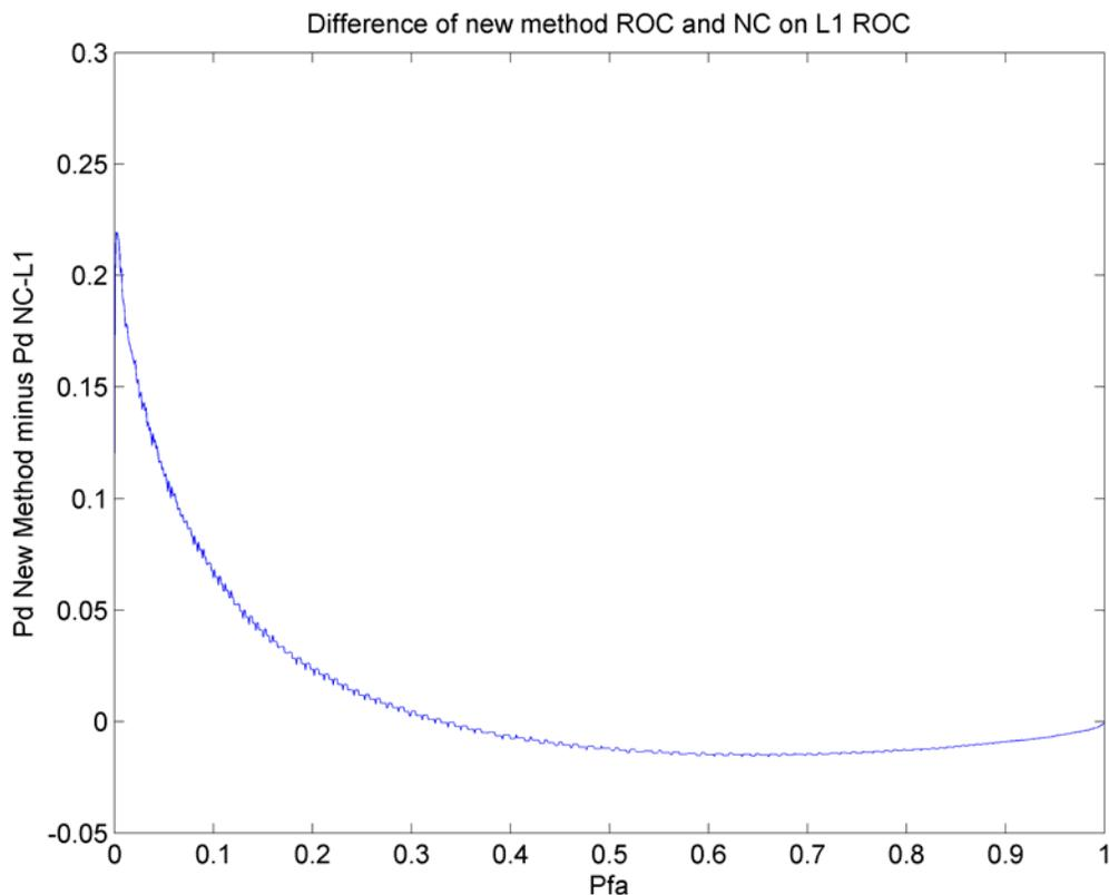
**Figure 4-16 : Difference between the  $\text{Diff}_{L1L2}$  ROC and the ROC obtained for a non-coherent acquisition on L1 only while limited the Doppler error to 100 Hz using simulated data**
