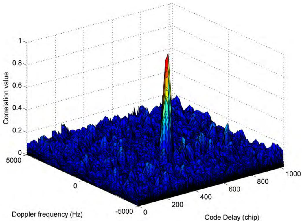
**Figure 2-7: Correlation of the GPS L1 C/A signal over the two-dimensional search space necessary for acquisition**
