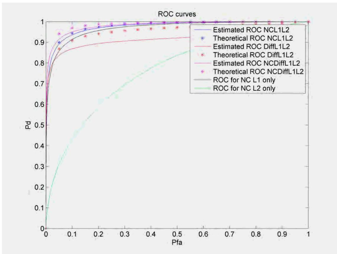
**Figure 4-27: ROC curves of the combined method obtained through the use of real data for a 2 ms coherent integration time**
