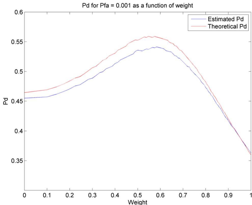
**Figure 4-10 : Theoretical probability of detection as a function of the weight applied on L2 for the NCDiff<sub>L1L2</sub> method**
