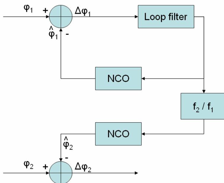
**Figure 5-1: L1 PLL feeding L2 tracking**
