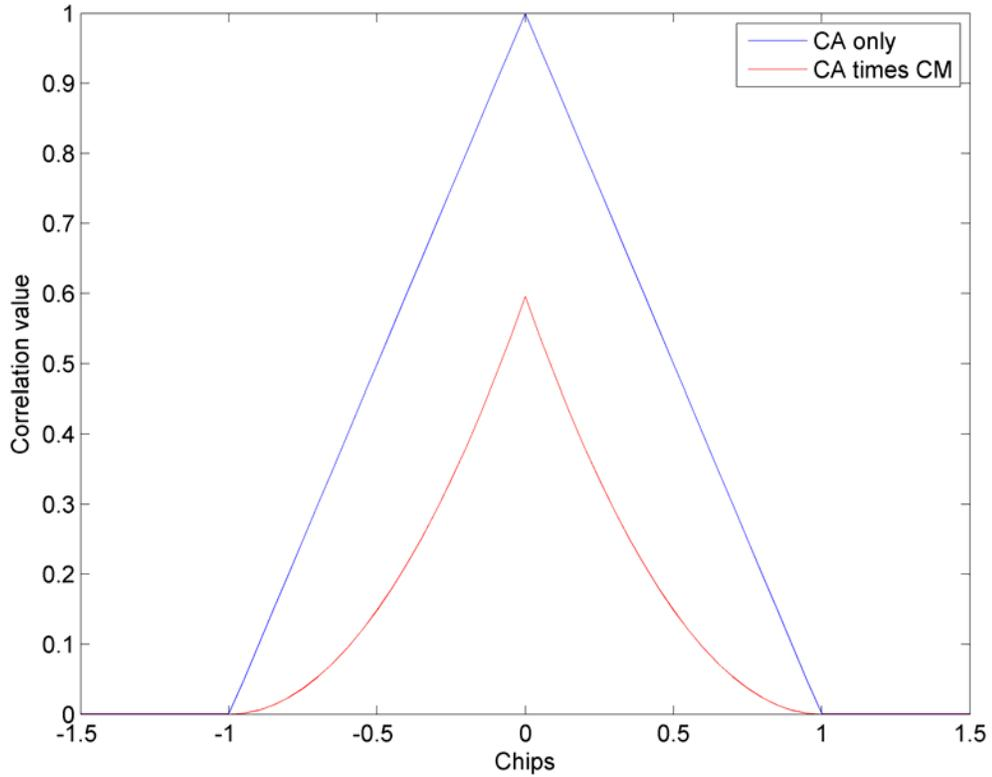
**Figure 3-7: Normalized correlation peaks of L1 C/A only compared to L1 C/A times L2 CM correlation peak. L1 C/A times L2C correlation is normalized by the correlation peak of L1 C/A**
