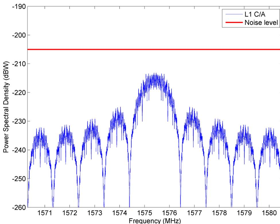
**Figure 2-4: Power Spectral Density of the GPS L1 C/A signal and typical thermal noise level**
