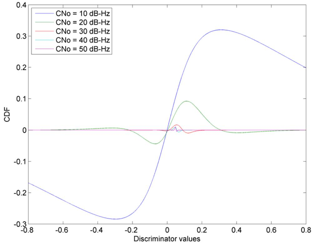
**Figure 5-19: difference between CDF of normalized early minus late envelope discriminator noise obtained through Monte-Carlo simulation and Gaussian noise approximation for different  $C/N_0$**
