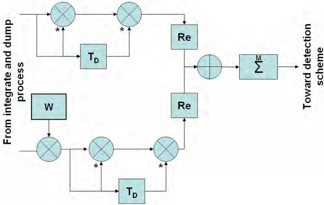
**Figure 3-4 : NCDiff<sub>L1L2</sub> represented as a block diagram**
