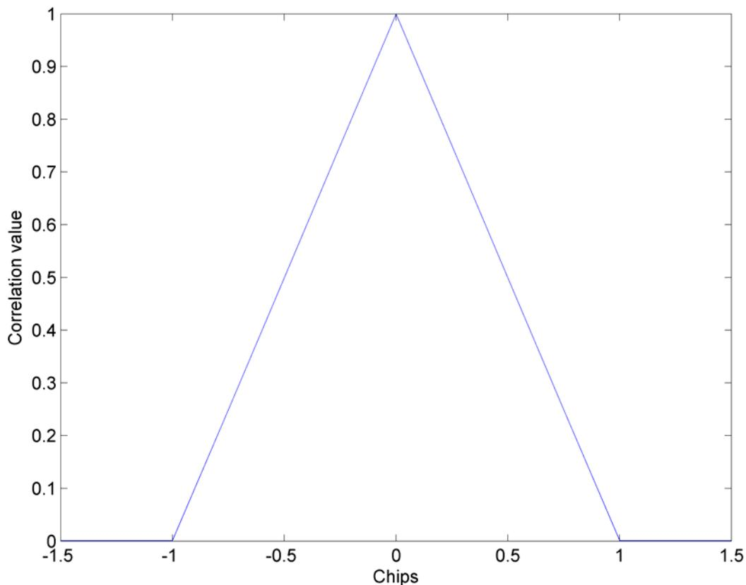
**Figure 2-2: Detailed view of the normalized correlation peak of GPS L1 C/A PRN 31 auto-correlation function**
