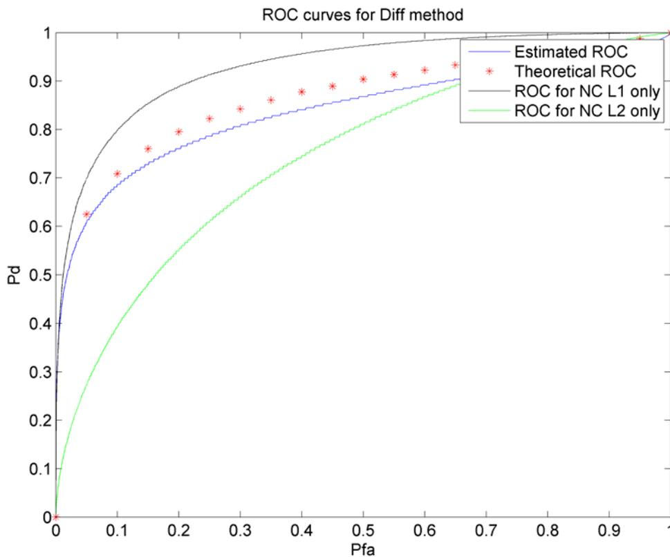
**Figure 4-13 : Theoretical and simulation estimated ROC curves for the Diff<sub>L1L2</sub> for residual Doppler values ranging from -333.33 Hz to 333.33 Hz**
