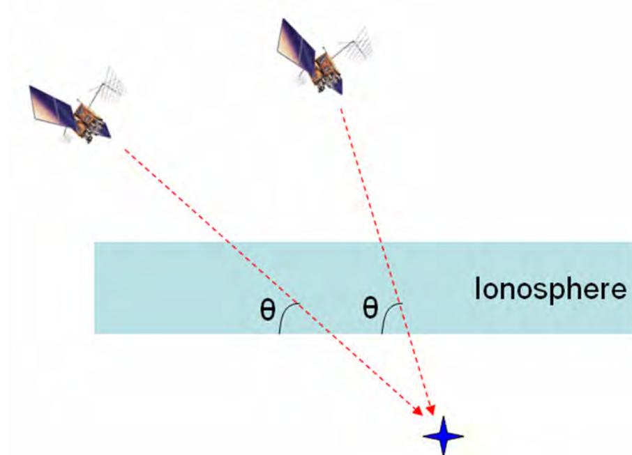
**Figure 5-4: Effect of satellite motion on signal path through an ionospheric layer**
