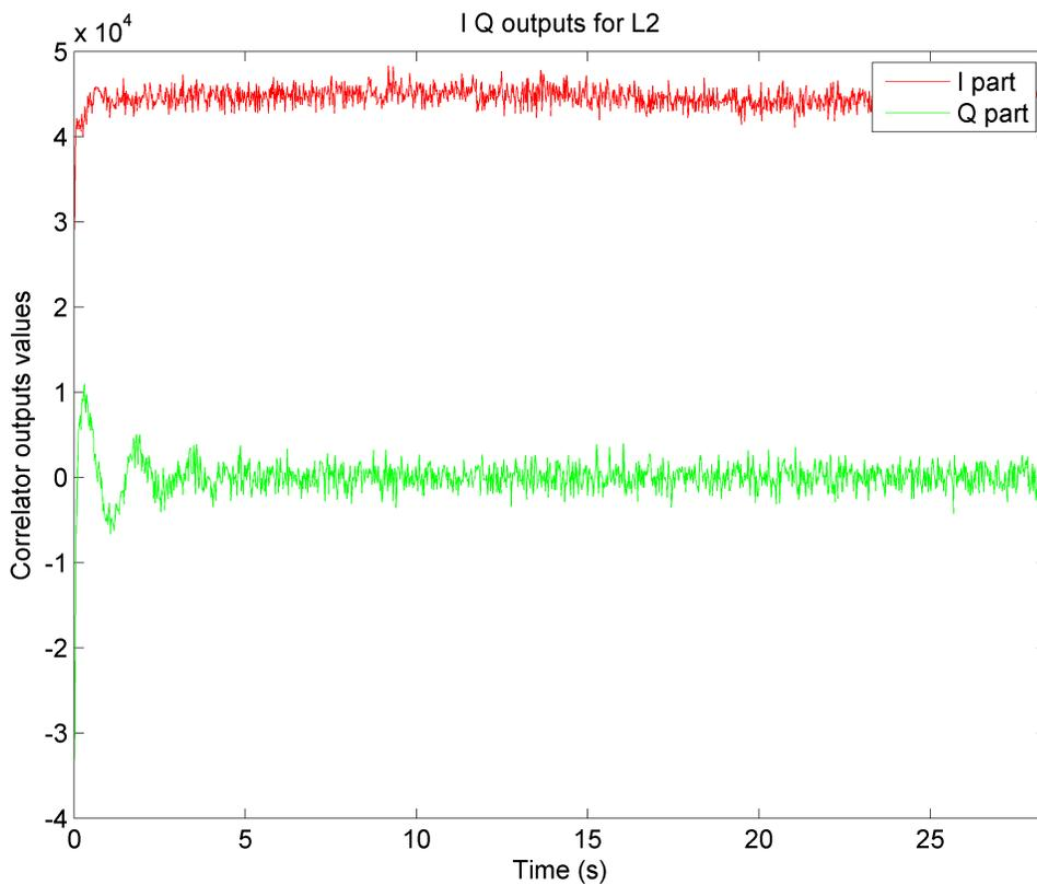
**Figure 5-8: L1 aiding L2, real and complex parts of L2 prompt correlator output**
