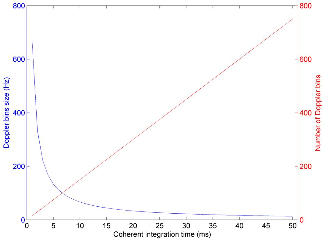
**Figure 2-10: Doppler bins size and number of Doppler bins needed to cover the search space as a function of the coherent integration time**
