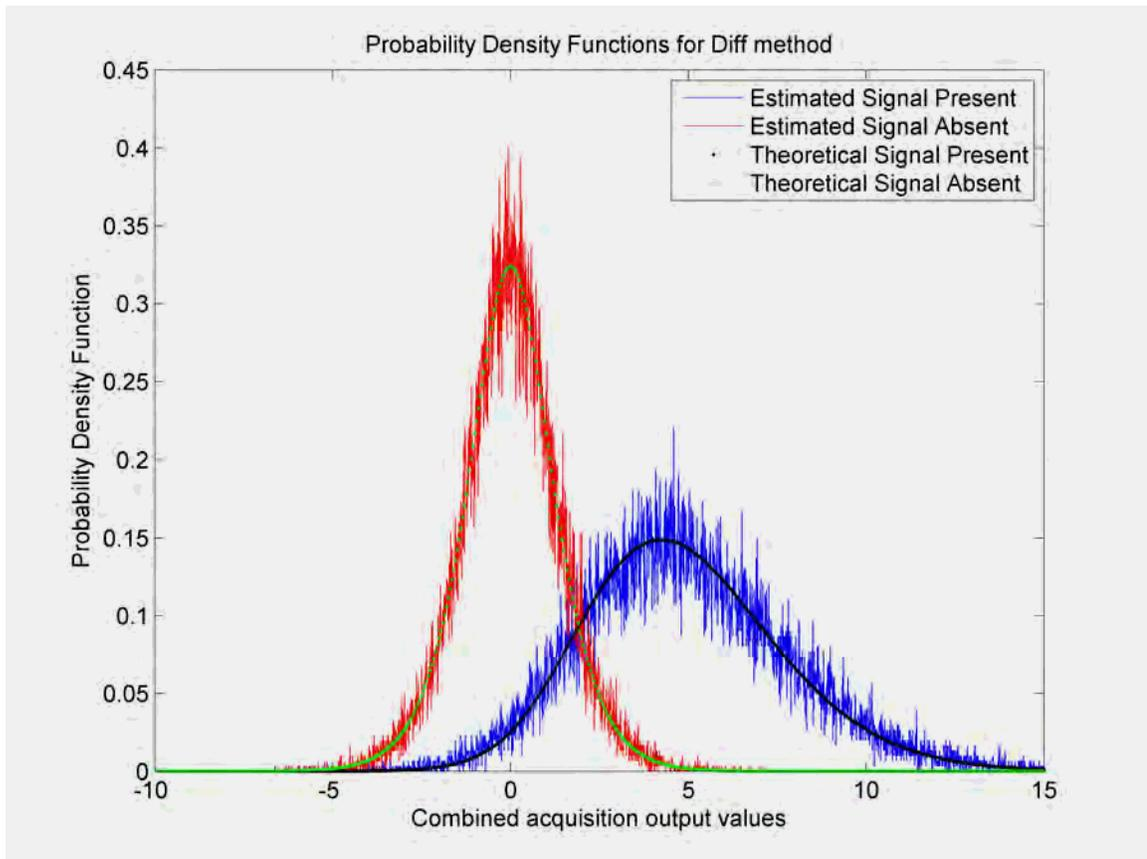
**Figure 4-5 : Probability density functions for the Diff<sub>L1L2</sub> method using real data**
