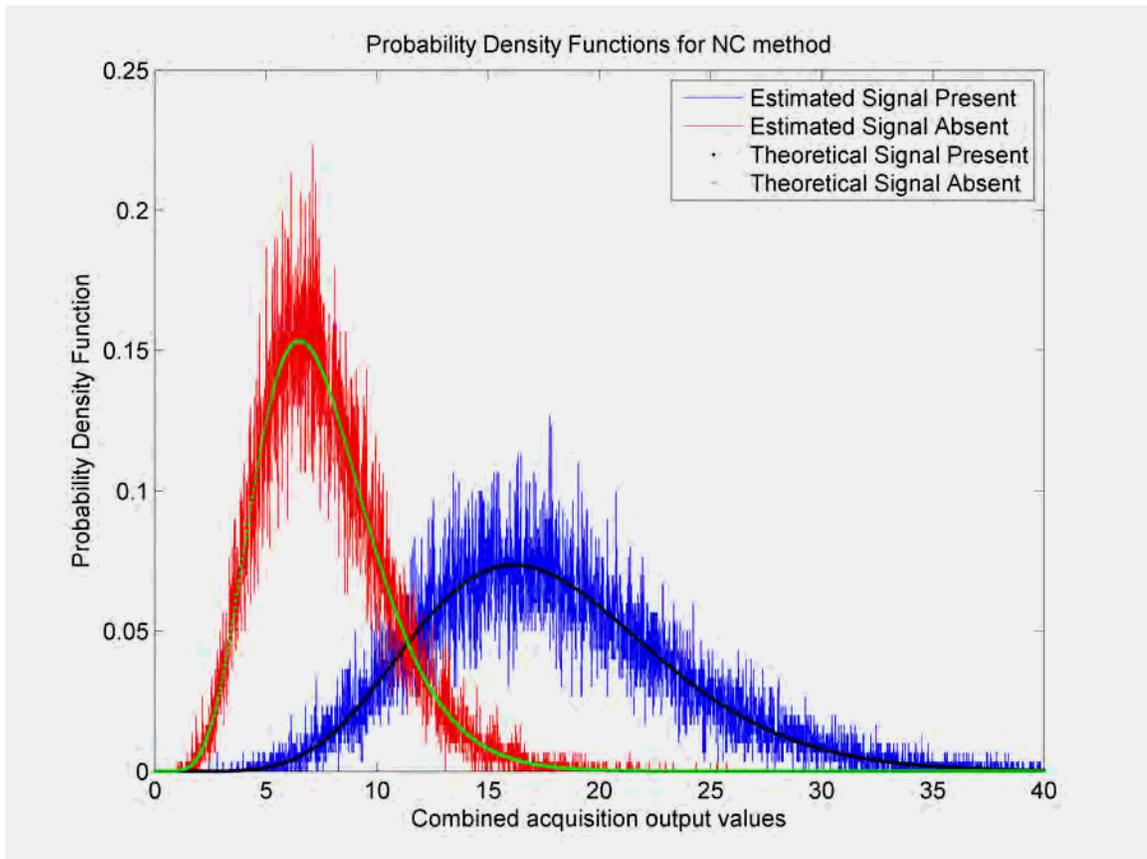
**Figure 4-3 : Probability density functions for the  $NC_{L1L2}$  method using real data**
