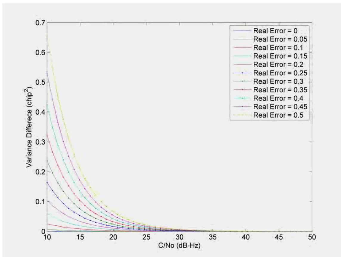
**Figure 5-14: Effect of assuming that the code error is zero when estimating the variance of the early minus late power discriminator**
