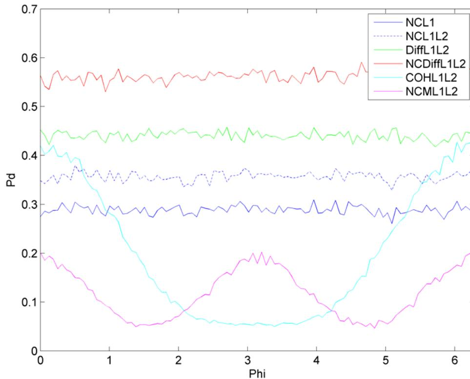
**Figure 3-15: Effect of the relative phase offset between L1 and L2 signals on the different acquisition methods**
