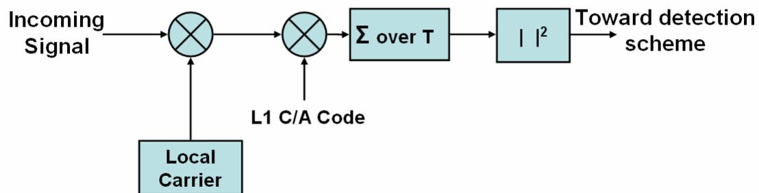
**Figure 2-8: Block diagram of a basic acquisition scheme**
