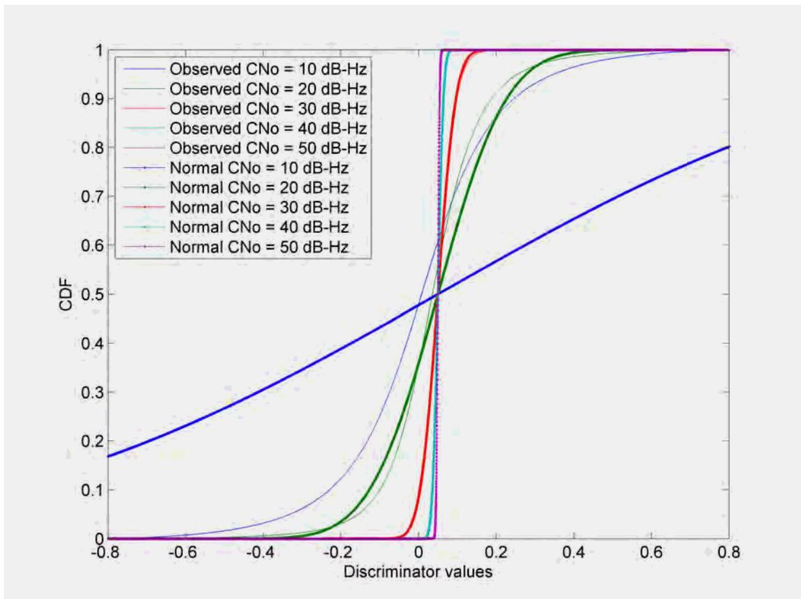
**Figure 5-18: CDF of normalized early minus late envelope discriminator noise obtained through Monte-Carlo simulation and Gaussian noise approximation for different  $C/N_0$  values**
