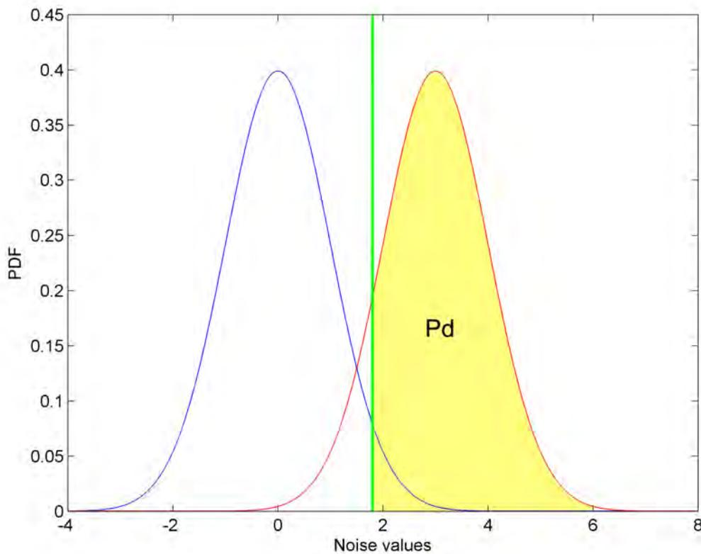
**Figure 3-9: Illustration of the probability of detection under Gaussian noise**
