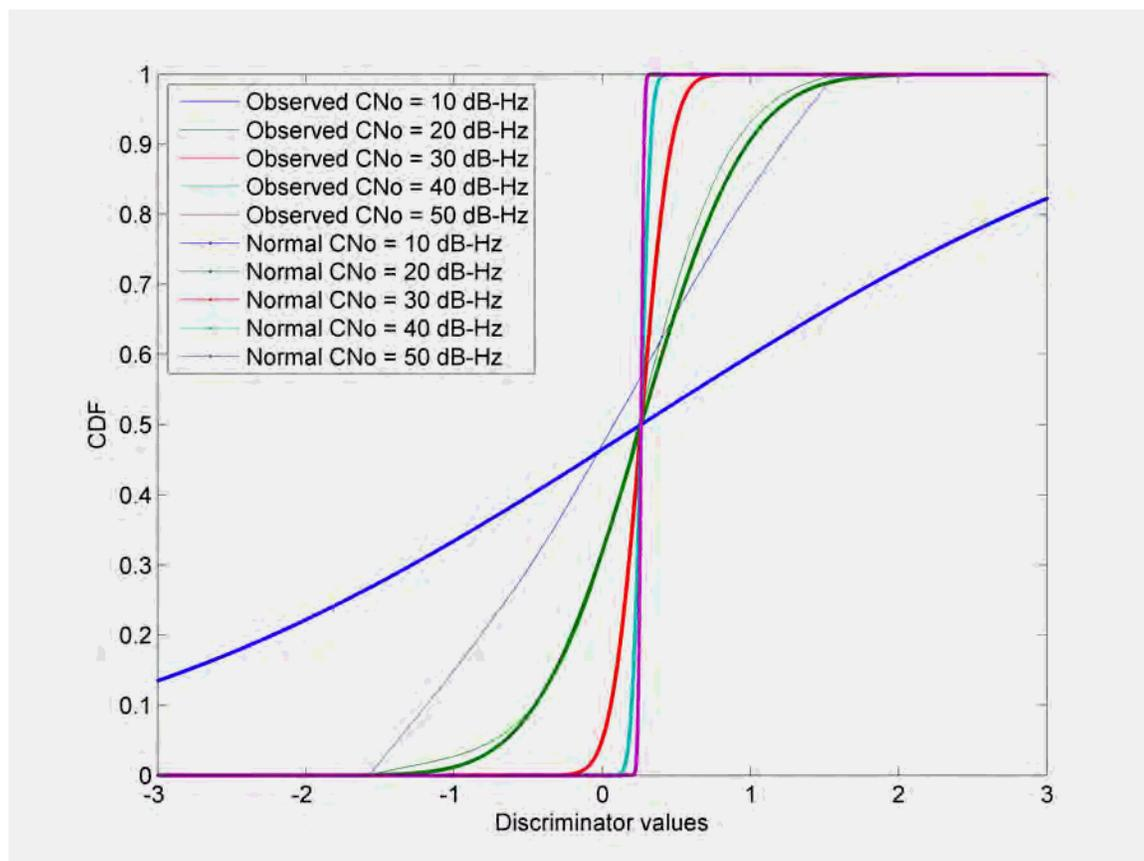
**Figure 5-12: CDF of *atan* noise obtained through Monte-Carlo simulation and Gaussian noise approximation for different  $C/N_0$  values**
