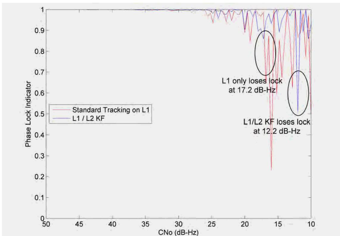
**Figure 6-9 : Phase lock indicator computed on the L1 C/A signal for the L1 only standard tracking module and the Kalman filter based tracking**
