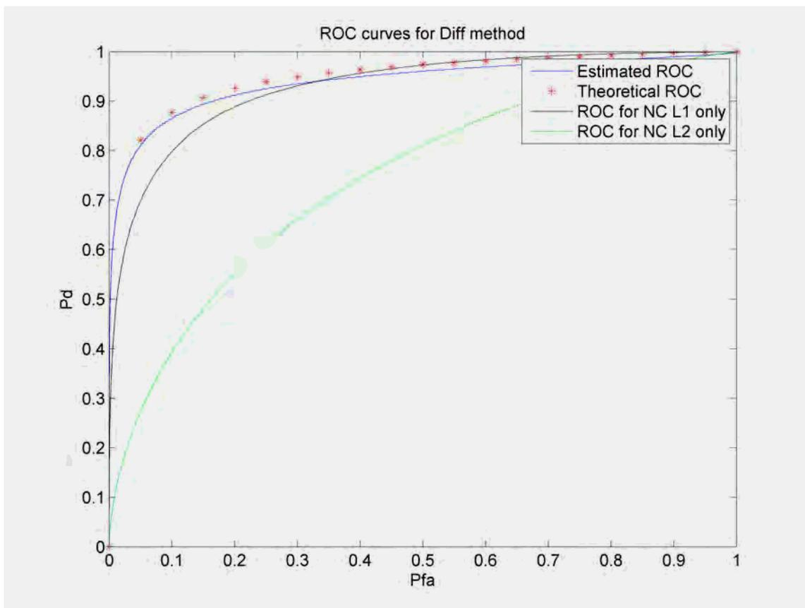
**Figure 4-15 : Theoretical and simulation estimated ROC curves for the Diff<sub>L1L2</sub> for residual Doppler values ranging from -100 Hz to 100 Hz**
