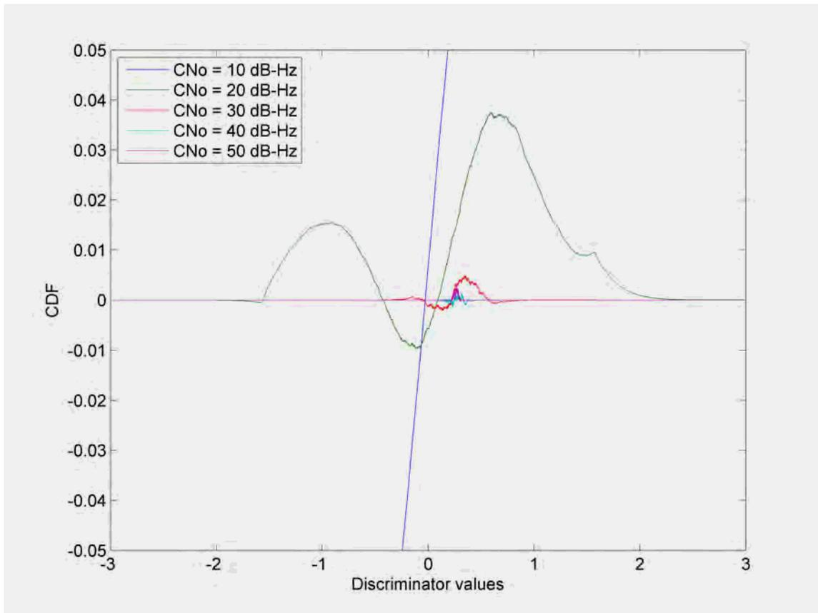
**Figure 5-13: Difference between CDF of *atan* noise obtained through Monte-Carlo simulation and Gaussian noise approximation for different  $C/N_0$  values**
