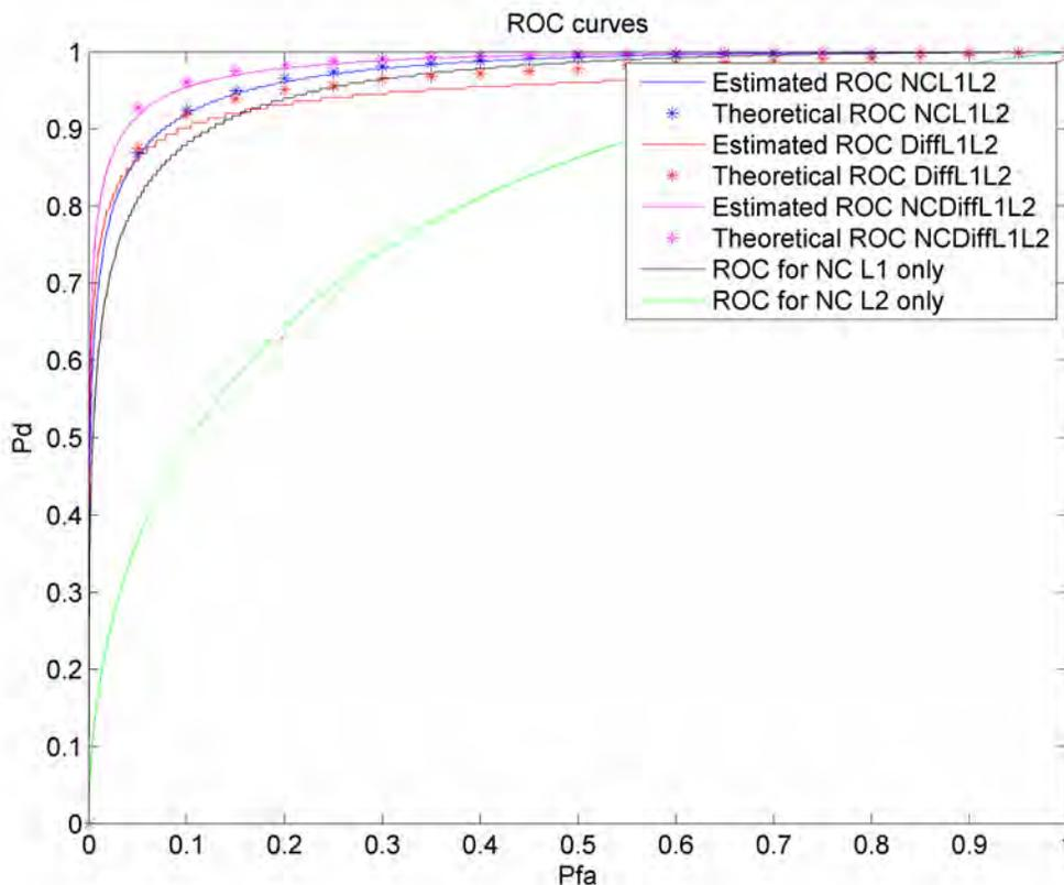
**Figure 4-25: ROC curves of the combined method obtained through simulation process for a 2 ms coherent integration time**
