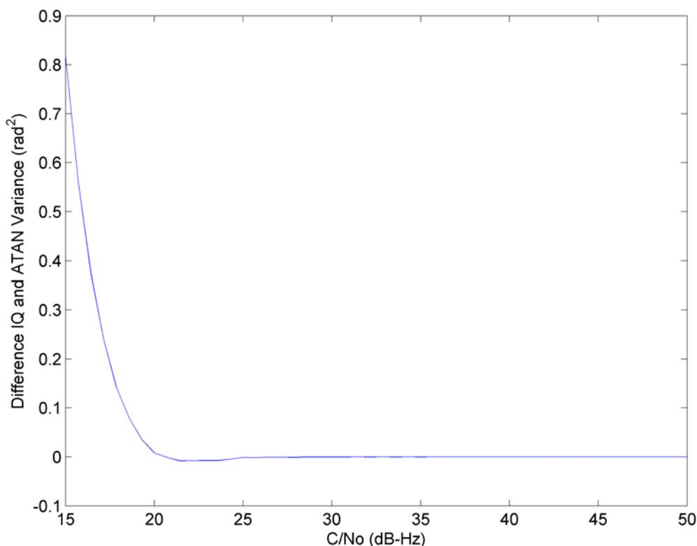
**Figure 5-11: Difference between the theoretical variance of  $I,Q$  and Monte-Carlo variance of  $atan$  discriminator as a function of  $C/N_0$**
