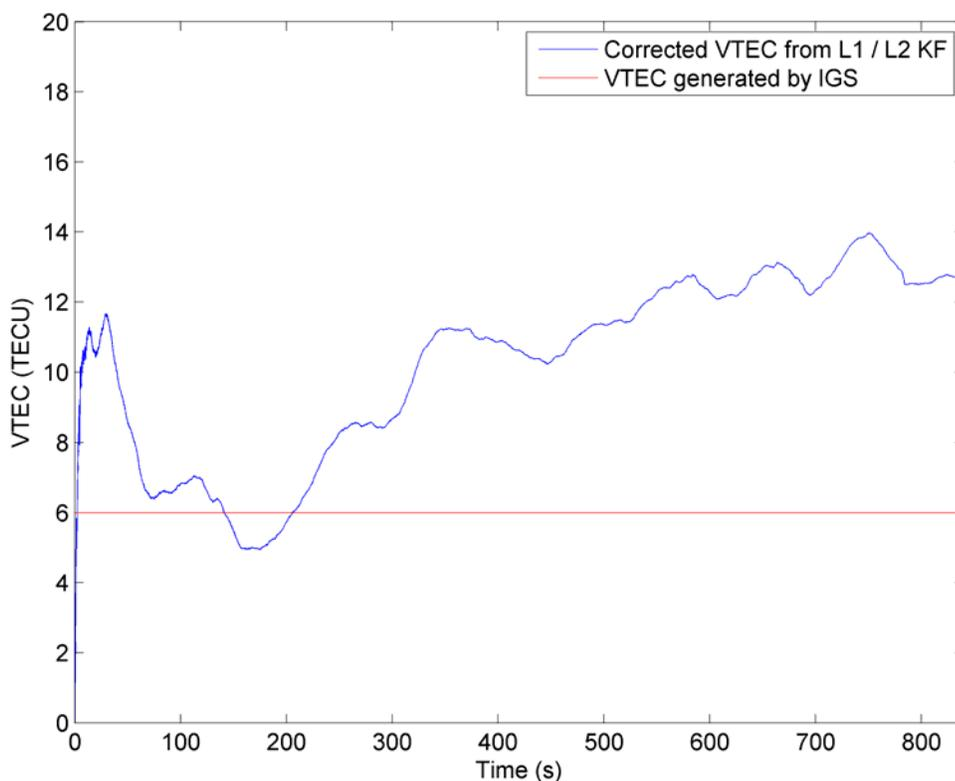
**Figure 6-14: Satellite and receiver biases free vertical TEC values derived from the Kalman filter based tracking and compared to the IGS generated values**
