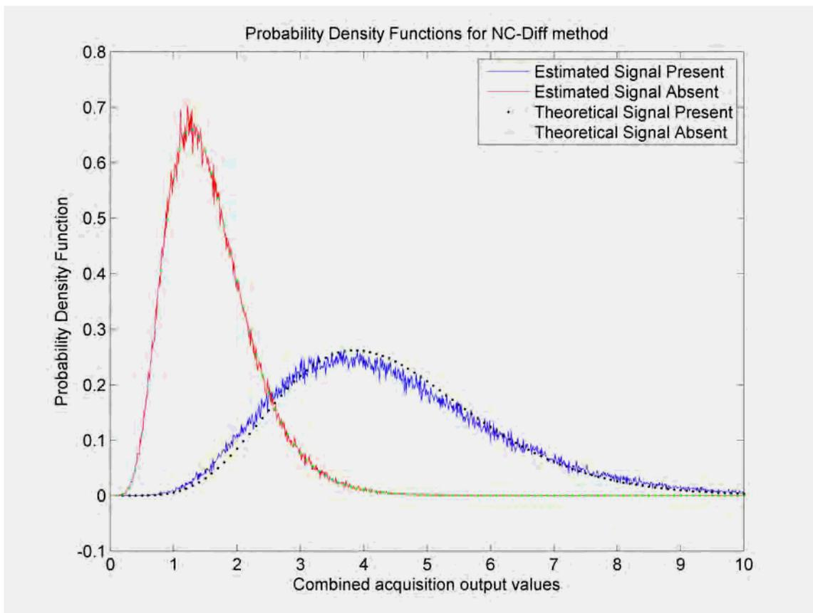
**Figure 4-6 : Probability density functions for the  $NCDiff_{L1L2}$  method using simulated data**
