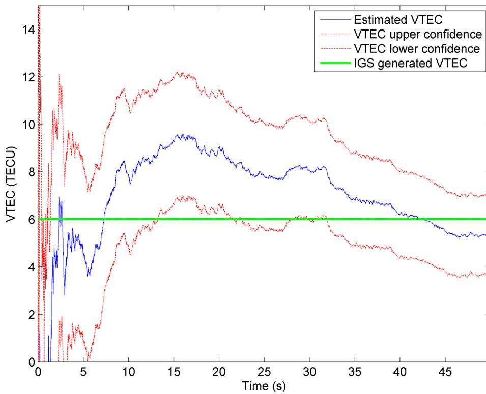
**Figure C-2: Estimated VTEC from the least-squares method using the Kalman filter based combined tracking outputs and IGS generated VTEC as well as the  $1\sigma$  confidence**
