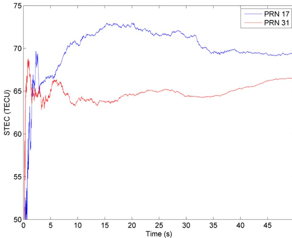
**Figure C-1: TEC encountered on the signal path for PRN 17 and PRN 31 as computed by the Kalman filter based combined tracking**
