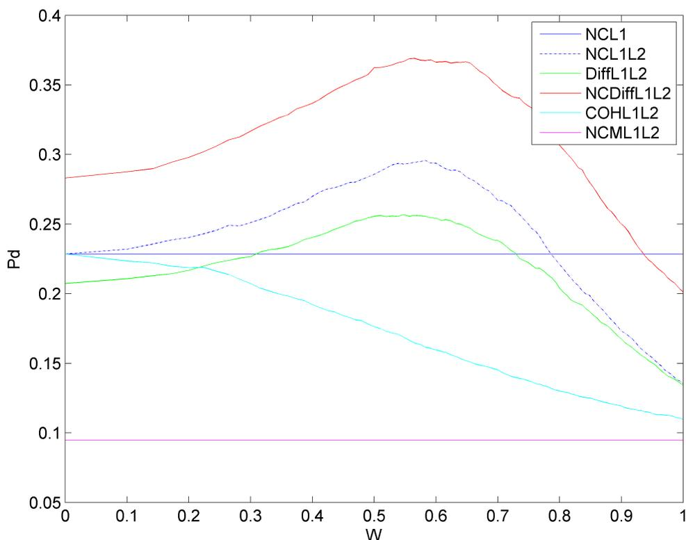
**Figure 3-11: Probability of detection obtained by applying different weights to the L2 post-correlation outputs for  $P_{fa}=1e-3$**
