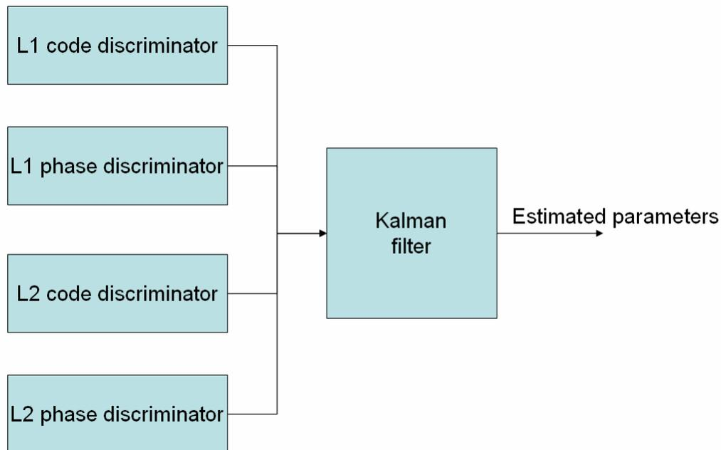
**Figure 5-9: Principle of proposed Kalman filter based tracking method**
