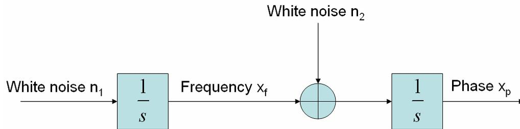
**Figure 5-20: General two state model describing the clock errors (Brown & Hwang 1992)**
