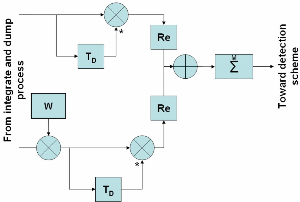
**Figure 3-3 : Diff<sub>L1L2</sub> represented as a block diagram**
