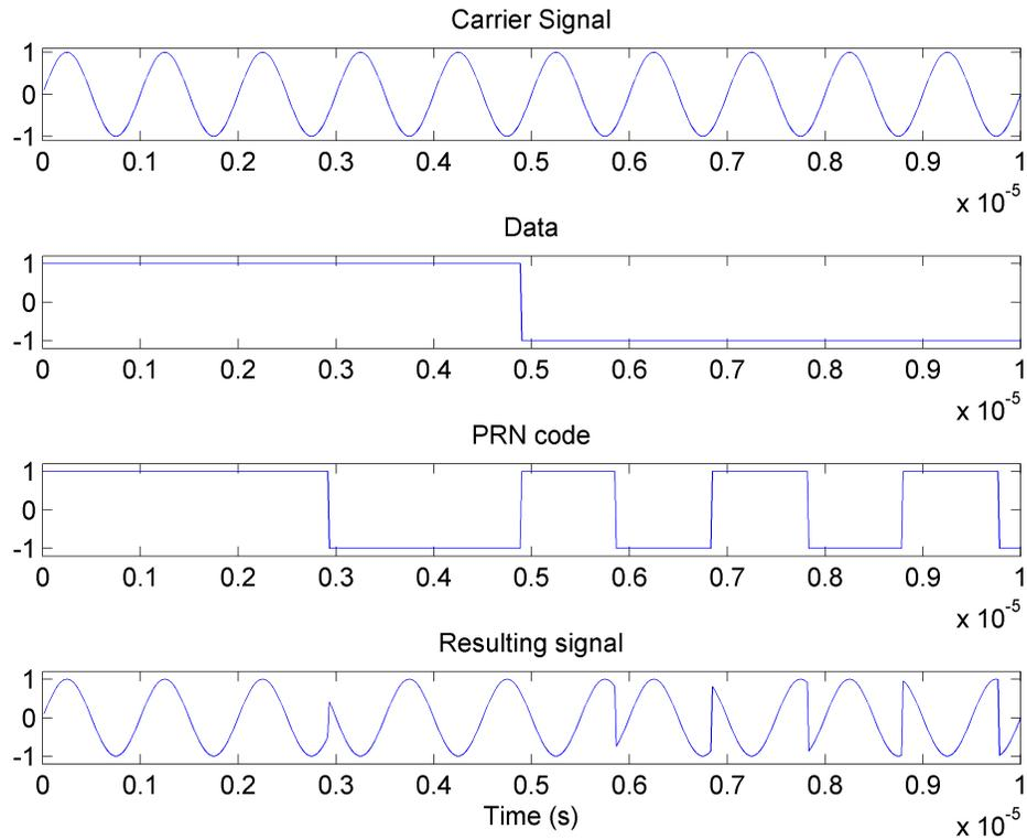
**Figure 2-3: Application of the DSSS process to the GPS signal.**
