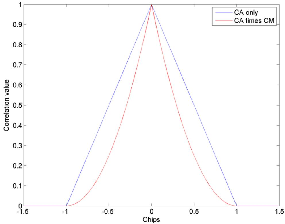
**Figure 3-6: Normalized correlation peaks of L1 C/A only and L1 C/A times L2 CM codes**
