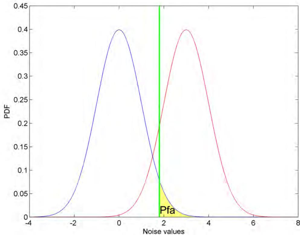
**Figure 3-10: Illustration of the probability of false alarm under Gaussian noise**
