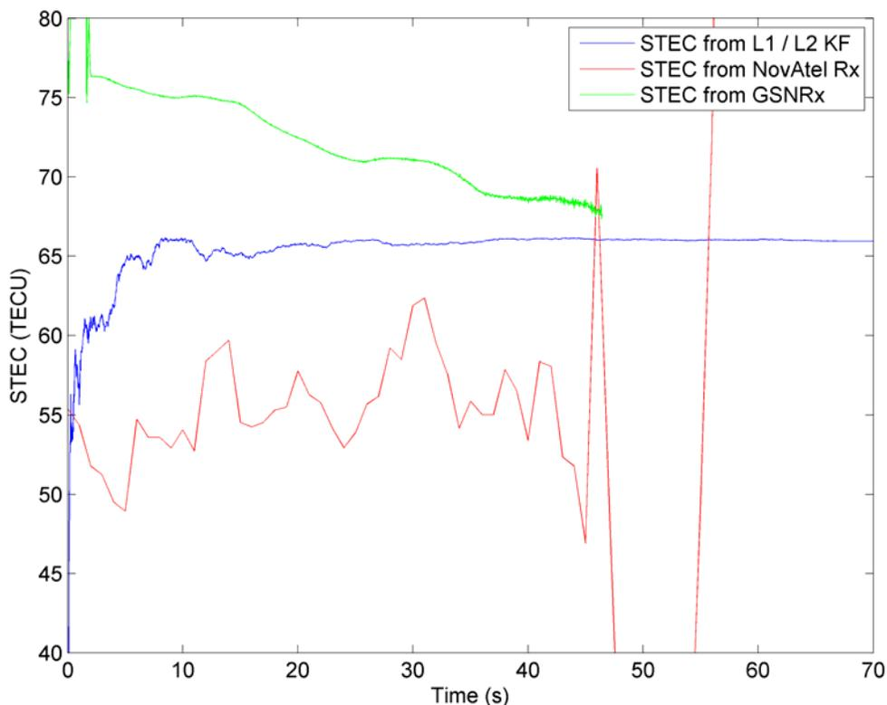
**Figure 6-11 : Estimated TEC values encountered on the signal path as a function of time**
