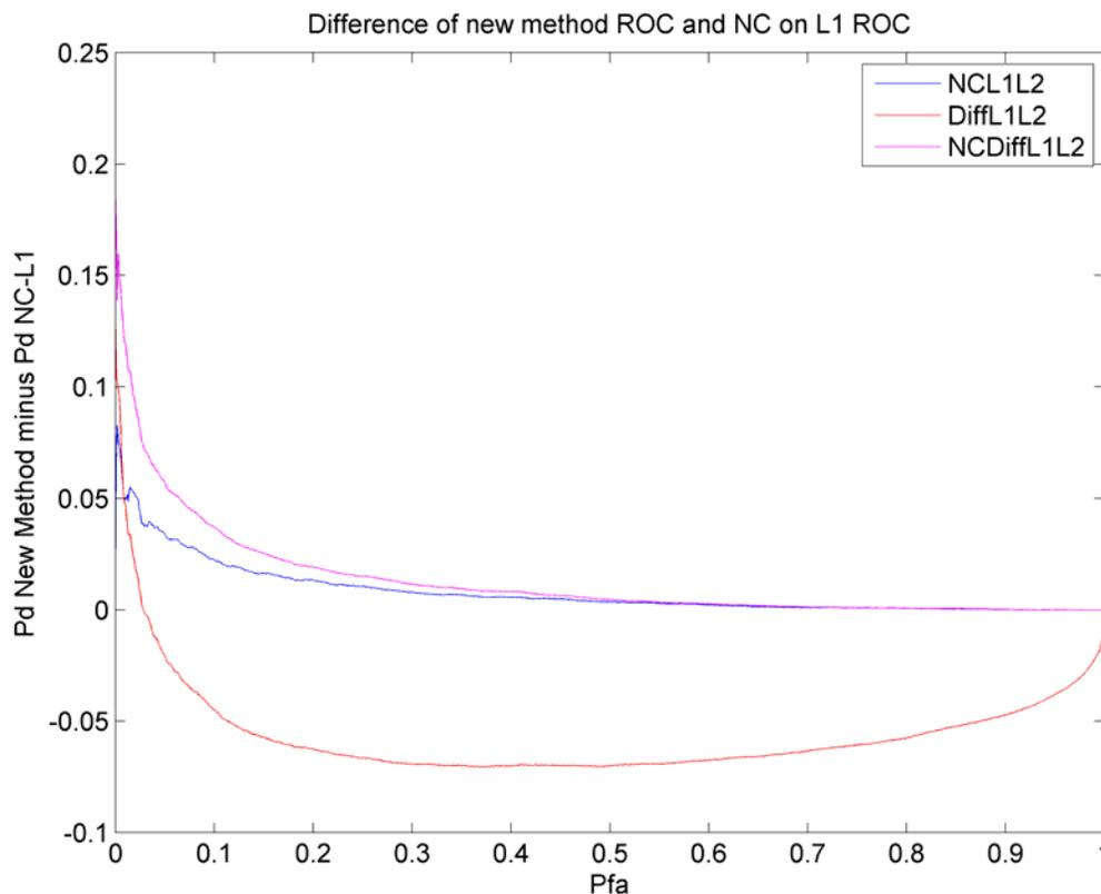
**Figure 4-28: Difference between the new combined method ROC curves with the non-coherent acquisition on L1 ROC curve**
