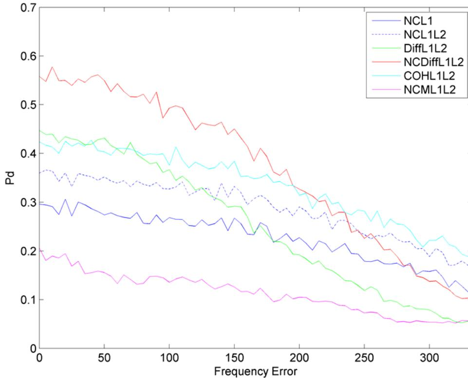
**Figure 3-14: Effect of residual Doppler errors on the different acquisition methods**
