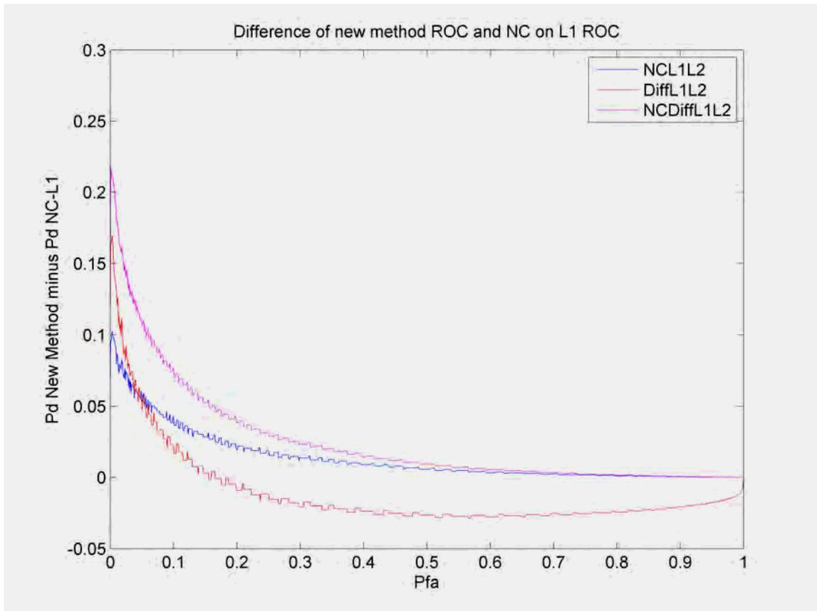
**Figure 4-26: Difference between the new combined method ROC curves with the non-coherent acquisition on L1 ROC curve**
