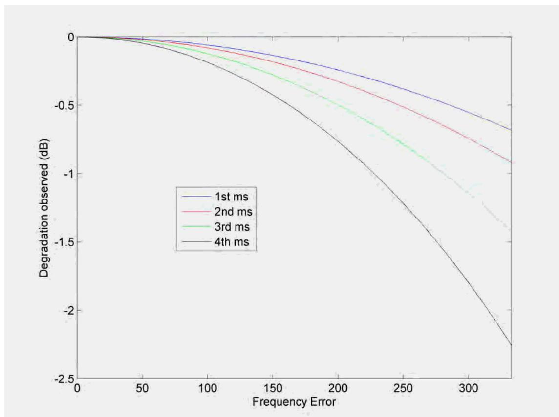
**Figure 3-13: Degradation observed on the coherent summation of L1 and L2 post-correlation outputs for each millisecond as a function of L1 Doppler residual**
