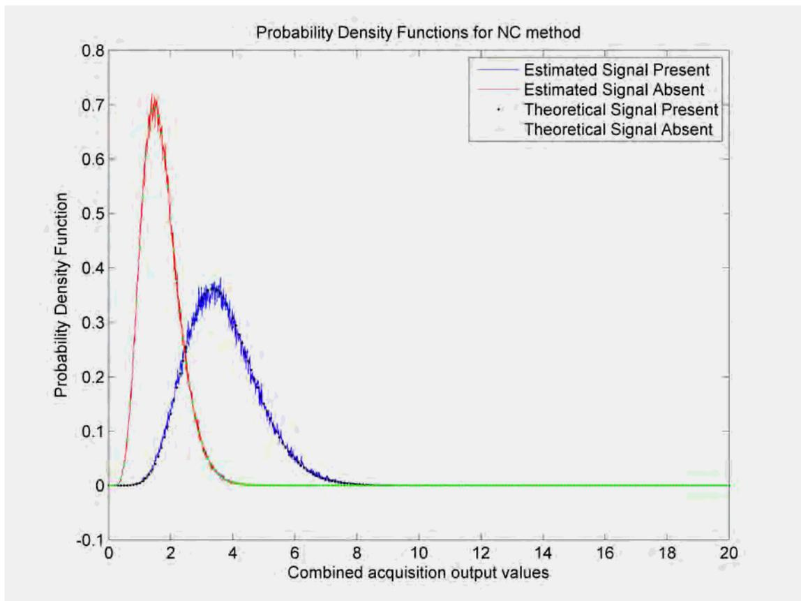
**Figure 4-2 : Probability density functions for the  $NC_{L1L2}$  method using simulated data**
