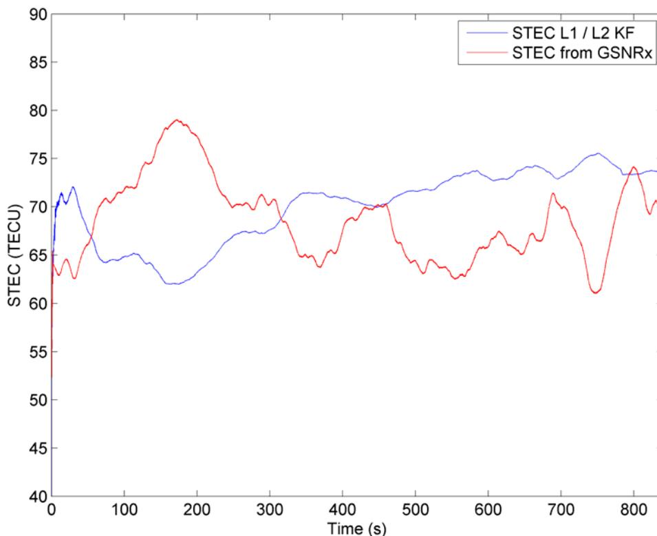
**Figure 6-13 : TEC values output by the Kalman filter tracking and GSNRx™ smooth pseudorange during scintillation**
