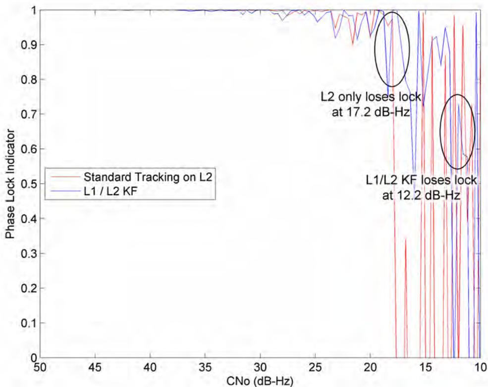
**Figure 6-10 : Phase lock indicator computed on the L2 CM + CL signal for the L2 only standard tracking module and the Kalman filter based tracking**
