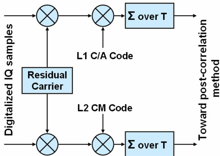
**Figure 3-1: Doppler removal, code removal and integrate and dump process performed prior to the proposed acquisition methods**
