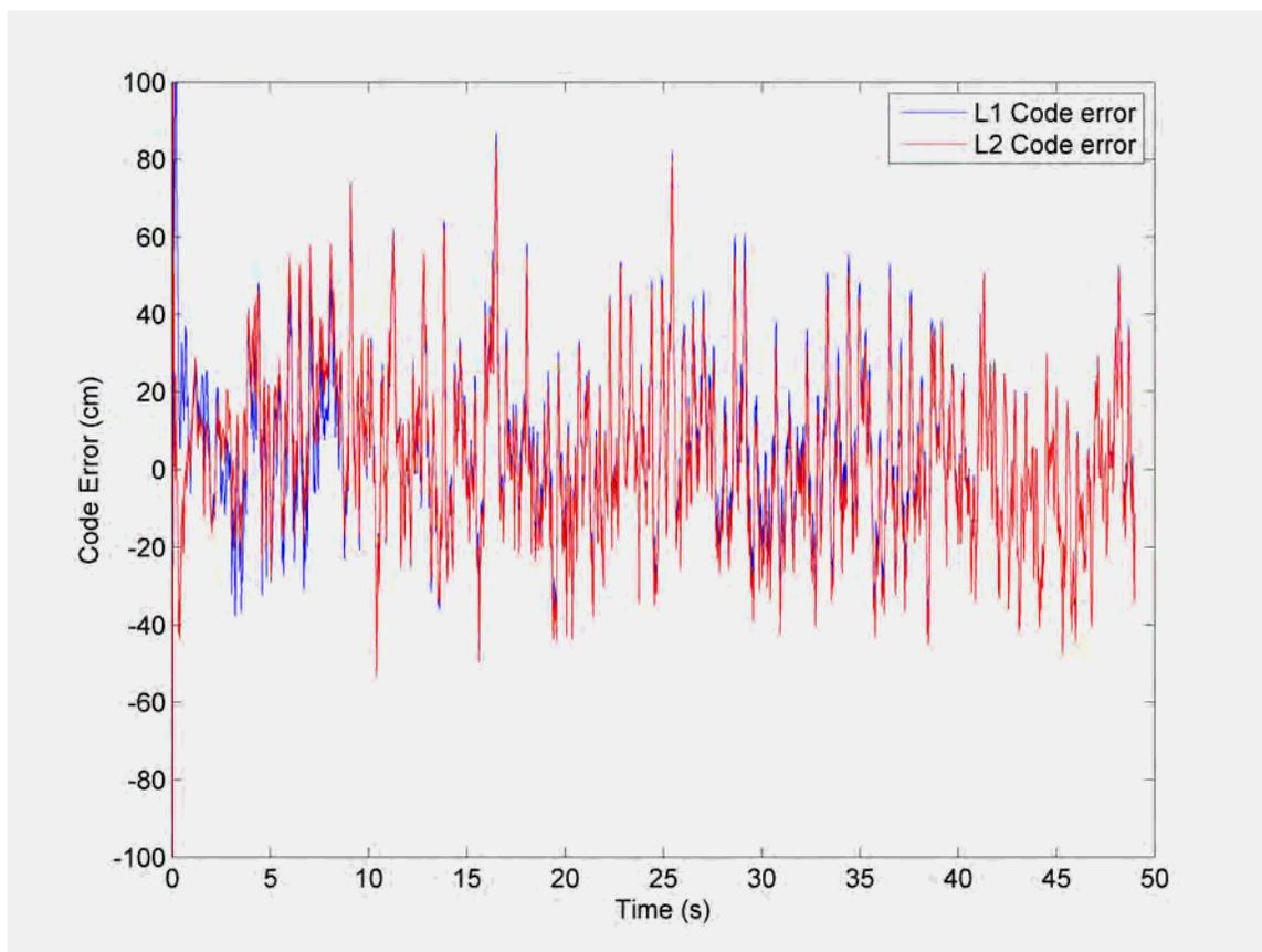
**Figure 6-2: Observed code errors in centimetres for L1 and L2**
