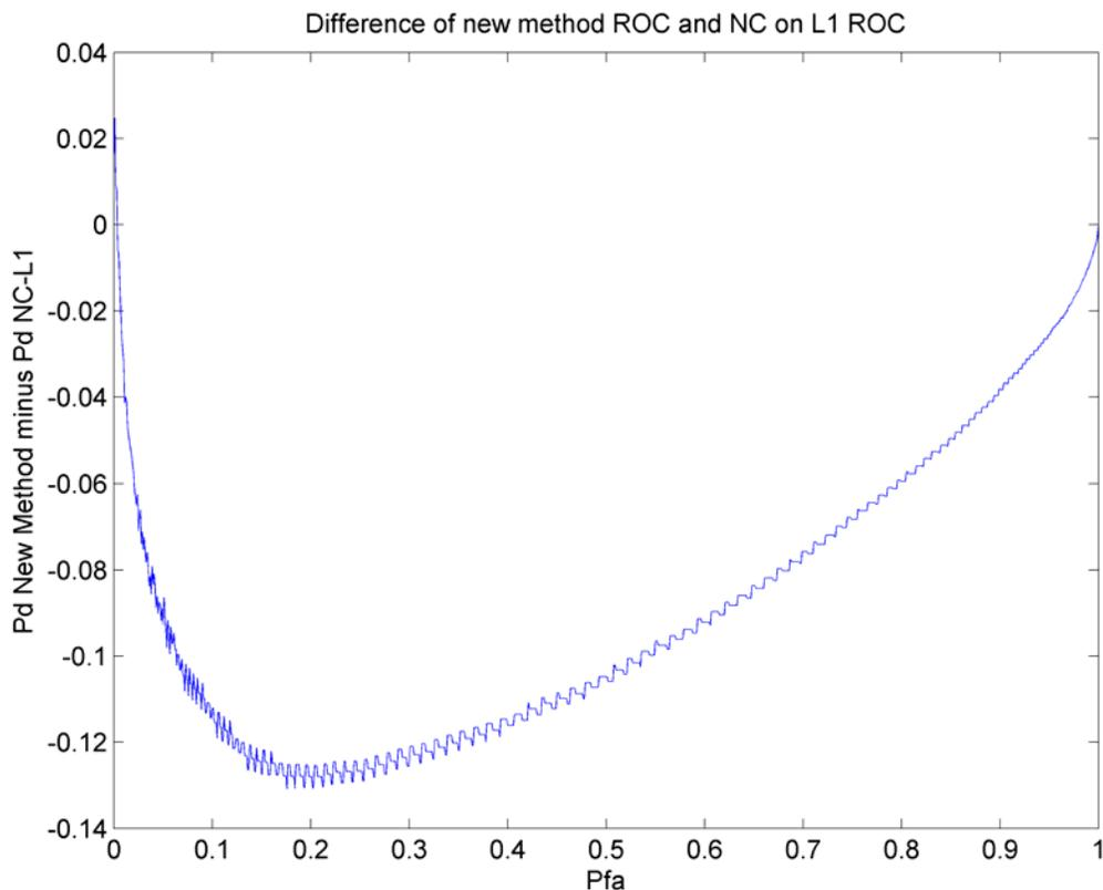
**Figure 4-14 : Difference between the  $\text{Diff}_{L1L2}$  ROC and the ROC obtained for a non-coherent acquisition on L1 only while limiting the Doppler error to  $\pm 333.33$  Hz using simulated data**
