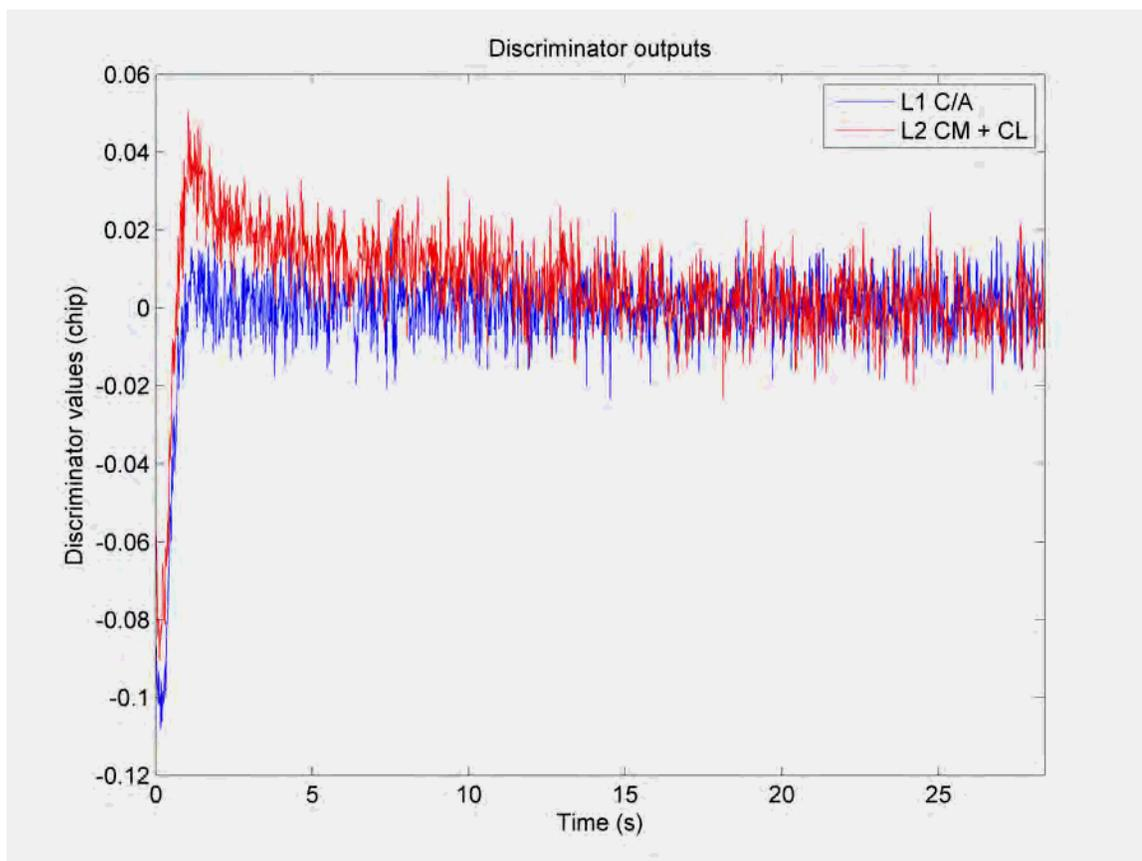
**Figure 5-6: L1 aiding L2 DLL discriminator outputs**
