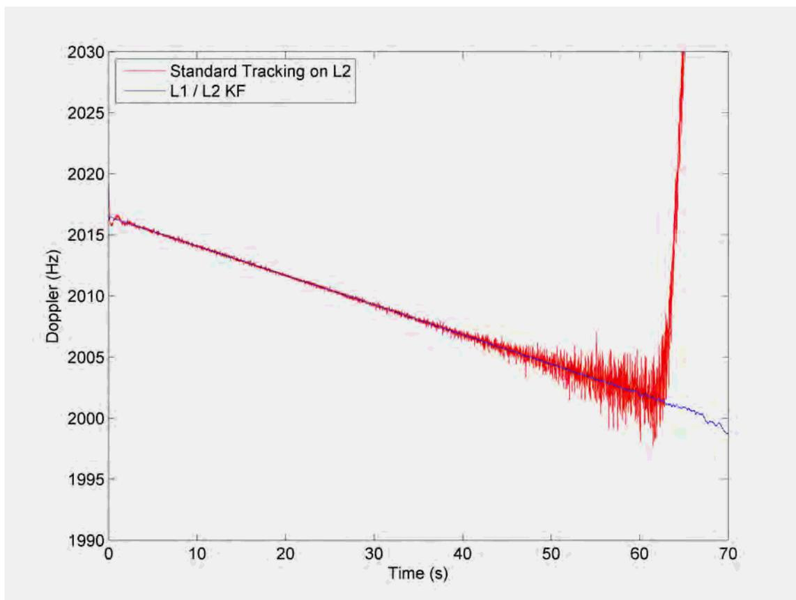
**Figure 6-8: L2 Doppler as measured by the standard L2 only tracking module and the L1/L2 Kalman filter based tracking module**
