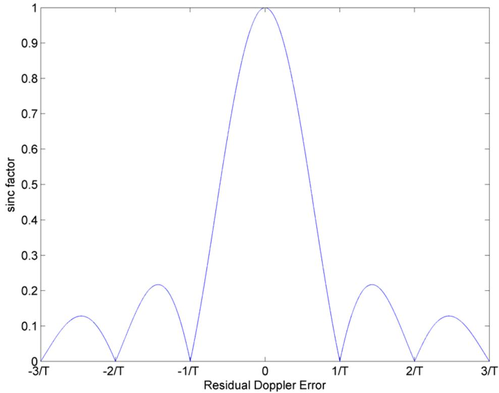
**Figure 2-9: Sinc function attenuation factor as a function of the residual frequency error and  $T$**
