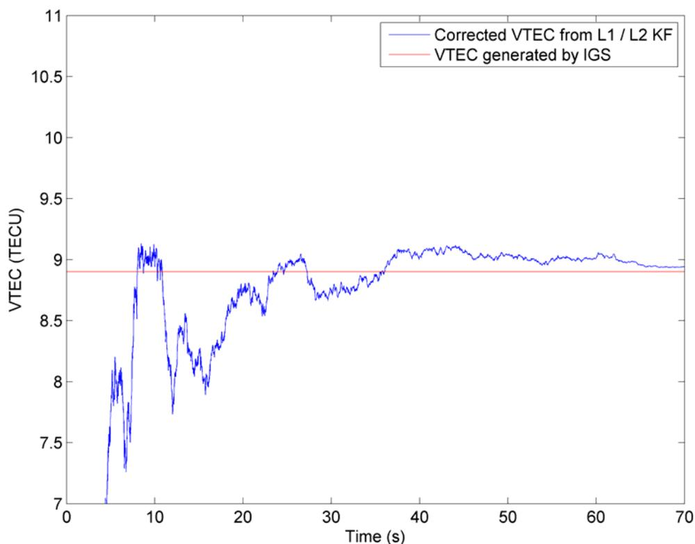
**Figure 6-12: Satellite and receiver bias free vertical TEC values derived from the Kalman filter based tracking and compared to the IGS generated values**
