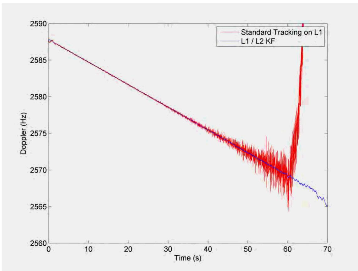
**Figure 6-7 : L1 Doppler as measured by the standard L1 only tracking module and the L1/L2 Kalman filter based tracking module**
