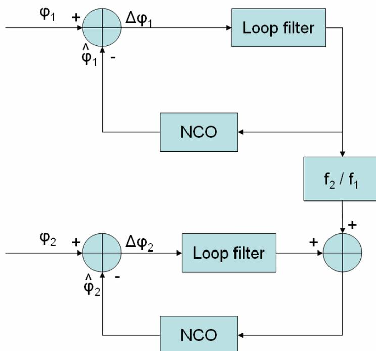
**Figure 5-5: L1 PLL aiding L2 PLL**
