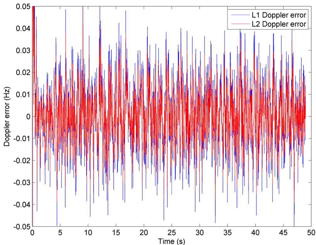
**Figure 6-1: Observed Doppler frequency error for L1 and L2**
