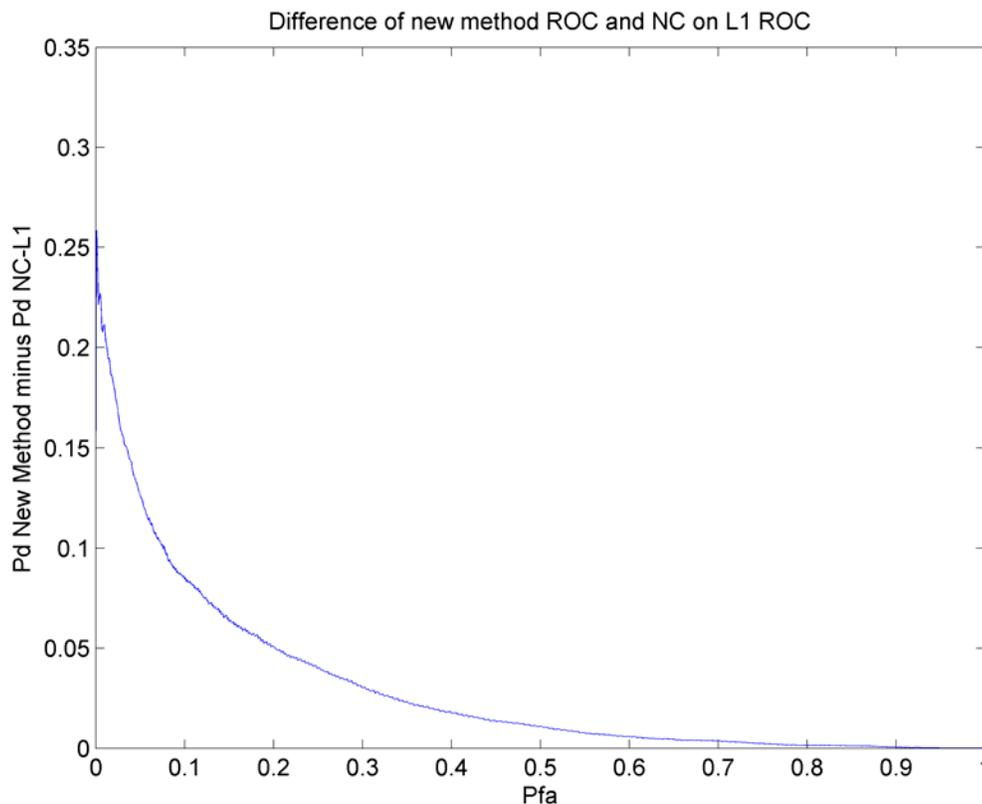
**Figure 4-24 : Difference between the  $\text{NCDiff}_{L1L2}$  and the ROC obtained for a non-coherent acquisition on L1 only using real data**
