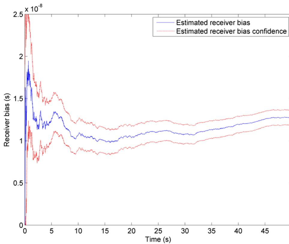
**Figure C-3: Estimated receiver bias from the least-squares method using the Kalman filter based combined tracking outputs as well as the  $1\sigma$  confidence**
