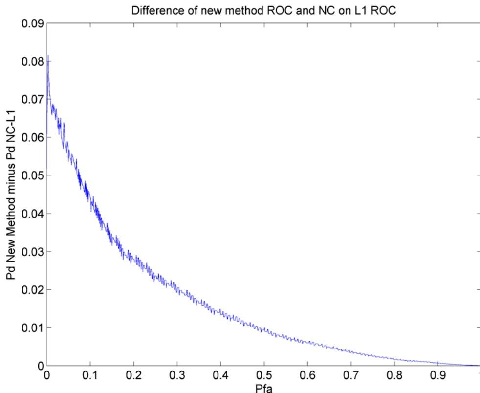
**Figure 4-12 : Difference between the  $NC_{L1L2}$  ROC and the ROC obtained for a non-coherent acquisition on L1 only using simulated data**
