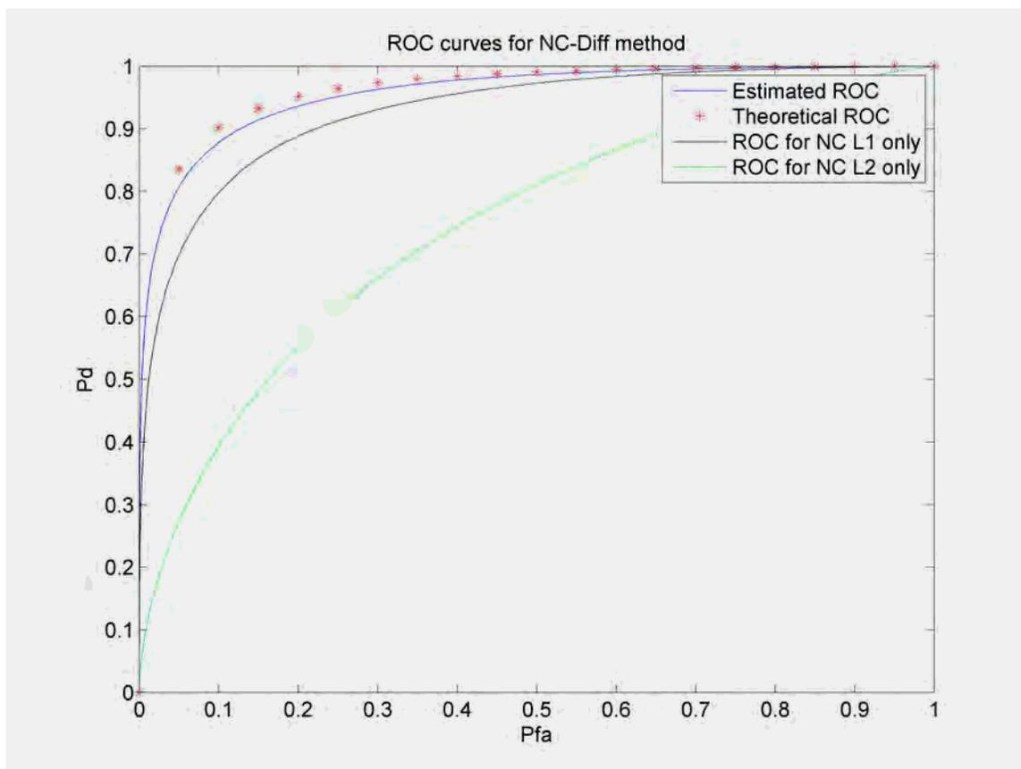
**Figure 4-17 : Theoretical and simulation estimated ROC curves for the NCDiff<sub>L1L2</sub> method**
