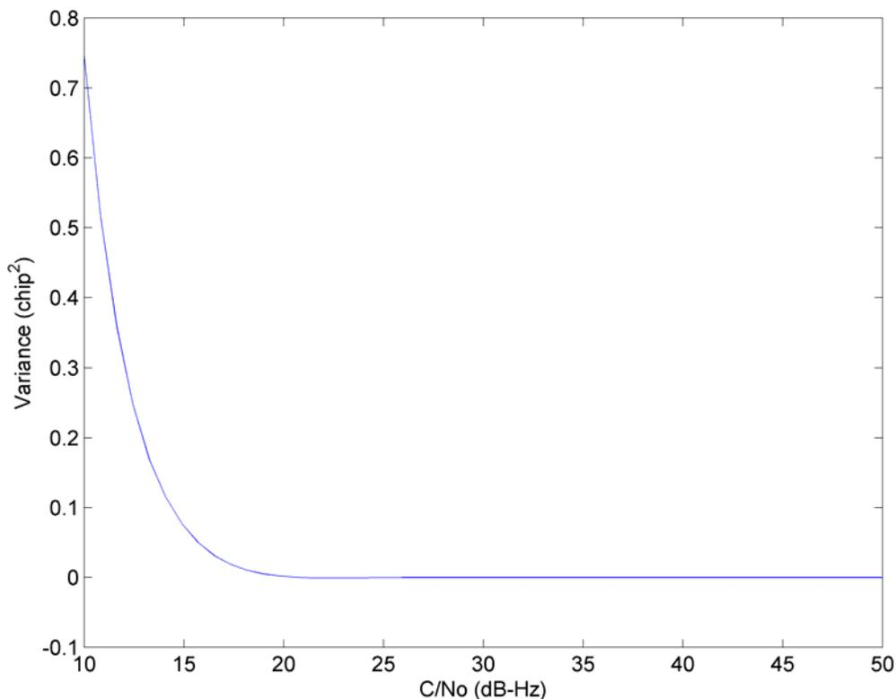
**Figure 5-16: Difference between theoretical variance of the early minus late power and Monte-Carlo variance of the normalized early minus late envelope discriminator as a function of the  $C/N_0$**
