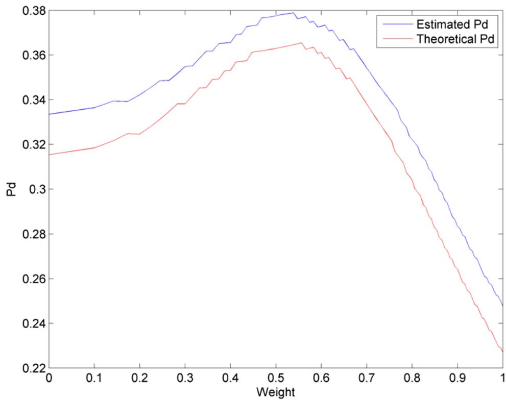
**Figure 4-9: Theoretical probability of detection as a function of the weight applied on L2 for the Diff<sub>L1L2</sub> method**
