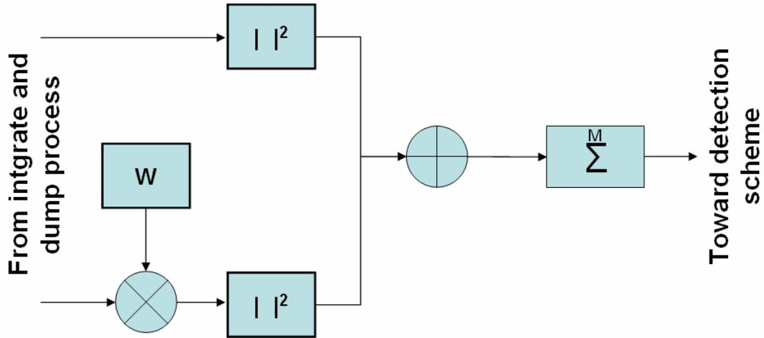
**Figure 3-2 :  $NC_{L1L2}$  method represented as a block diagram**
