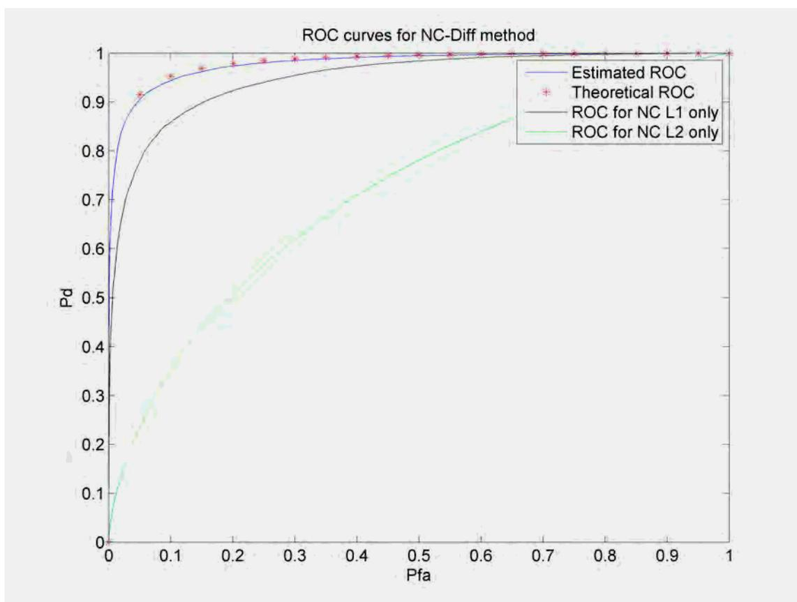
**Figure 4-23 : Theoretical and “real data” estimated ROC curves for the NCDiff<sub>L1L2</sub> method**
