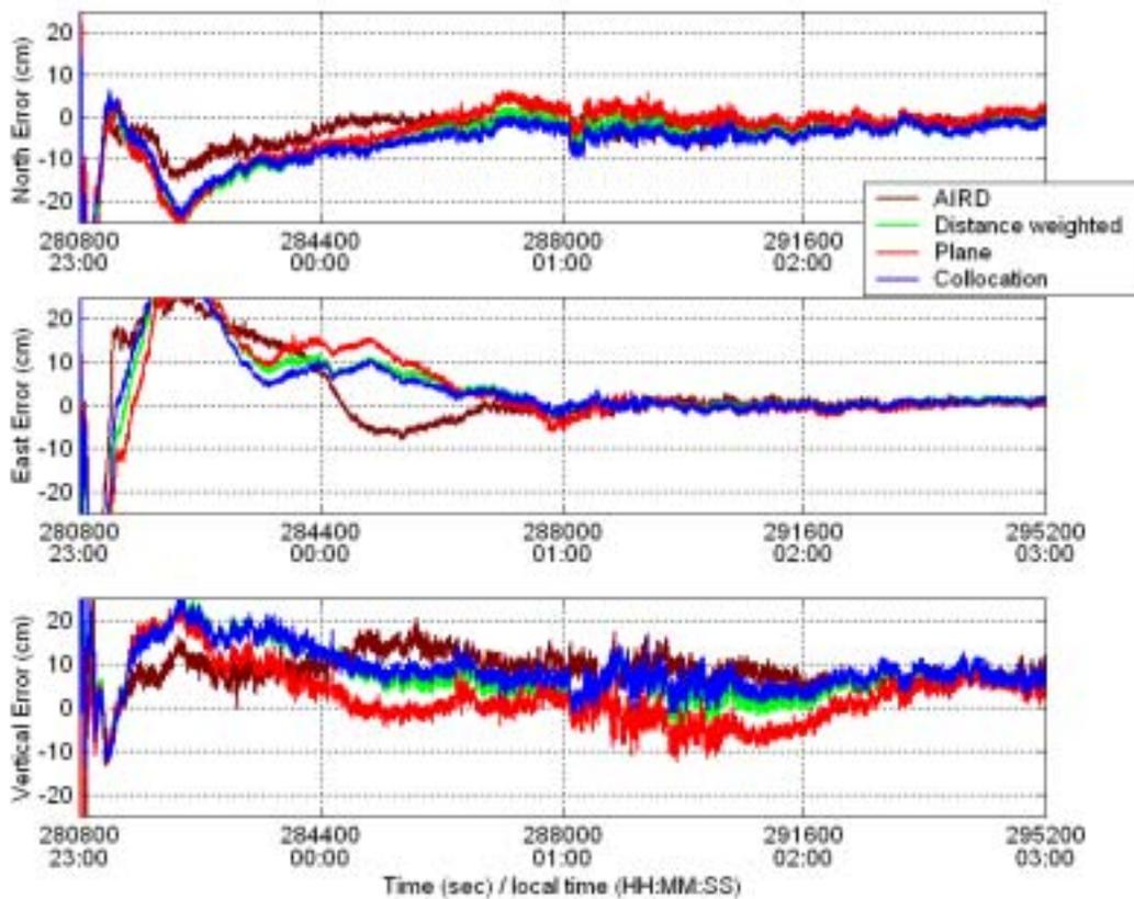
Figure 6.17: North, east and vertical position errors over time for the single reference station approach and multiple reference station approach using three interpolation methods with KAR disabled in GrafNav™
