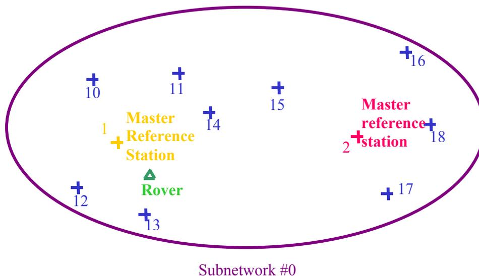
Figure 3.5: One subnetwork with two master reference stations
