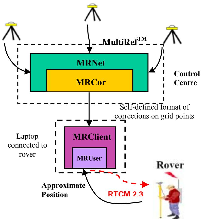
Figure 4.3: MultiRef™ option 2 structure
