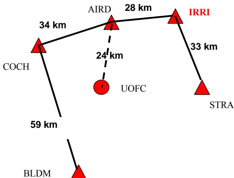
Figure 6.2: Network configuration (the master station is shown in red.)
