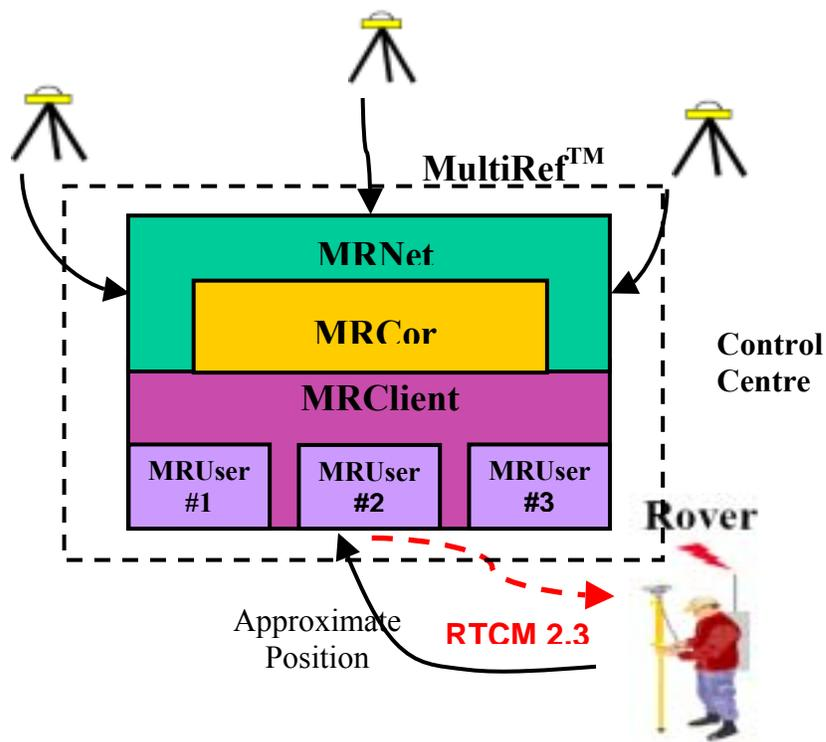
Figure 4.2: MultiRef™ option 1 structure
