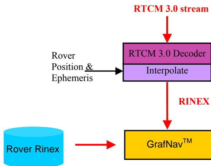
Figure 5.1: Post-mission test scheme at rover
