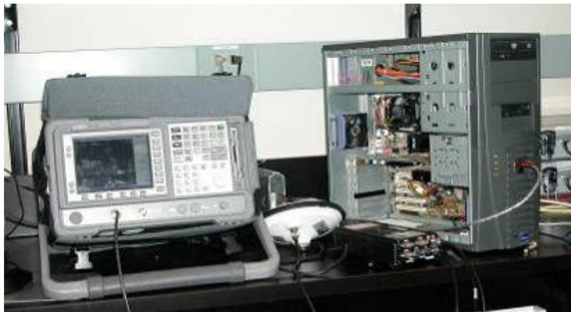
**Figure 3.2: Interference Measurement near a PC**
