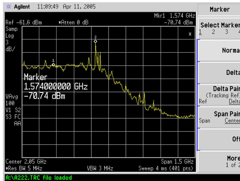
**Figure 3.6: Interference Measurement in ICT Building - Enlarged Scale of Frequency Span**
