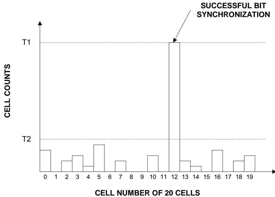
Figure 6.2: A histogram showing successful bit synchronization
