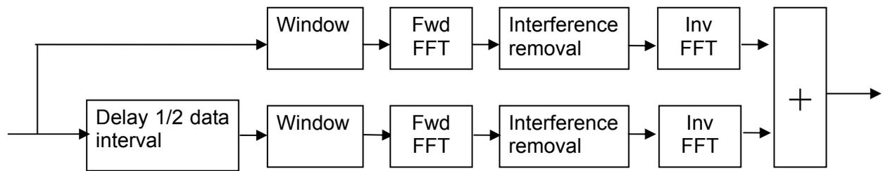
Figure 7.4: Block diagram of 50 percent overlap processing
