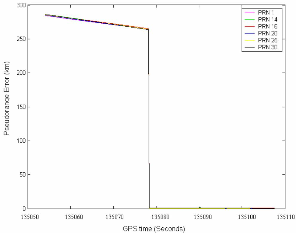
Figure 6.6: Pseudorange error using improved bit synchronization procedure
