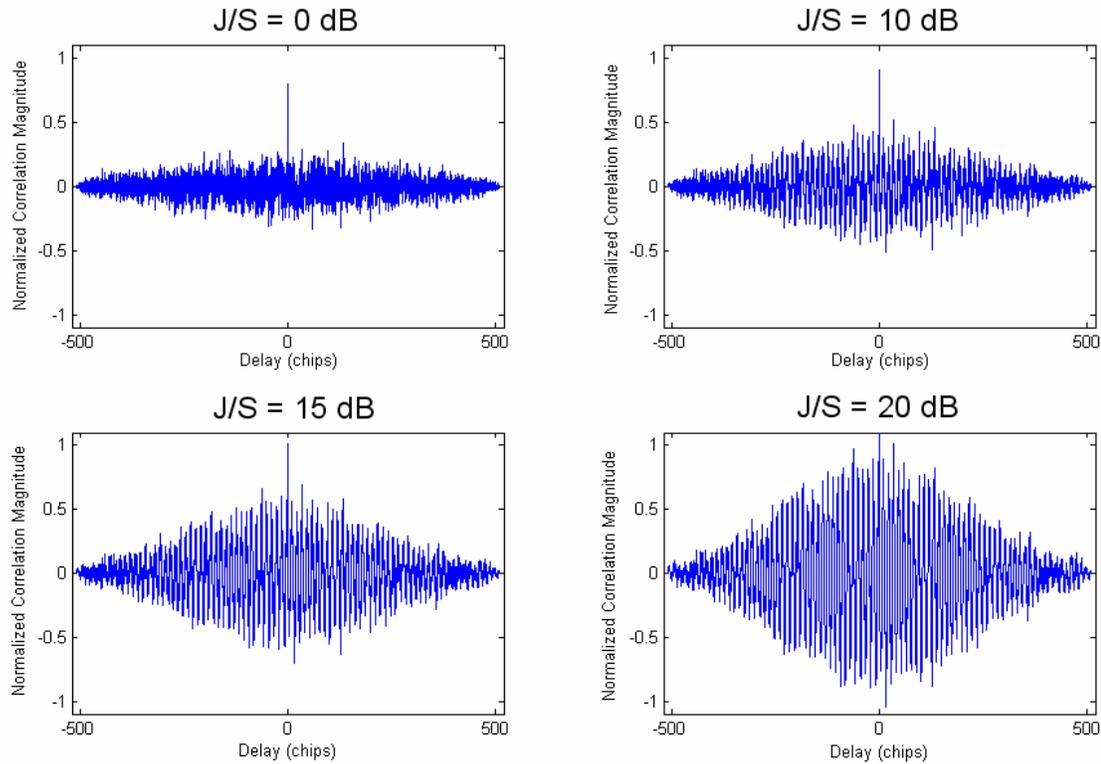
Figure 4.3: Correlation for CW interference of different power levels
