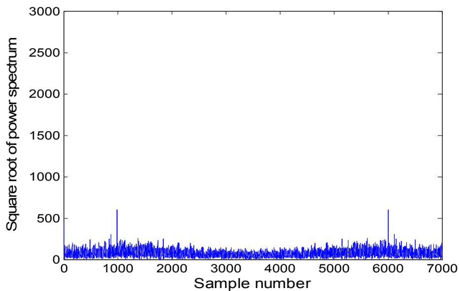
Figure 3.4: 1 ms FFT without CW interference
