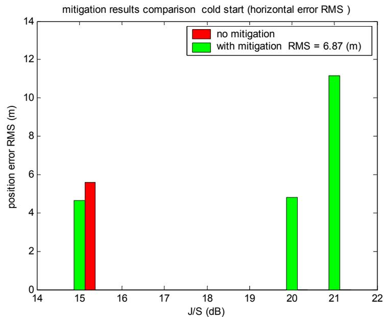
Figure 5.15: Mitigation results comparison with AM interference
