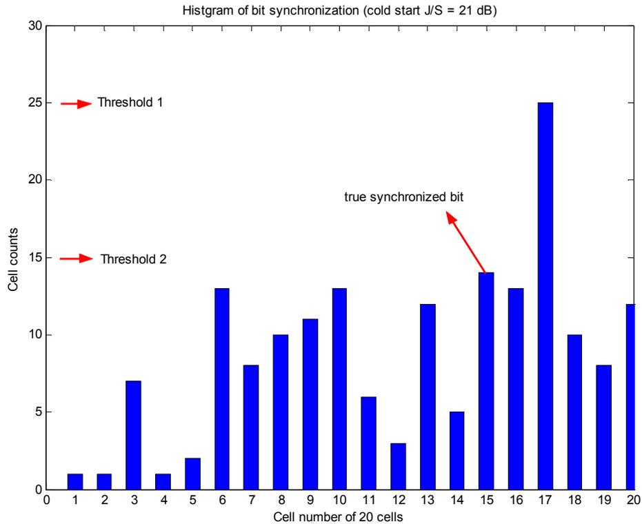
Figure 6.3: Bit synchronization result for PRN 20
