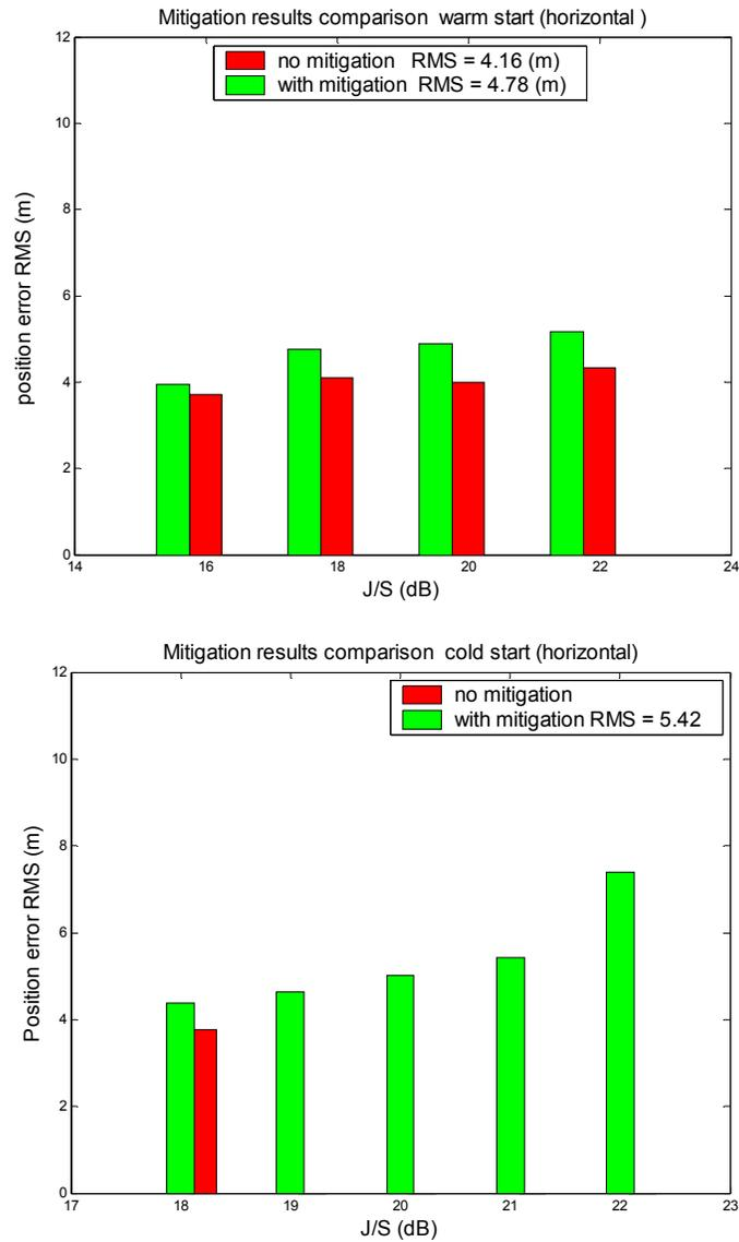
Figure 5.9: Comparison of mitigation results with CW interference
