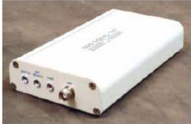
Figure 3.2: Hardware front-end “GPS Signal Tap”
