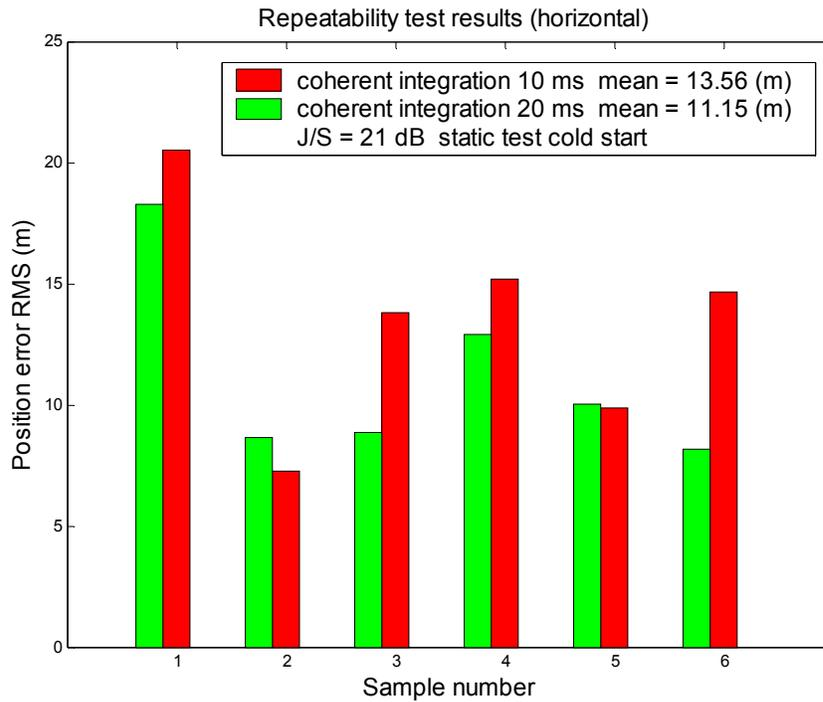
Figure 5.11: Comparison of coherent integration time on position
