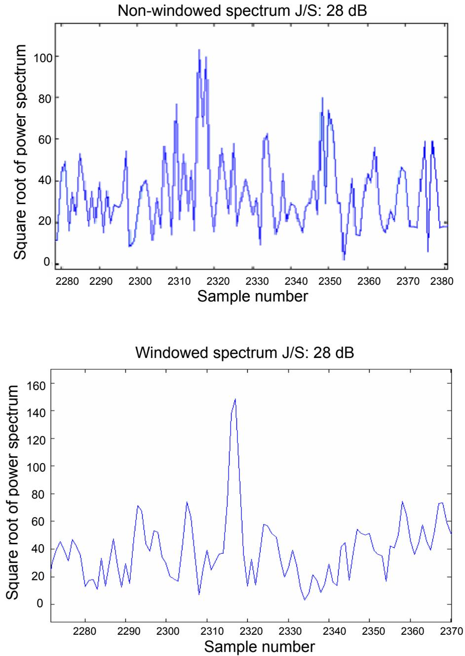
Figure 7.5: Enlarged spectra of windowed and non-windowed data
