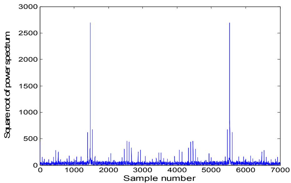
Figure 3.5: 1 ms FFT with CW interference ( $J/S = 30$  dB)
