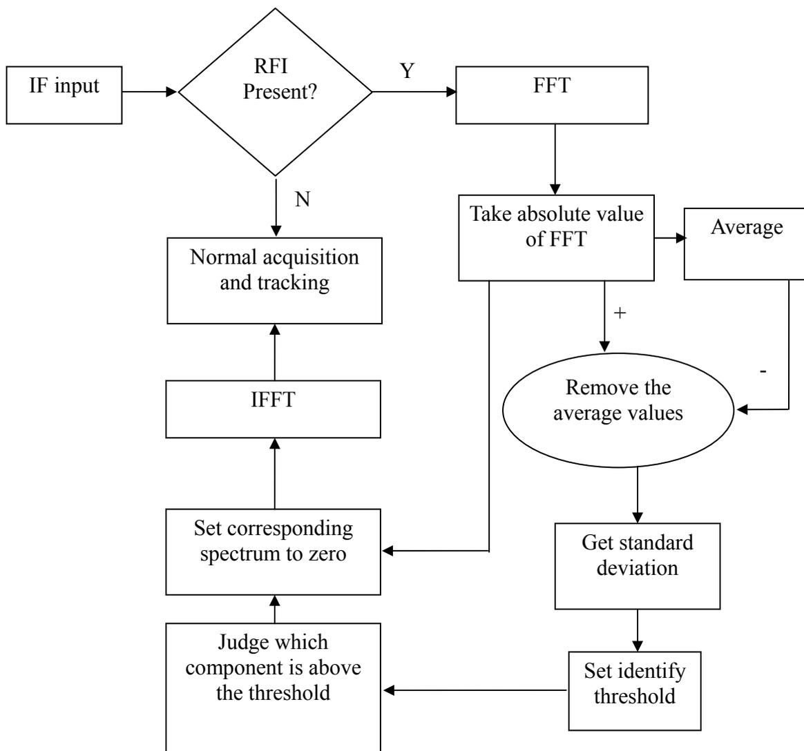
Figure 3.6: Flowchart of frequency excision algorithm
