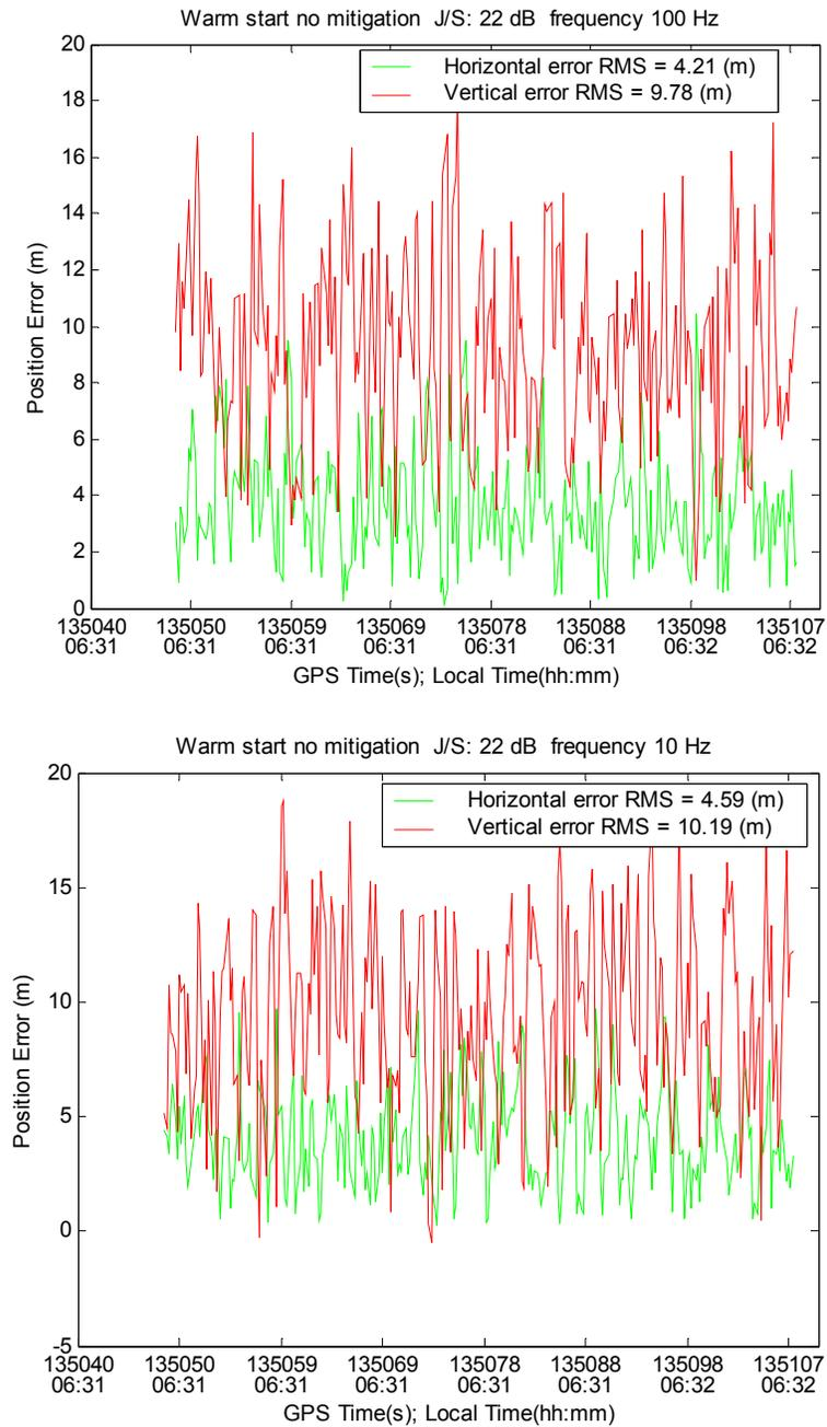
Figure 5.13: Impact of modulating signal frequency of AM interference on mitigation results
