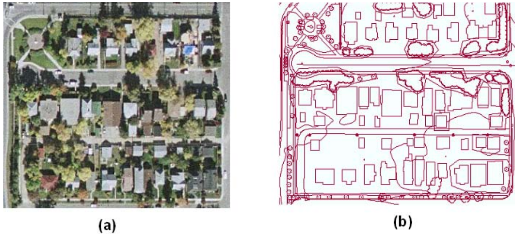
Figure 2.1: Example of Raster and Vector Data: a) Raster Data, b) Vector Data
