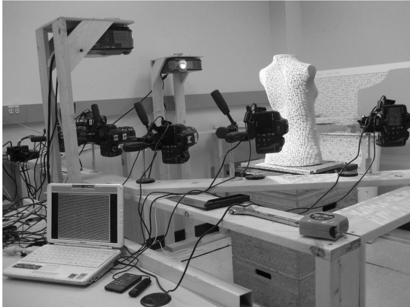
**Figure 5.20 Dual projector sensor arm setup showing all the cameras pointed towards the torso mannequin**
