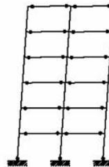
(b) Beam - Hinging Mechanism
