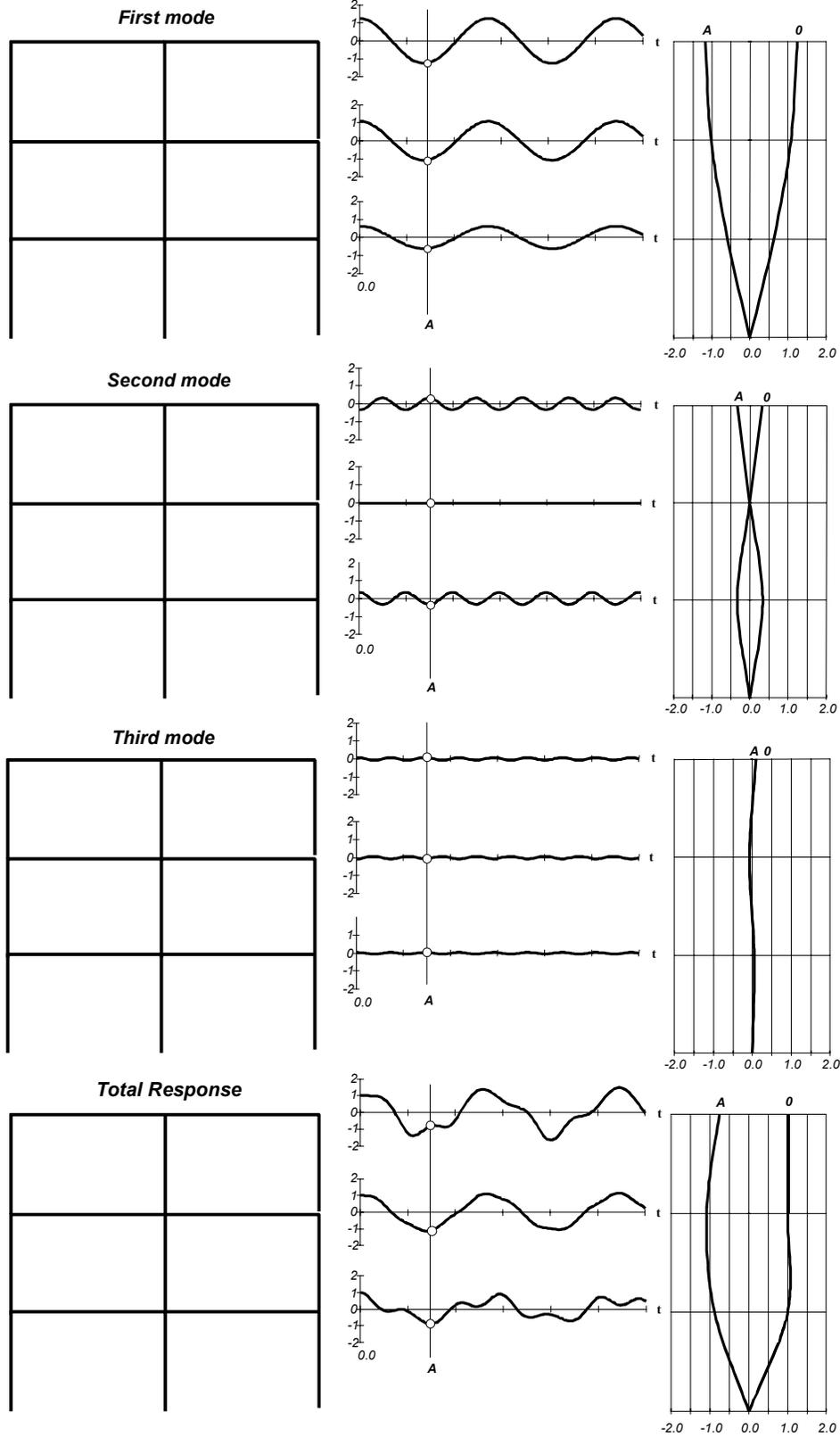
Fig. 2 - Response to initial displacement conditions. Case (a)
