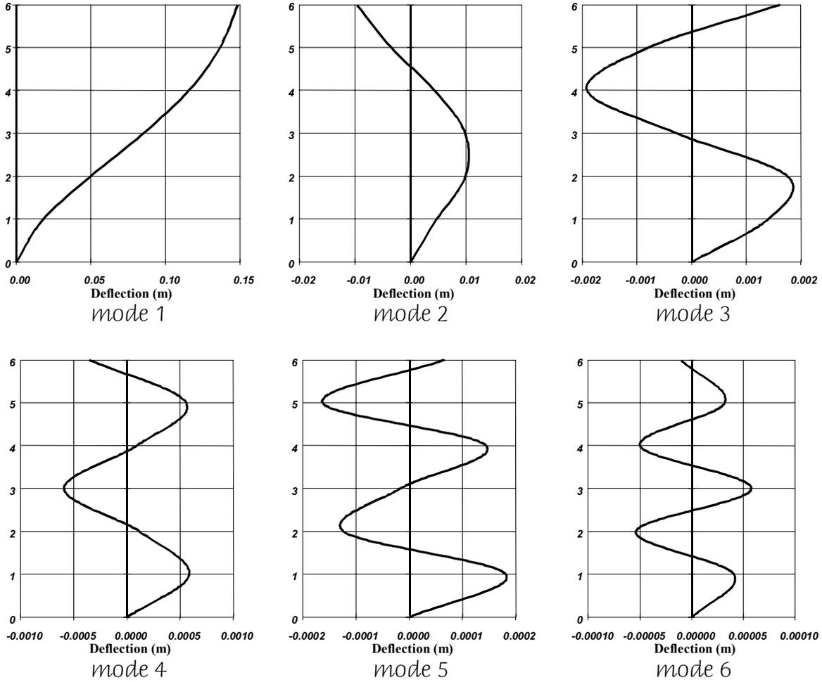
**Fig. 16 - Example 6 - Maximum lateral displacements for each mode**
