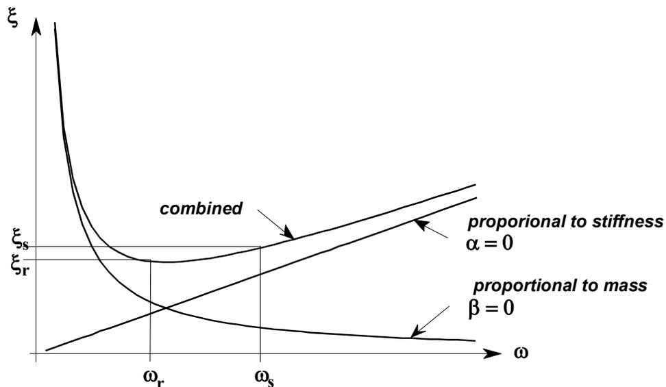
Fig. 3 - Relationship between damping and frequency for Rayleigh's damping
