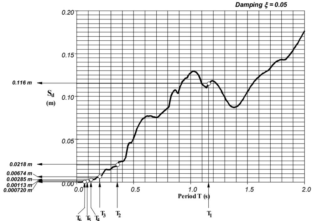
Fig. 15 - Example 6 - Displacement response spectrum for El Centro NS record
