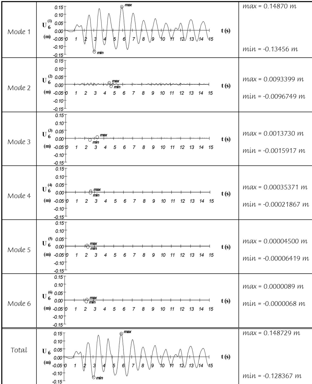
Fig. 12 - Example 5 - Roof displacements from each mode and total response
