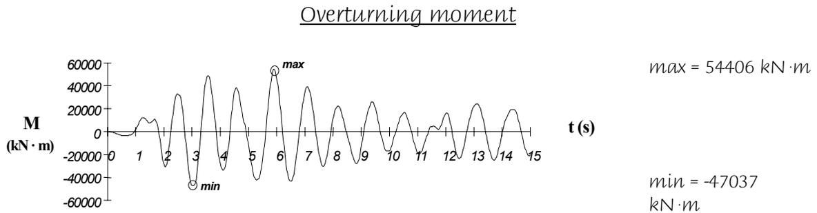
**Fig. 14 - Example 5 - Overturning moment of the structure**
