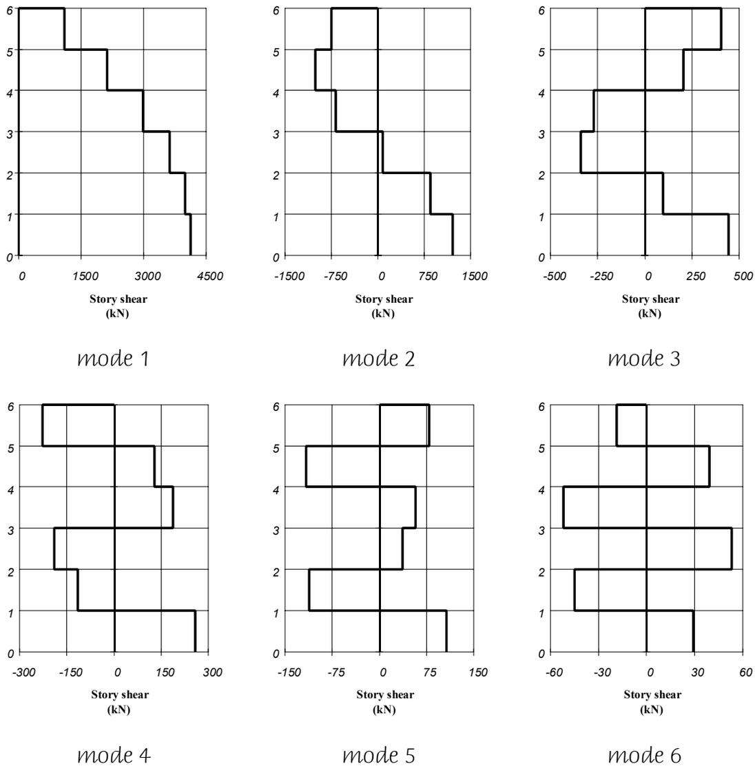
**Fig. 19 - Example 6 - Maximum story shear for each mode**
