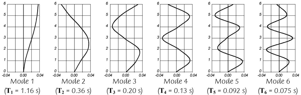
Fig. 10 - Example 5 - Structure vibration periods and modes
