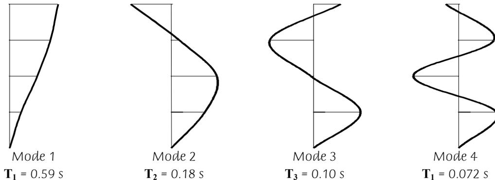
Fig. 6 - Example 4 - Vibration modes and periods of the structure
