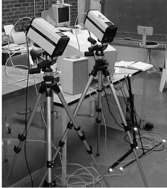
Figure 2.6: Infrared tracking cameras
