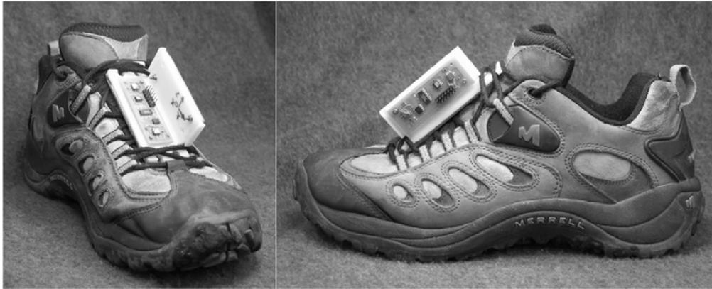
Figure 2.4: Prototype sensor array attached to shoe
