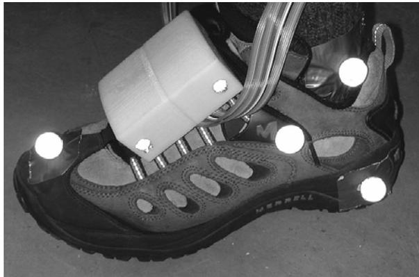
Figure 6.1: Reflective markers on shoe and footpod
