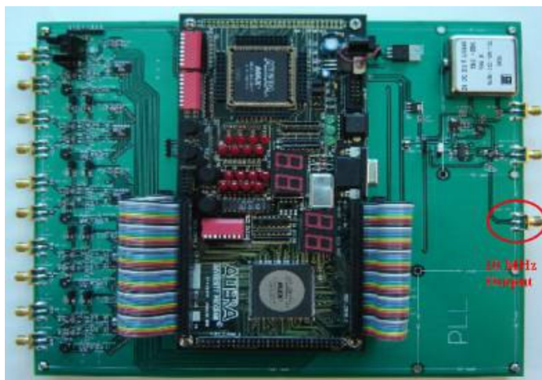
(b) Baseband with Five Channels & Altera FPGA (1 st Generation Receiver)
