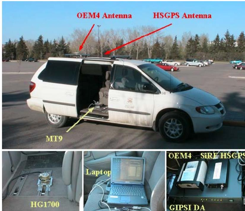
Figure 6.2: Equipment set-up on the test vehicle
