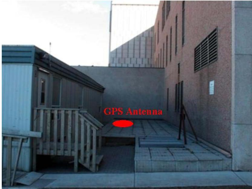
Figure 4.3: Test set-up in a high signal-degraded environment
