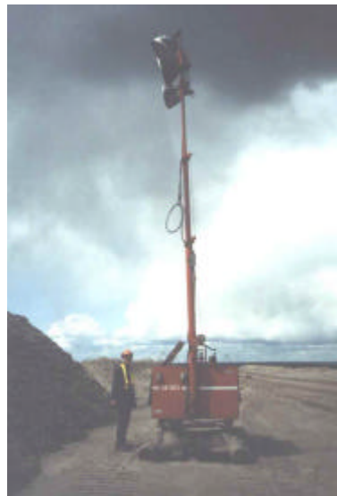
Figure 6.4: Typical Lightplant on Syncrude' s Mine Site
