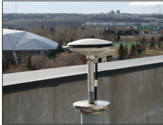
Figure 4.17b: GPS Antenna Receiving WAAS Downlink and GPS Signals
