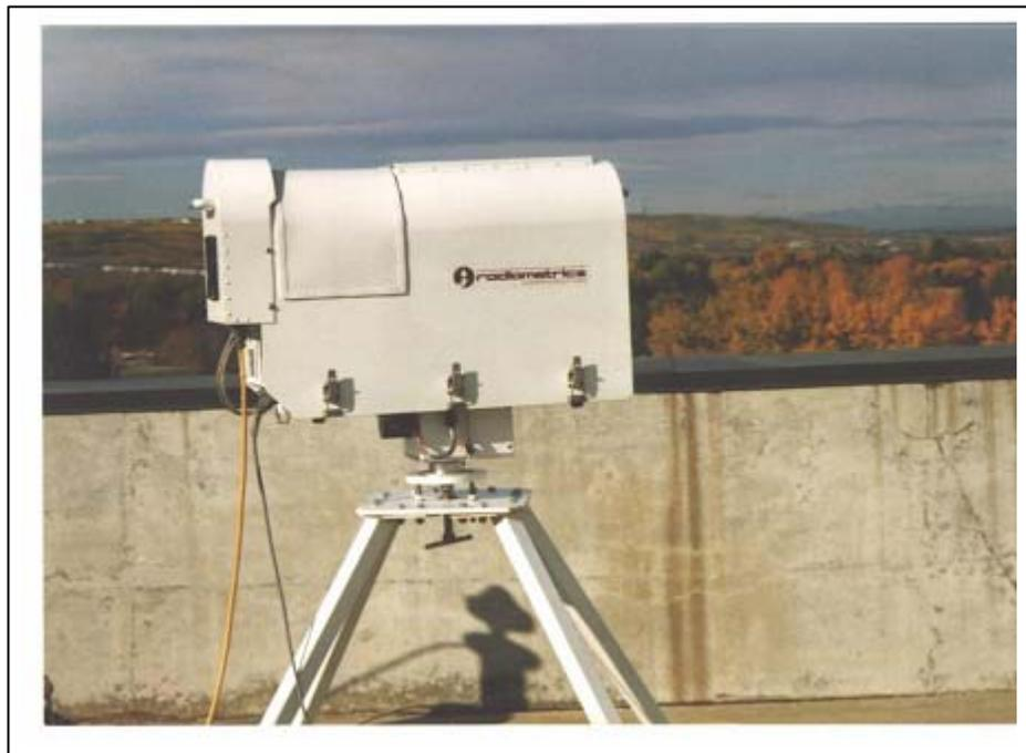
**Figure 4.5 Water Vapor Radiometer (WVR).**
