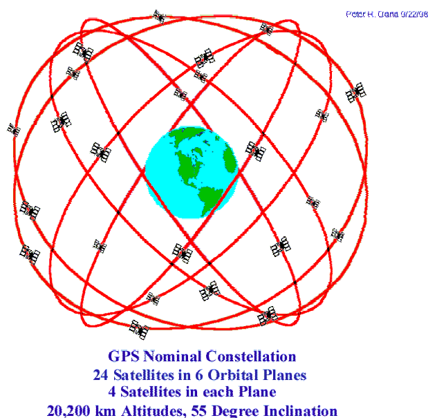
Figure 2.1 GPS satellite constellation
