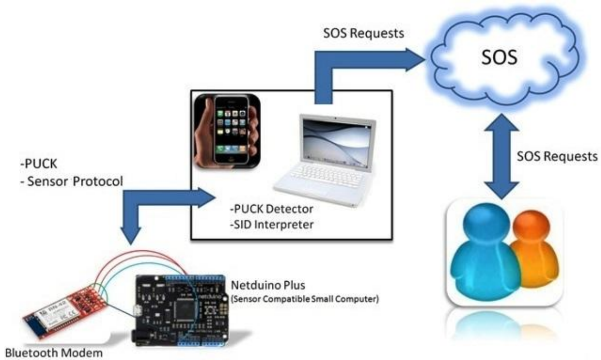
Figure 2.1 The overall workflow of accessing to the sensor measurements
