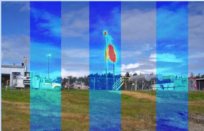
Apparent Temperature in Degrees Kelvin Overlaid thermal IR imagery on the corresponding visible photography.
