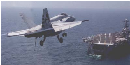
Flying at 240 km/h to a landing target only 45 m long, on a runway only 150 m long.
