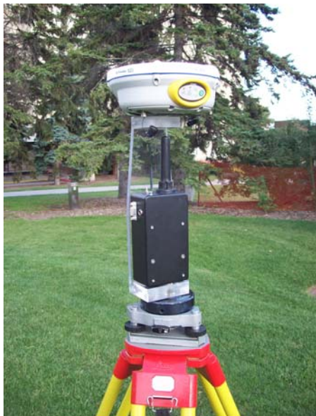
UWB ranging radio and a GPS receiver on a co-axial mount.
