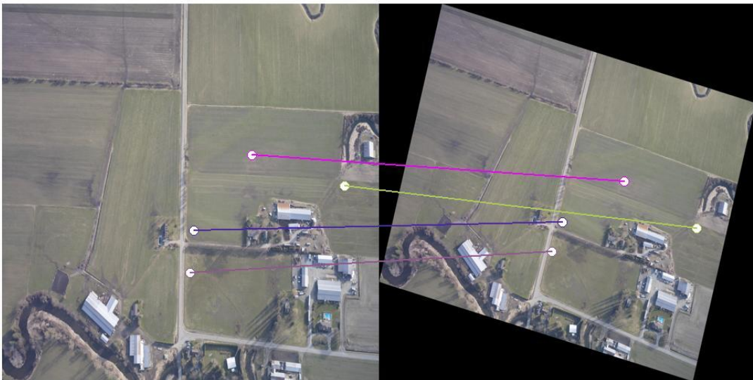
Figure A 4: Descriptor length 128 with scale variation = 0.8 and rotation = 15 and number of sample points 5x5
