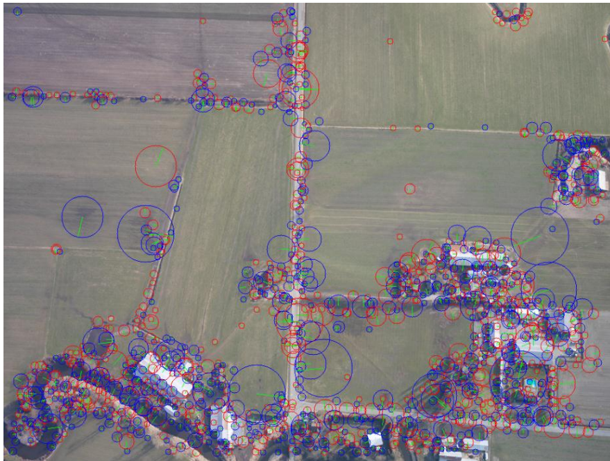
Figure 3.38: Output image with interest points detected (Sheta et al. 2012e)
