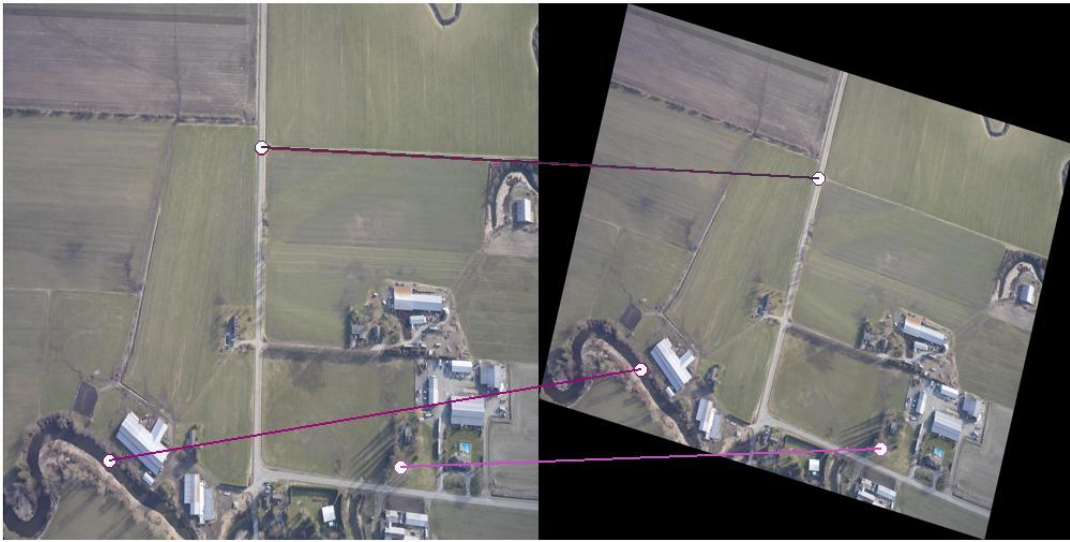
Figure A 22: Descriptor length 36 with scale variation = 0.4 and rotation =15 and number of sample points 9x9
