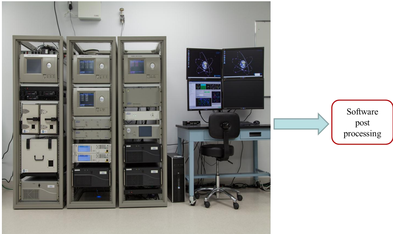
Figure 5.9: Hardware configuration for H/W simulator Spirent GSS 8000 used for flight scenario generation and testing.
