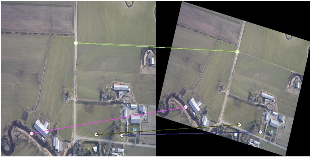
Figure A 24: Descriptor length 36 with scale variation = 0.8 and rotation =15 and number of sample points 9x9
