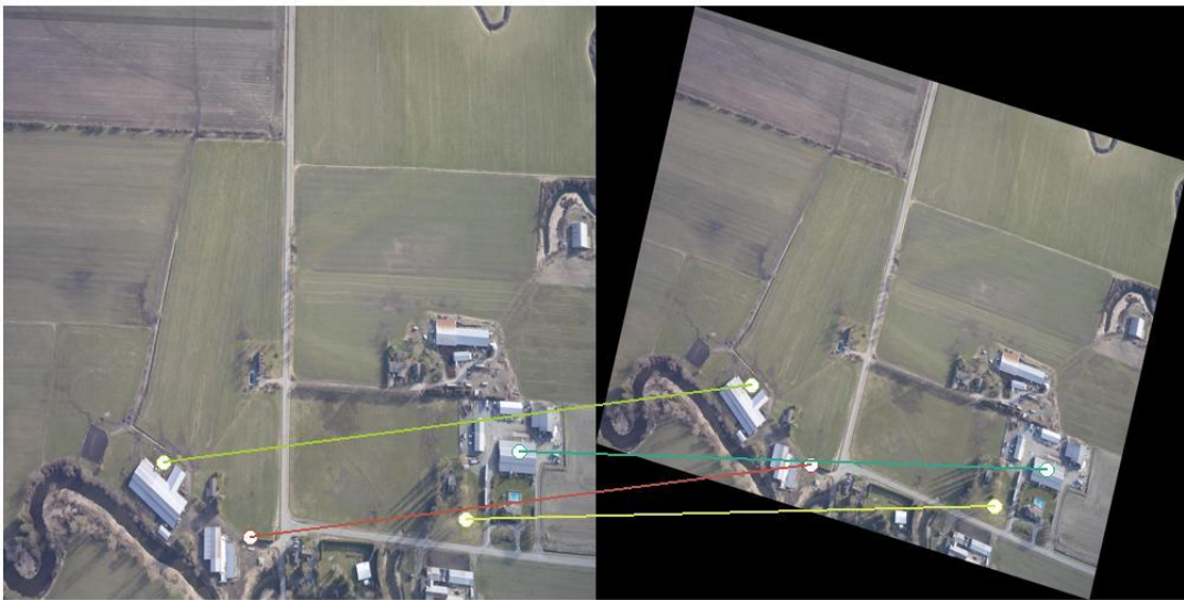
Figure 3.28: Descriptor length 36 with scale variation =0.8 and rotation = 15 and number of sample points 5x5
