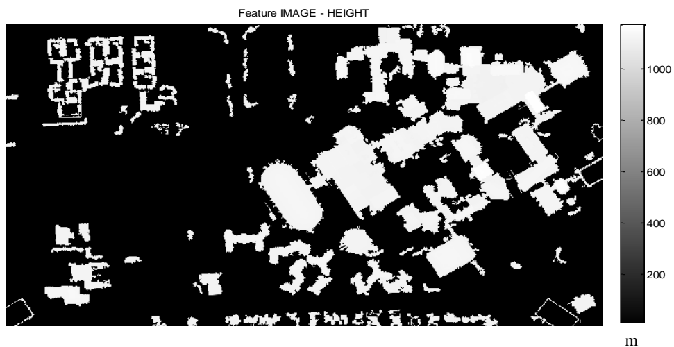
Figure 4-16: Building Extraction Image of the Area of Study (Height Information)
