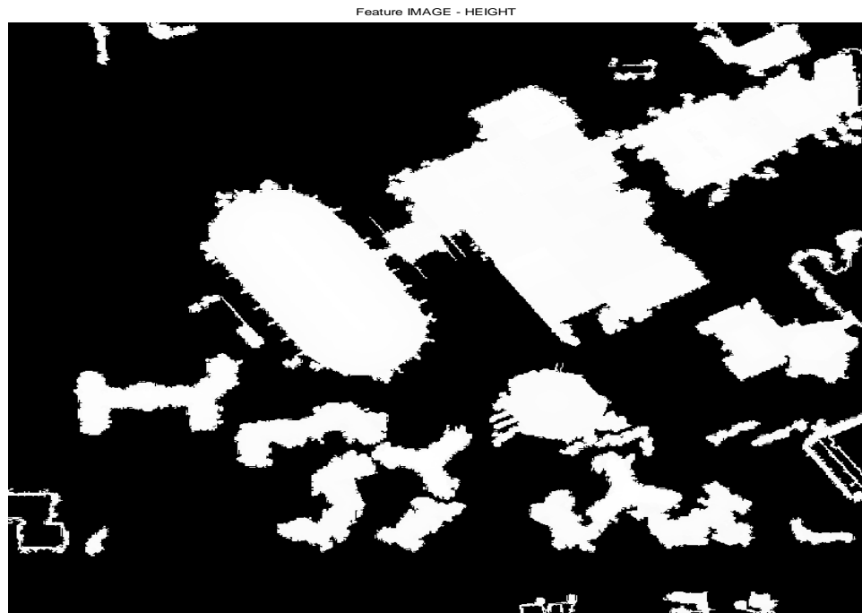
Figure 4-20: Building Extraction Image (Height)
