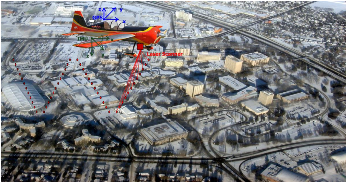
Figure 2-3: LIDAR System Components
