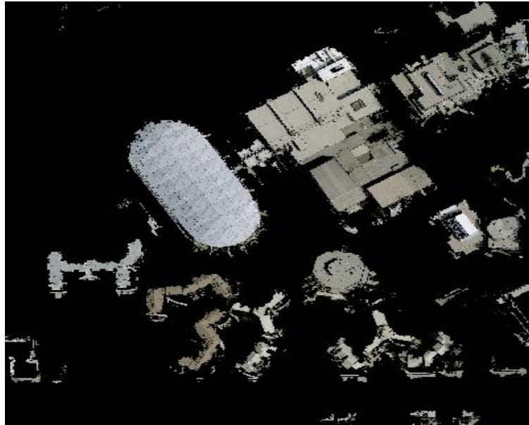
Building image after removing vegetation and shadows
