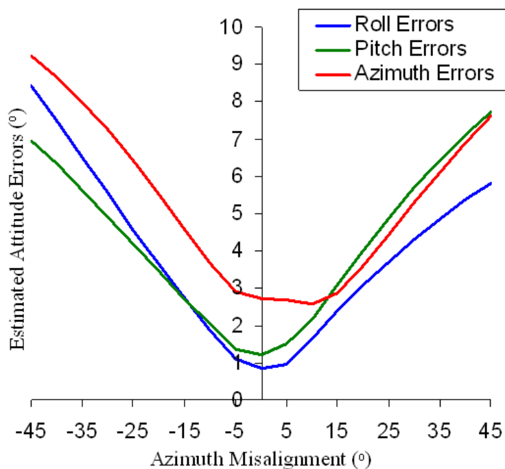
Figure 6-8. Typical induced attitude errors due to misalignment in azimuth
