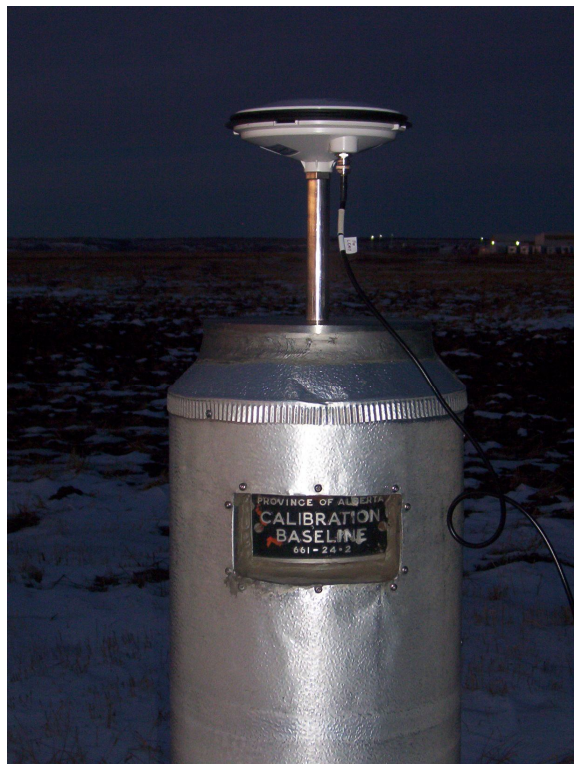
Figure 4.7: Base station for DGPS in Springbank
