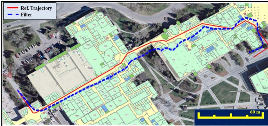
**Figure 6.15: PDR trajectory compared to a reference trajectory**
