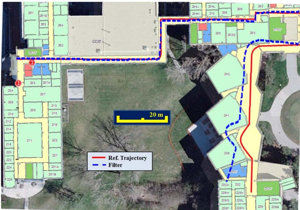
**Figure 6.9: PDR trajectory compared to a reference trajectory**
