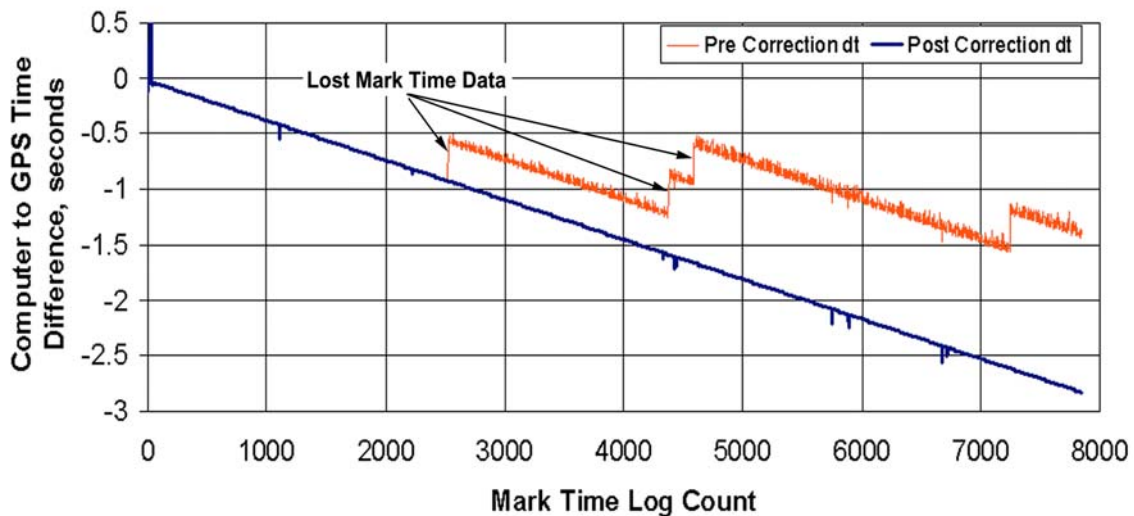
Figure 6-13: Comparison between Video Timing Signal and GPS Mark Time
