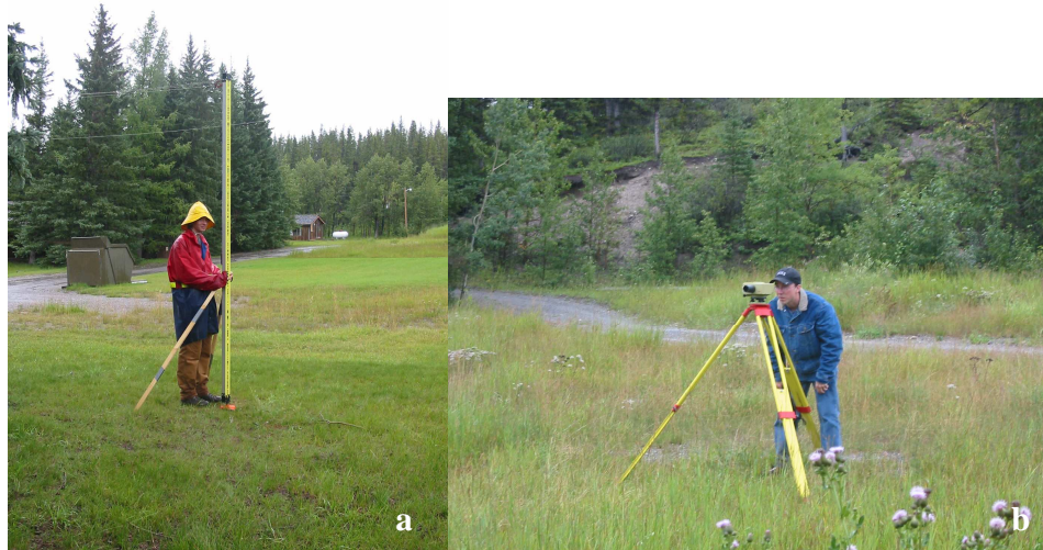
Figure 2.4: Example of conventional leveling with a precise rod (a) and level (b)
