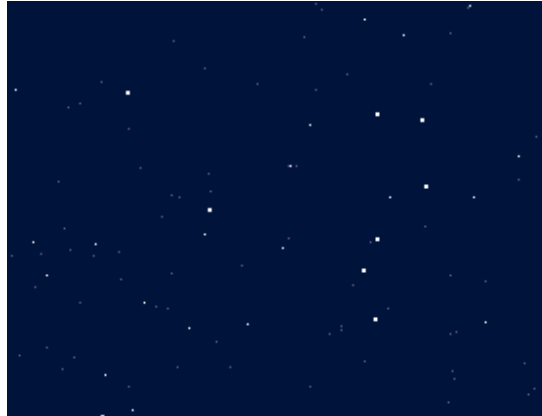
Figure 3.2: Backscatter power of a group of scatterers in a pixel with dominant scatterers
