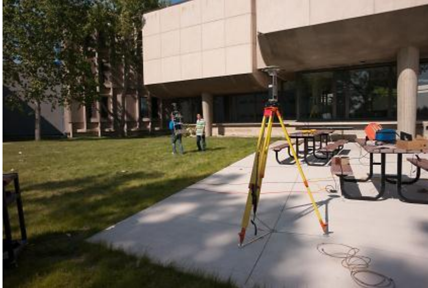
Figure 4.12: Static Station 2 – Outdoor UWB Radio
