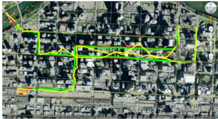
Figure 5.18: Position Performance of the Assumed LOS Peak Strategy for 200 ms Coherent Integration by Employing Kalman Filter (Red: Reference, Green: GSNRx-hs TM Receiver, Yellow: Commercial High Sensitivity Receiver)
