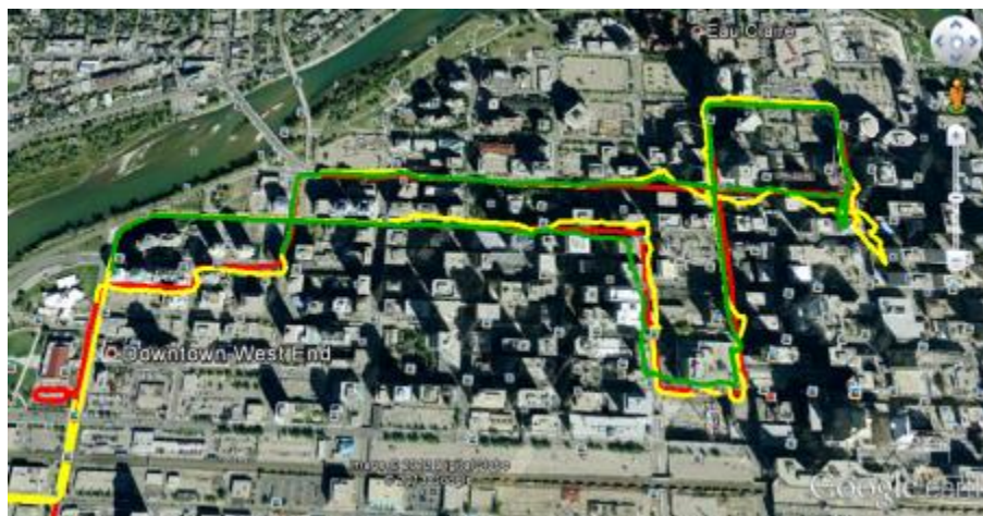
Figure 5.39: Position Performance Comparison for August 19, 2011 Data Set in the Downtown Calgary (Red: Reference, Green: GSNRx-hs TM Receiver, Yellow: Commercial HSGPS)
