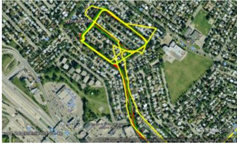
Figure 5.45: Position Performance Comparison for Dense Foliage Data Set (Red: Reference, Green: GSNRx-hs™ Receiver, Yellow: Commercial High Sensitivity Receiver)
