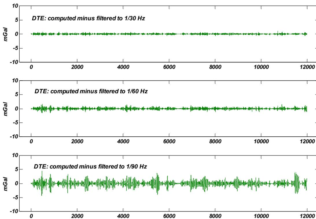
**Figure 3-12: Difference between computed and filtered DTEs (mGal)****Table 3-13: Statistics of the three datasets reduced by the un-filtered DTE (mGal)**
