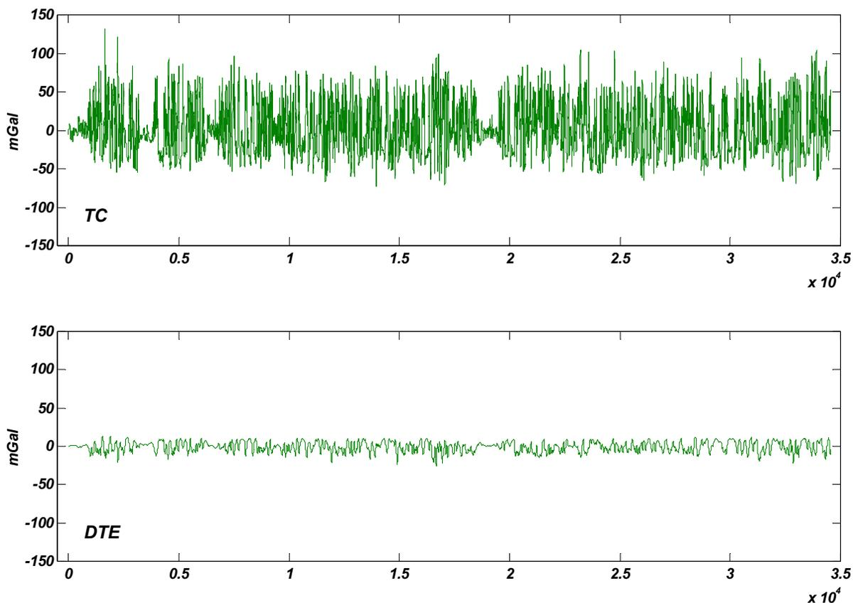
**Figure 3-8: TC and DTE computed at the flight level using 15 arcsec DTM (mGal)**
