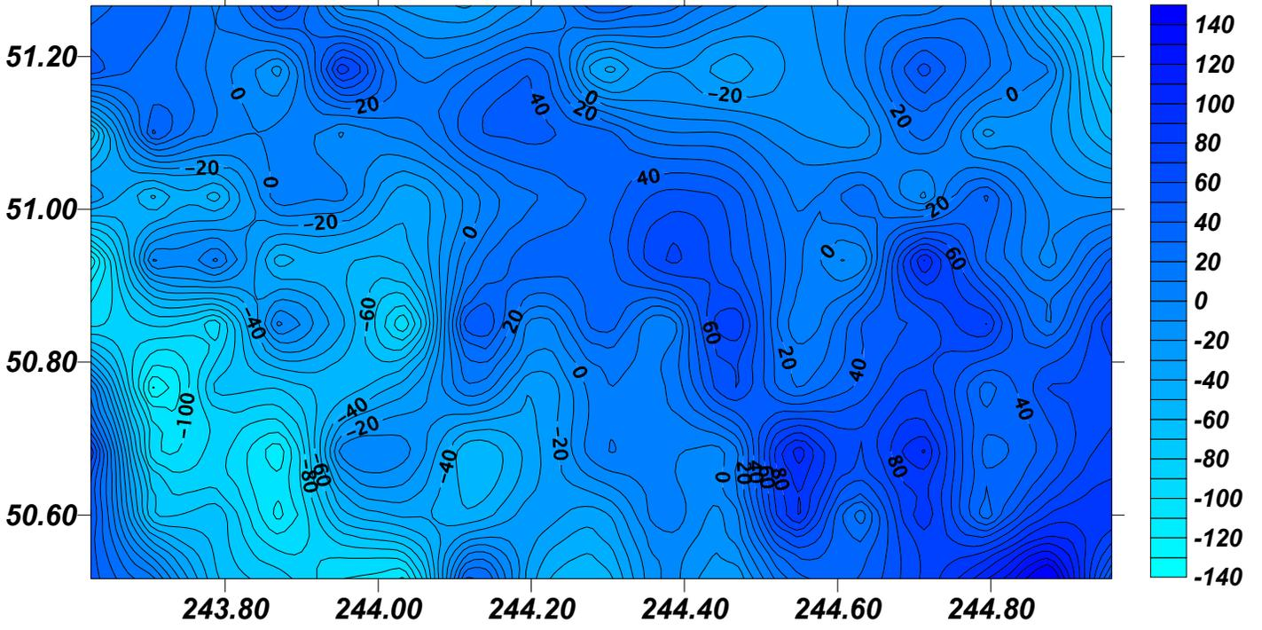
Figure 3-19: Downward continued data\_dte airborne gravity disturbances (mGal)
