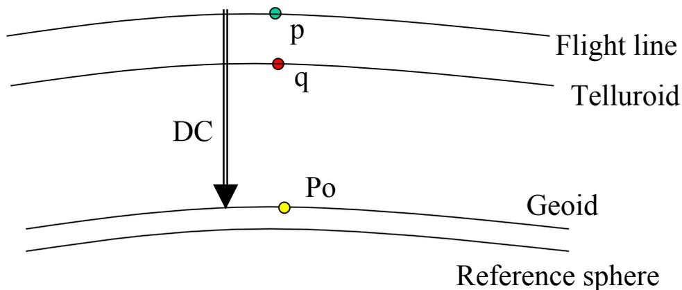
Figure 2-7: Methodology # 1 when computing gravity anomalies
