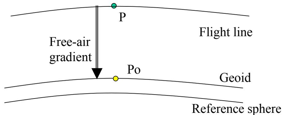
Figure 2-6: Methodology # 2 when computing gravity disturbances
