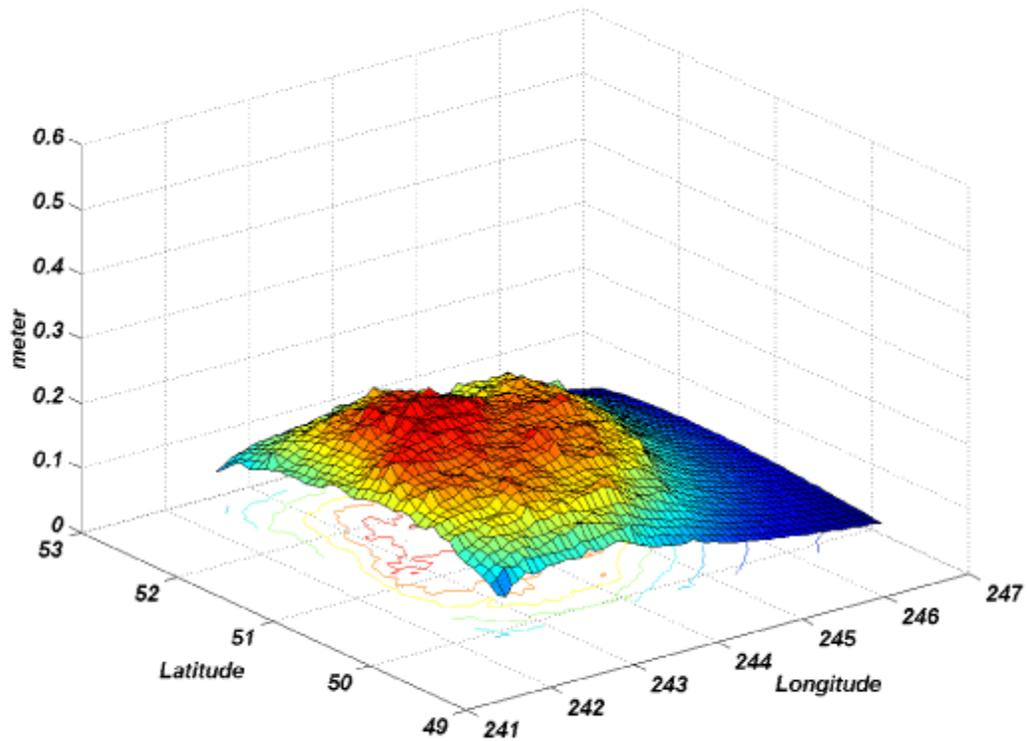
**Figure 4-3: Difference in the geoid contributions of the DTE using 15 and 30 arcsec DTMs (m)**
