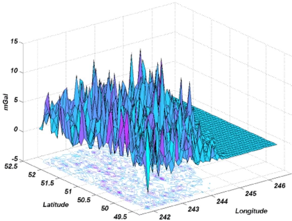
Figure 3-5: Difference between the TC computed from a 15 and 60 arcsec DTM (mGal)
