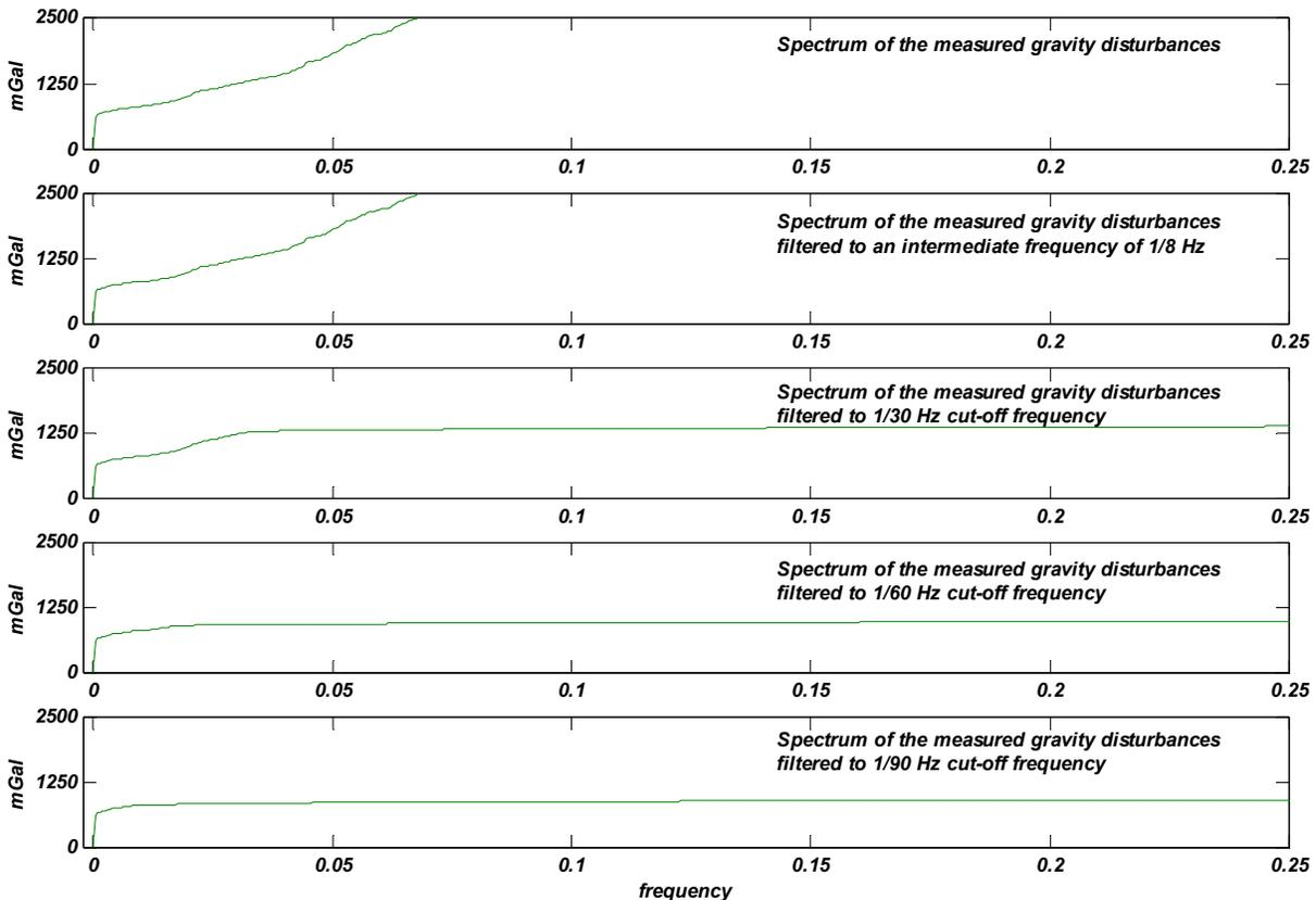
Figure 2-4: Cumulative spectra of the measured and filtered gravity disturbance
