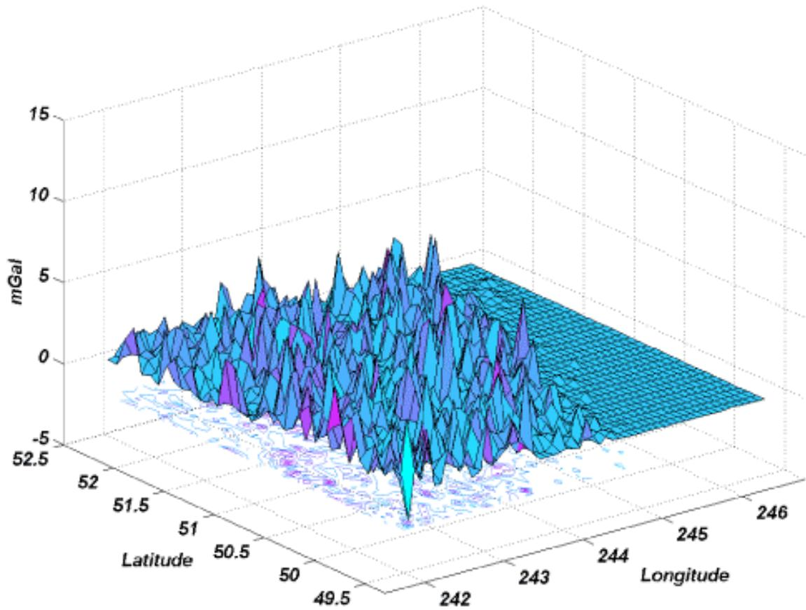
Figure 3-4: Difference between the TC computed from a 15 and 30 arcsec DTM (mGal)
