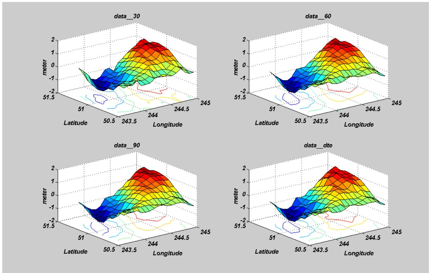
Figure 4-9: The four residual geoids computed from the four data sets created using the 1<sup>st</sup> methodology (m)
