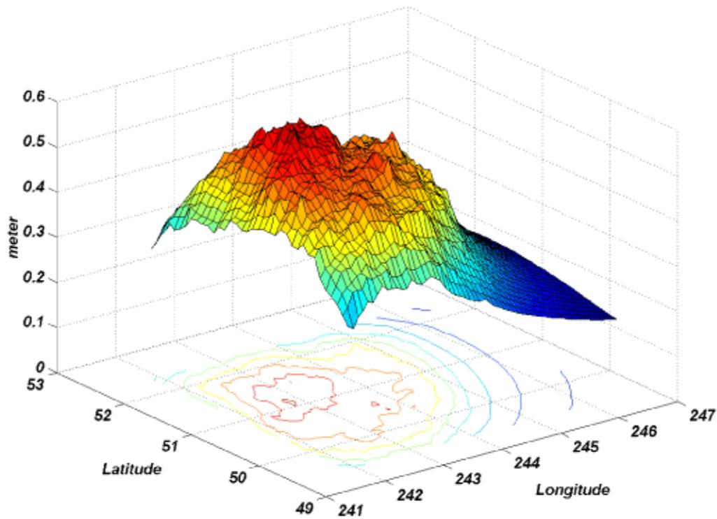
Figure 4-2: Difference in the geoid contributions of (TC - CTC<sup>0</sup>) using 15 and 60 arcsec DTMs (m)
