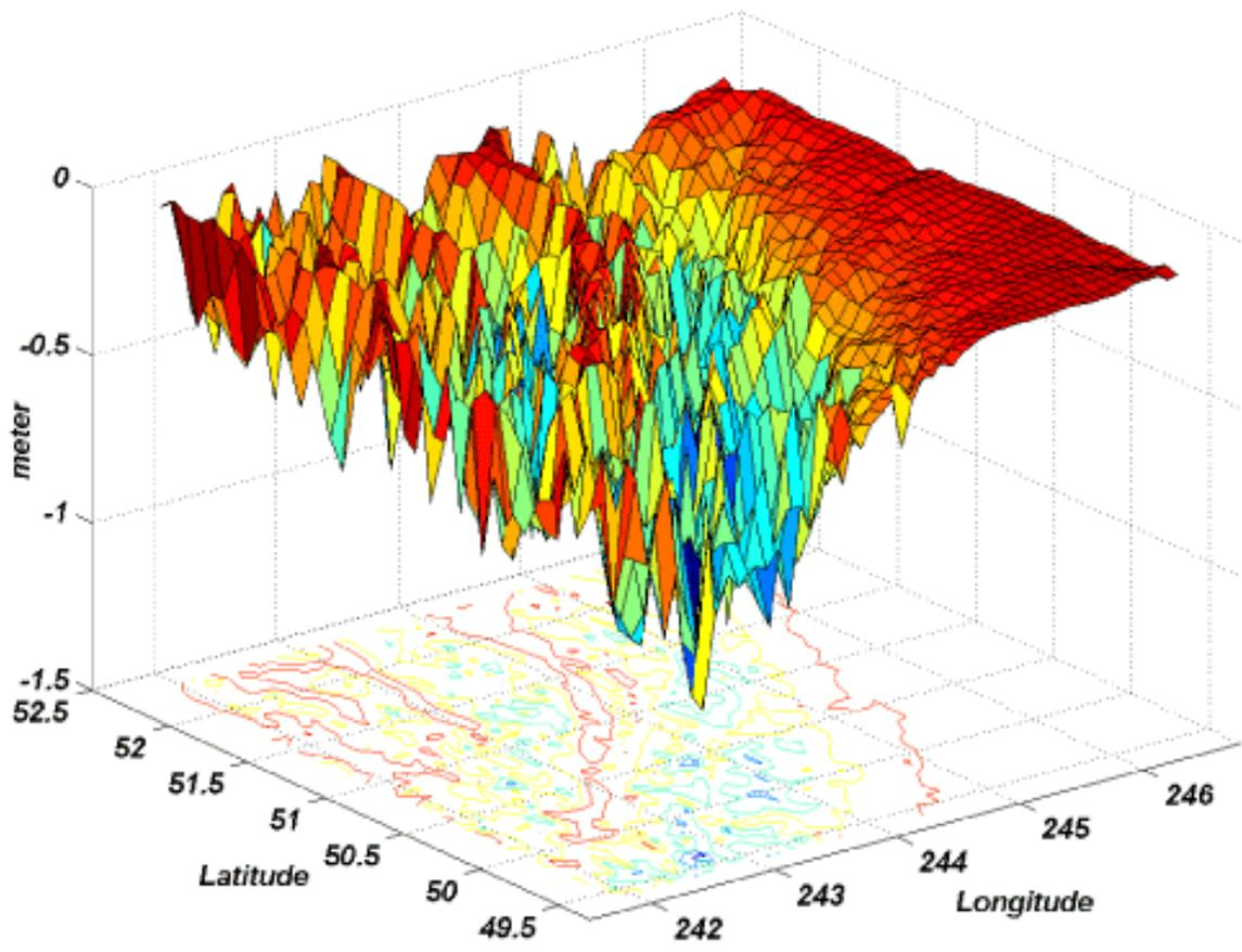
Figure 3-6: GIE computed using the 15 arcsec DTM on 5' x 5' grid (m)
