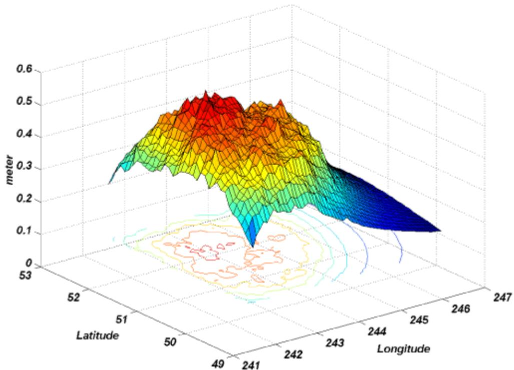
Figure 4-4: Difference in the geoid contributions of the DTE using 15 and 60 arcsec DTMs (m)
