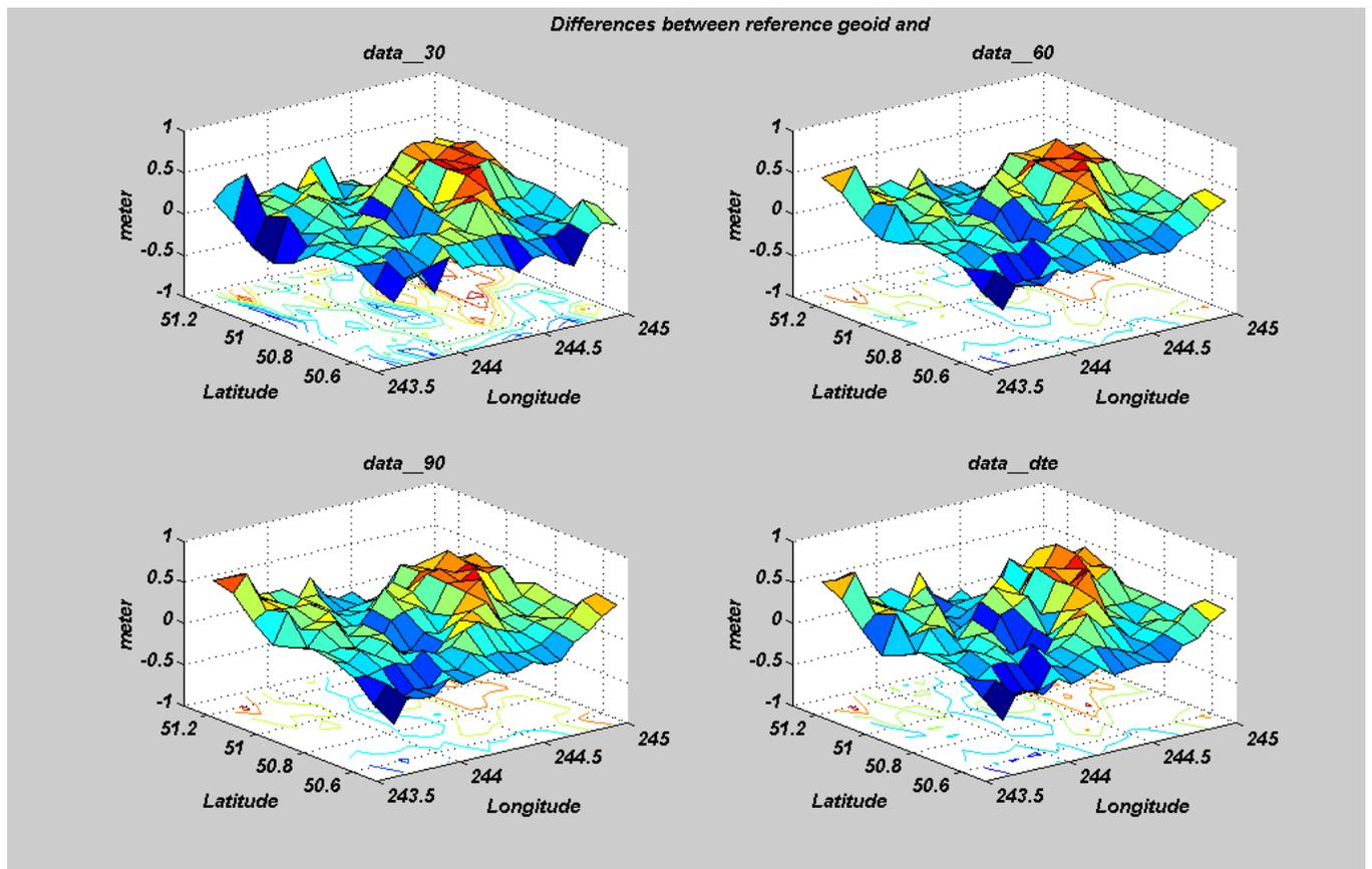
Figure 4-10: Differences between the reference geoid and geoids computed from the 1<sup>st</sup> methodology (m)
