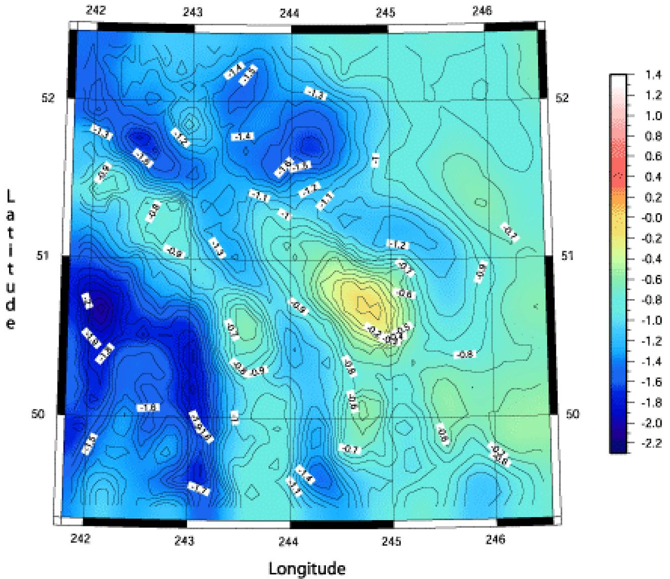
Figure 4-6: Residual geoid computed from the 2<sup>nd</sup> methodology (m)
