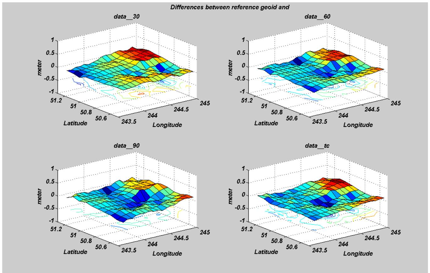
Figure 4-12: Differences between the reference geoid and geoids computed from the 2<sup>nd</sup> methodology (m)
