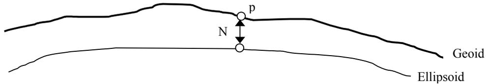
**Figure 2-1: Geoid and ellipsoid**
