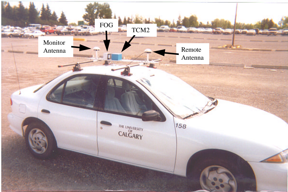
Figure 6.4 - Sensor array rigidly mounted on a test vehicle.
